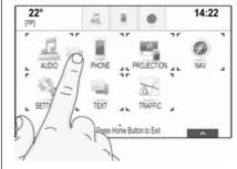
Touch and hold the element you wish to move until frame marks appear around the icons. Move your finger to the desired location and release the element.
