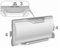
1. Press release button (3) to disengage locking shifters (4).
