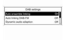
Press the **CONFIG** button. Select **Radio settings** and then **DAB settings**. The following options are available in the configuration menu:
