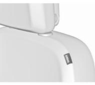
The side airbag system consists of an airbag in each front seat backrest. This can be identified by the word **AIRBAG**.
