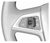
With speed limiter active, hold thumb wheel turned to **RES/+** or briefly turn to **RES/+** repeatedly until the desired maximum speed is displayed in the Driver Information Centre.
