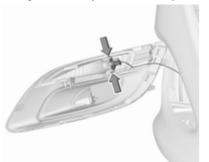
3. Disengage the bulb socket from the reflector by pressing both retaining lugs.
