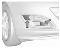
1. Release both caps with a screwdriver at the marked area.
