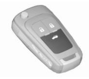
To unlock the boot lid, press  $\iff$  on the remote control for at least two seconds, or, to open from the inside, press  $\iff$  in the centre console; the boot lid is opened slightly.
