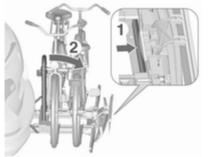
Push the lever (1) to disengage and hold.
