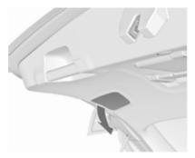
Remove the bulb holder by turning anticlockwise and replace the bulb by withdrawing or pushing the bulb slightly into the socket and rotating anticlockwise:
