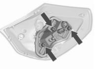
6. Unscrew the three screws with a screwdriver and remove the bulb carrier from the light assembly.
