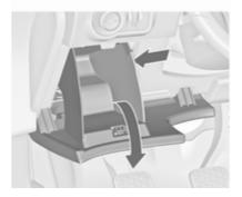
In left-hand drive vehicles, the fuse box is behind the storage compartment in the instrument panel.
