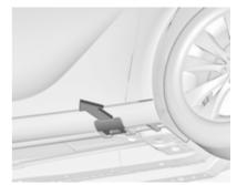
Some versions have sill panellings with covered vehicle jacking points: pull out the cover at the respective jacking point firstly.
