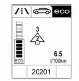
Shift indication: Current gear is indicated inside an arrow. The figure above recommends upshifting for fuel saving reasons.
