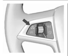
Press Jk; the current setting is shown in the Driver Information Centre. Press Jk again to change the alert sensitivity. The setting is also displayed in the top line of the Driver Information Centre.
