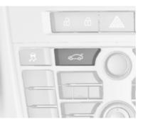
With the doors centrally locked, the boot lid cannot be opened by pressing in the centre console.
