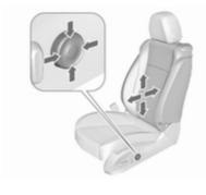
Adjust lumbar support using the four-way switch to suit personal requirements.
