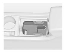
Depending on the version, cupholders are located under a cover in the centre console. Slide cover backwards. Bottles can be stowed after folding up the intermediate shelf  $\Rightarrow$  66.
