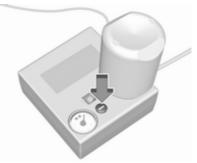
If the prescribed tyre pressure is not obtained within ten minutes, remove the tyre repair kit. Move the vehicle one tyre rotation. Reattach the tyre repair kit and continue the filling procedure for ten minutes. If the prescribed tyre pressure is still not obtained, the tyre is too badly damaged. Seek the assistance of a workshop. Drain excess tyre pressure with the button over the pressure indicator.
