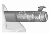
Push lever. Washer fluid is sprayed onto the rear window and the wiper wipes a few times.
