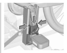
Insert pedal crank mount into outer rail of each pedal crank recess from above and slide downwards until at least underneath the notching.
