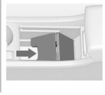
A further storage compartment is located under the intermediate shelf. Fold up the intermediate shelf and fix it in the vertical position. The frame of the cupholder can be reintegrated to stow bottles.
