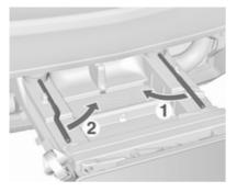
Swivel the right clamping lever (1) first, followed by the left clamping lever (2), until a resistance is noticeable.
