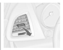
Direct the flow of air by tilting and swivelling the slats.
