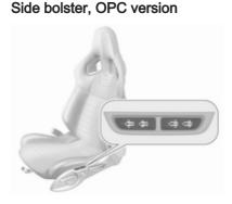
Adjust seat width and backrest width using the switches to suit personal requirements.
