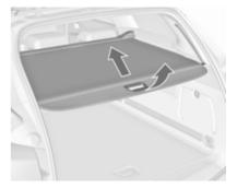
Push the handle at the end of the cover downwards. The rear of the cover is guided upwards automatically.
