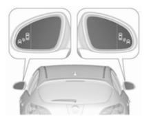
Side blind spot alert is active from speeds of 10 km/h up to 140 km/h. Driving faster than 140 km/h deactivates the system, indicated by low lighting warning symbols  $_{\mu^{ef}}$  in both exterior mirrors. Reducing the speed again will extinguish the warning symbols. If a vehicle is then detected in the blind zone, the warning symbols  $_{\mu^{ef}}$  will illuminate as normal on the relevant side.
