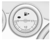
Displays the fuel level or gas level in the tank depending on the operation mode.
