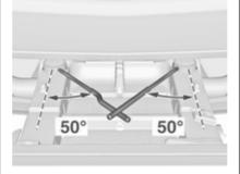
The rear carrier system is locked when the clamping levers are swivelled by approx. 50°. Otherwise safe functionality is not guaranteed.
