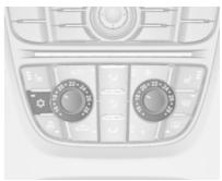
Press 🌣 to switch on cooling. Activation is indicated by illumination of the LED in the button. Cooling is only functional when the engine is running and climate control fan is switched on.
