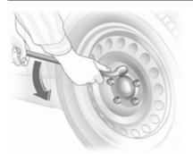
Install the wheel wrench ensuring that it locates securely and loosen each wheel nut by half a turn.
