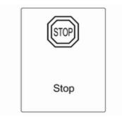
The parking slot suggestion of the system is accepted when the vehicle is stopped by the driver within ten metres after the "Stop" message is given. The system calculates the optimal route into the parking slot. Then it manoeuvres the driver into the slot by giving detailed instructions.
