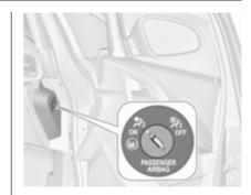
The front passenger airbag system can be deactivated via a keyoperated switch on the right side of the instrument panel. Use the ignition key to choose the position:
