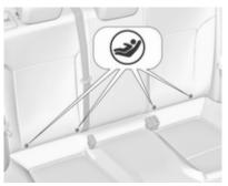
Fasten vehicle-approved ISOFIX child restraint systems to the ISOFIX mounting brackets. Specific vehicle ISOFIX child restraint system positions are marked in the table by IL.
