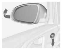
Turn control to **0**, then push the control down. Both exterior mirrors will fold.
