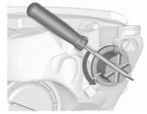
1. Rotate the cap (3) anticlockwise and remove it. Use the screwdriver to rotate the cap.
