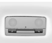
Illuminates in conjunction with the front courtesy light depending on rocker switch position.
