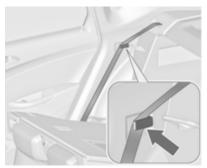
If the vehicle is to be loaded via a rear door, take the seat belt out of the seat backrest guide and put it behind the retainer (as shown in the illustration).
