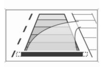
Trajectory lane of the vehicle is shown in accordance with the steering angle.
