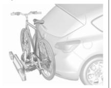
The rear carrier system (Flex-Fix system) allows bicycles to be attached to a pull-out carrier integrated into the vehicle floor. The transportation of other objects is not permitted.
