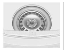
The spare wheel is located in the load compartment beneath the floor covering. It is secured with a wing nut.
