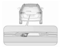
The camera is mounted in the tailgate handle and has a viewing angle of 130°.
