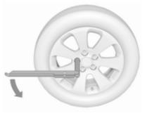
Fold out the wheel wrench and install ensuring that it locates securely and loosen each wheel nut by half a turn.
