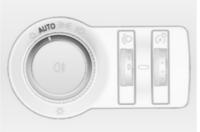
When the automatic light control function is switched on and the engine is running, the system switches between daytime running light and headlights automatically depending on the lighting conditions and information given by the rain sensor system.
