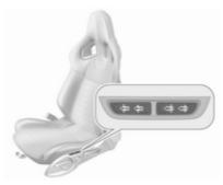
Adjust seat width and backrest width using the switches to suit personal requirements.
