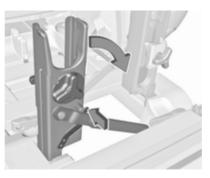
Disengage the locking lever on the diagonal support and fold both pedal crank recesses down.
