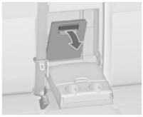
• Pull the grip and open the cover. Suitable for loading long, narrow objects.
