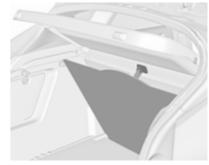
The rear floor cover can be lifted. Hinge the loop into the hook on the lower side of the load compartment cover.
