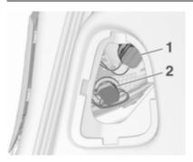
2. Remove the bulb holder by turning and replace the bulb by withdrawing or pushing the bulb slightly into the socket and rotating anticlockwise:
