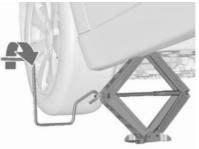
Attach jack handle and with the jack correctly aligned rotate
