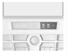
If the control indicator  $\Re_2$  illuminates for approx. 60 seconds after the ignition is switched on, the front passenger airbag system will inflate in the event of a collision.
