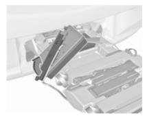
Open out the lamp support on the back of the tail lamp completely.
