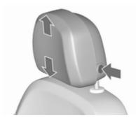
Press release button, adjust height, engage.
