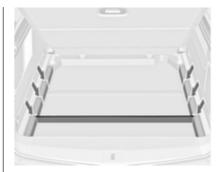
Insert the bar into the recesses at the sidewalls.
