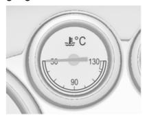
Displays the coolant temperature.
