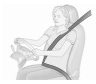
The seat belts are locked during hard acceleration or deceleration of the vehicle holding the occupants in the sitting position. Therefore the risk of injury is considerably reduced.
