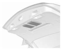
Fold down strap. Stow the first aid kit in the space behind a strap on the inside of the tailgate.
