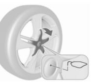
Alloy wheels with centre wheel bolt cap: Disengage centre cap by inserting and pulling the extractor in the recess of the brand emblem, vehicle tools  $\Rightarrow$  264.
