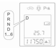
The mode or selected gear is shown in the transmission display.
