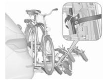
4. Guide the strap attached to the adapter underneath the lever for folding back the rear carrier system. Fasten the strap.
