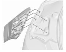
3. Carefully withdraw the light assembly from the recesses and remove.
