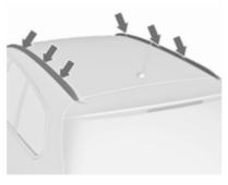
Fasten the roof rack in the area of the holes, indicated by the arrows in the illustration.
