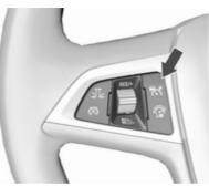
Press ℜ to switch on adaptive cruise control. The control indicator ℕ illuminates white.
