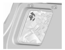
2. Unscrew the plastic securing nut from the inside by hand.
