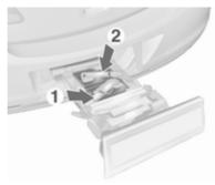
First remove the rear (1), then the front (2) tail lamp from the recesses.
