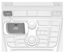
Pressing LPG switches between petrol and liquid gas operation as soon as the required parameters (coolant temperature, gas temperature and minimum engine speed) have been reached. The requirements are usually fulfilled after around 60 seconds (depending on exterior temperature) and the first firm press on the accelerator. The LED status shows the current operating mode.
