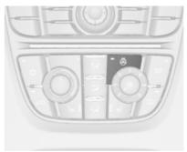
Activate heating by pressing . Activation is indicated by illumination of the LED in the button.
