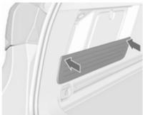
When assembling press the blind on the left-hand side into the rubber grommets to reach full retention force.
