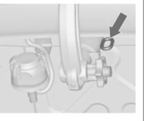
Attach breakaway stopping cable to eye.
