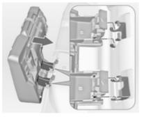
• To attach, apply seat cushion as shown in the illustration and engage both levers.
