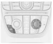
Press Solution to activate air recirculation mode. Activation is indicated by the LED in the button.
