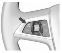
Press  $\mathfrak{F}_{\mathfrak{C}}$ ; the current setting is shown in the Driver Information Centre. Press  $\mathfrak{F}_{\mathfrak{C}}$  again to change the following distance. The setting is also displayed in the top line of the Driver Information Centre.
