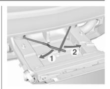
Swivel first the left clamping lever (1), followed by the right clamping lever (2), until they stop.
