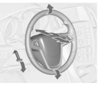
Unlock the lever, adjust the steering wheel, then engage the lever and ensure it is fully locked.
