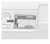
Press button to remove the frame of the cupholder. The frame can be stowed in the glovebox.
