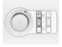
To adapt headlight range to the vehicle load to prevent dazzling: turn thumb wheel D to required position.
