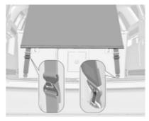
Attach lower hook with opening facing backward to eye in the right and left of the floor. Adjust strap length on safety net by attaching the upper hook to the eyes of the strap. Keep strap under tension while proceeding with installation of rod.
