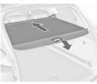
Pull the handle at the end of the cover to the rear and downwards. It rolls up automatically.
