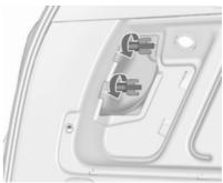
3. Unscrew two plastic securing nuts from the inside by hand.
