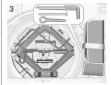
The jack and the tools are in the tool box below the spare wheel in the load compartment. The wheel wrench, the towing eye and an extension bolt for securing a damaged wheel (only vehicles with temporary spare wheel) are in the tool bag located in the spare wheel well near the tool box. Spare wheel  $\Rightarrow$  279.
