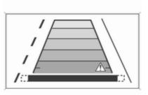
Due to the high position of the camera the rear bumper can be seen on the display as a guide to position.
