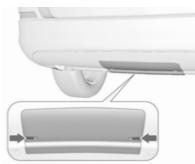
All versions except 3-door hatchback: Press fastenings inward and fold the cover downward at the front. Remove cover.
