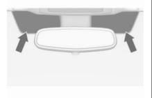
The marked areas on the windscreen are not covered with the coating. Devices for electronic data recording and fee payment must be attached in these areas. Otherwise data recording malfunctions may occur.
