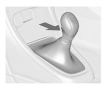
To engage reverse, with the vehicle stationary, depress clutch pedal, press the release button on the selector lever and engage the gear.
