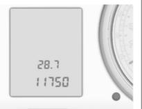
The bottom line displays the recorded distance in km.
