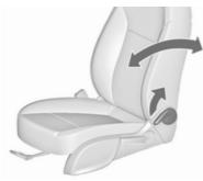
Pull lever, adjust inclination and release lever. Allow the seat to engage audibly.
