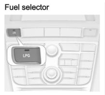
Press **LPG** to switch between petrol and liquid gas operation. The LED — status shows the current operating mode.
