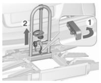
Arrange mounting brackets as shown in the illustration.
