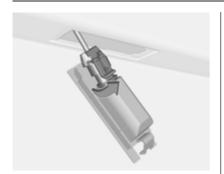
2. Remove lamp downwards, taking care not to pull on the cable.
