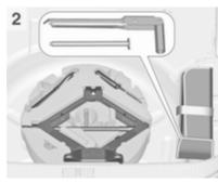
The jack, the tools and the towing eye are in the tool box below the spare wheel in the load compartment. The wheel wrench and an extension bolt for securing a damaged wheel (only vehicles with temporary spare wheel) are in the tool bag located in the spare wheel well near the tool box. Spare wheel  $\diamondsuit$  279.
