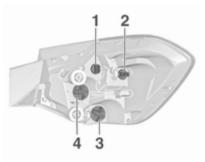
Remove the bulb holder by turning anticlockwise and replace the bulb by withdrawing or pushing the bulb slightly into the socket and rotating anticlockwise:
