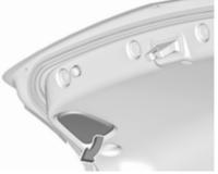
1. Open the tailgate and remove the cover on the respective side.
