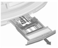
Completely pull out the rear carrier system until you hear it engage.
