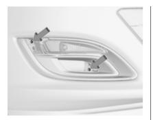
2. Unscrew both screws and remove light assembly from the bumper.
