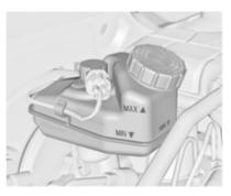
The brake fluid level must be between the **MIN** and **MAX** marks.
