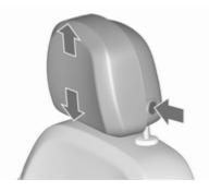
Height adjustment Press release button, adjust height, engage.
