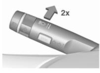
The high beam assist is activated by pushing the indicator lever twice with a speed above 40 km/h.
