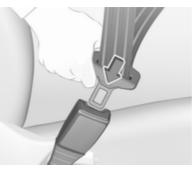
Loose or bulky clothing prevents the belt from fitting snugly. Do not place objects such as handbags or mobile phones between the belt and your body.
