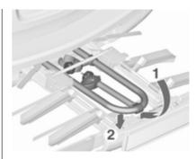
Fold the rack backwards, then push forwards until it stops (1). Press the rack down at the rear (2).
