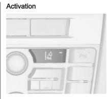
The lane departure warning system is activated by pressing lá. The illuminated LED in the button indicates that the system is switched on. When control indicator lá in the instrument cluster illuminates green, the system is ready to operate.
