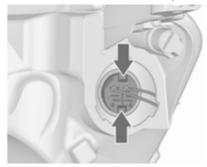
2. Press latches together and withdraw the bulb holder from the reflector.
