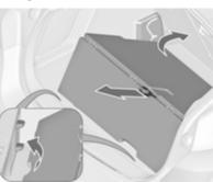
To lift the cover to a higher level, pull the loop backwards and lift the rear edge of the cover onto the corresponding supports.
