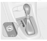
Without brake pedal applied, the control indicator (S) illuminates.
