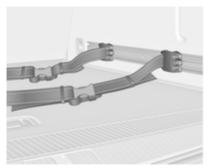
Insert the adapters of the strap set in a rail. Make sure that the belt is not twisted.
