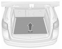
Lift the rear floor cover by pulling the handle. Fold and place the cover behind the rear seats.
