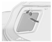
1. Release the cover on the respective side and remove it.
