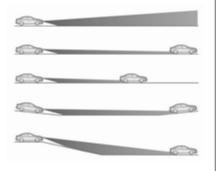
A special topographical evaluation function detects preceding vehicles on hills or slopes by recognising the rear light moving ahead. The system adjusts the height of the light range to ensure optimum illumination on the road ahead without dazzling.
