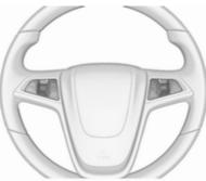
The Infotainment system, the cruise control and a connected mobile phone can be operated via the controls on the steering wheel.
