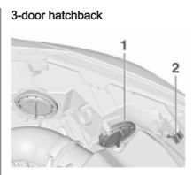
**Bi-Halogen Headlight (1)** with one bulb for low and high beam. **Sidelight/Daytime running light (2)**.
