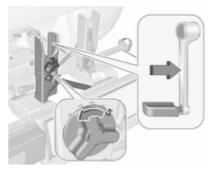
With the rotary lever on the pedal crank recess, roughly adapt the adjustable pedal crank unit to the protrusion of the pedal crank.
