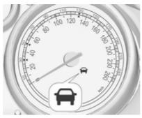
The green illuminated vehicle ahead control indicator  $rac{l}$  is displayed in the speedometer when the system detects a vehicle in the driving path.
