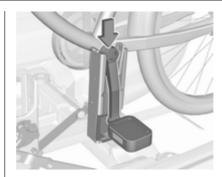
Put on the bicycle. The pedal crank here must be placed in the pedal crank recess opening, as shown in the illustration.
