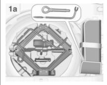
The jack, the tools and a strap for securing a damaged wheel are in the tool box below the spare wheel in the load compartment. The wheel wrench and the towing eye are in the tool bag located in the spare wheel well near the tool box. Spare wheel  $\diamondsuit$  279.
