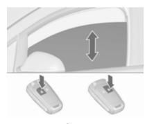
Press and hold a to open windows. Press and hold a to close windows. Release button to stop window movement.
