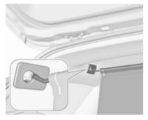
There are two installation openings in the roof frame: suspend and engage rod of net at one side, compress rod and suspend and engage at other side.
