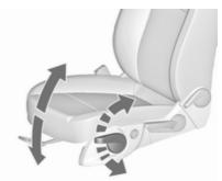
Lever pumping motion up : front end higher down : front end lower
