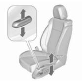
Move switch upwards/downwards.
