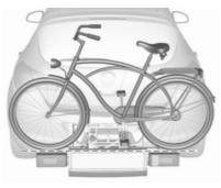
Place the wheel recesses such that the bicycle is more or less horizontal. Here, the distance between the pedals and the tailgate should be at least 5 cm.
