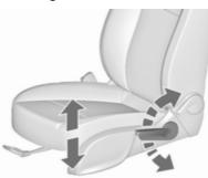
Lever pumping motion up : seat higher down : seat lower
