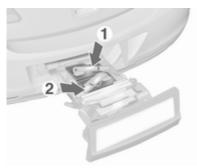
Fold in the lamp supports on the backs of the tail lamps.
