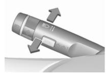
To switch from low to high beam, push lever.
