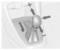
Move selector lever out of position D towards the left to select manual mode M.
