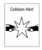
When the distance to a preceding moving vehicle gets too small or when approaching another vehicle too rapidly and a collision is imminent, the collision alert symbol pops-up in the Driver Information Centre.
