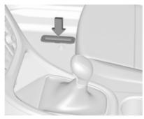
The Vehicle Identification Number may be stamped on the identification plate and on the floor pan, under the floor covering, visible under a cover. The Vehicle Identification Number may be embossed on the instrument panel, visible through the windscreen, or in the engine compartment on the right body panel.
