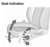
Lever pumping motion up : front end higher down : front end lower
