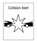
If a vehicle directly ahead is approached too quickly, a warning chime and alert in the Driver Information Centre is provided.
