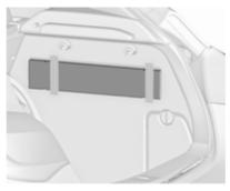
Stow the warning triangle in the space behind the strap on the right side of the load compartment.
