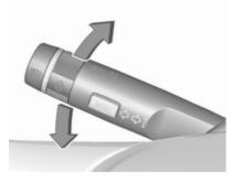
lever up : right turn signal lever down : left turn signal
