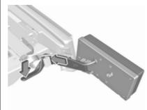
Push the clamping lever down and push the lamp support into the retainer until it engages.
