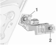
5. Remove and replace the bulb by withdrawing or pushing the bulb
