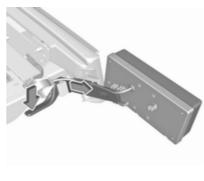
Push the clamping lever down and pull both lamp supports out of the recesses.
