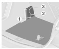
The height adjustable cover can be mounted in three positions:
