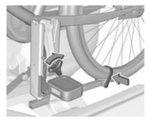
Tighten the attachment screw for the pedal bearing mount to its maximum point by hand.
