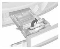
Fold one or both pedal crank recesses upwards until the diagonal support engages.
