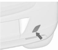
Insert a screwdriver in the slot at the lower bend of the cap. Release the cap by carefully moving the screwdriver downwards.
