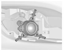
3. Unscrew three screws and remove fog light assembly from the bumper.
