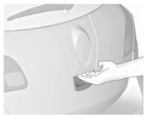
After unlocking, push the touchpad switch below the brand emblem and open the tailgate.
