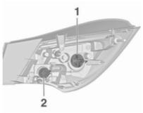
Remove the bulb holder by turning and replace the bulb by withdrawing or pushing the bulb slightly into the socket and rotating anticlockwise:
