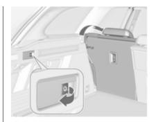
Pull switch on left or right sidewall of the load compartment to fold the corresponding part of the rear seat.
