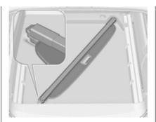
The removed cover can be stored under the rear floor cover like shown in the graphic.
