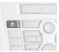
For very high-performance driving ESC and TC can be deactivated separately. The following modes are selectable:
