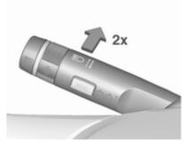
Intelligent light ranging and automatic high beam activation are switched on together by pushing the indicator lever twice. They can be switched on with ignition on. Automatic high beam activation operates at a speed above 40 km/h and deactivates below 20 km/h. Intelligent light ranging operates above 55 km/h.
