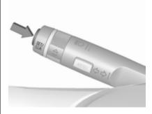
The alert function can be activated or deactivated in the Settings menu of the traffic sign assistant page by pressing **SET/CLR** on the turn signal lever.
