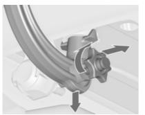
Open the protective flap and turn the key to position a to unlock the coupling ball bar.
