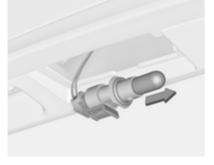
Remove bulb holder from lamp housing by turning anticlockwise.
