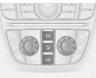
Press appropriate button for desired adjustment. Activation is indicated by illumination of the LED in the button.
