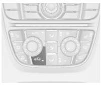
Press Solution to activate the air recirculation mode. Activation is indicated by illumination of the LED in the button.
