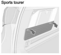
1. On left-hand side, fold down the blind and remove.
