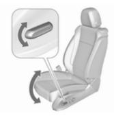
Move front of switch upwards/ downwards.
