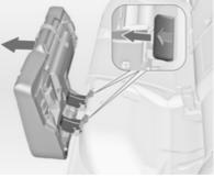
• Push both levers forward and remove seat cushion to extend the loading area.
