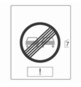
An exclamation mark in a frame indicates that there is an add-on sign detected which cannot be recognised by the system.
