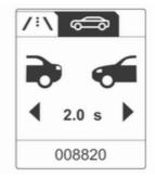
• Following Dist.: Displays the distance to a moving vehicle ahead ♀ 200.
