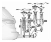
The rear carrier system (Flex-Fix system) allows two bicycles to be attached to a pull-out carrier integrated into the vehicle floor. It is possible to attach two further bicycles on an adapter. The transportation of other objects is not permitted.
