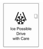
If outside temperature drops to 3 °C, a warning message is displayed in the Driver Information Centre with Uplevel-Combi-Display.
