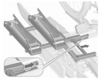
1. Apply the adapter to the rear carrier system as shown in the illustration.
