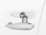
2. Turn bulb holder anticlockwise and remove from housing.
