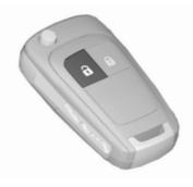
Press d to unlock the doors and load compartment. Open the doors by pulling the handles.
