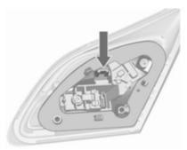
4. Press the retaining lug and remove the bulb carrier from the light assembly.
