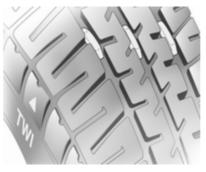
The legally permissible minimum tread depth (1.6 mm) has been reached when the tread has worn down as far as one of the tread wear indicators (TWI). Their position is indicated by markings on the sidewall. If there is more wear at the front than the rear, swap round front wheels and rear wheels periodically. Ensure that the direction of rotation of the wheels is the same as before.
