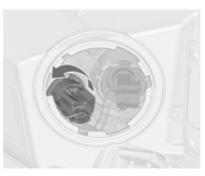
2. Rotate bulb socket anticlockwise to disengage and withdraw from the reflector.
