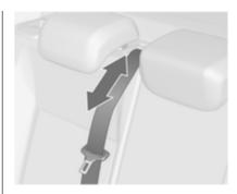
The seat belt of the centre seat could be blocked when the backrest is folded up too quickly. To unlock the retractor, push in the seat belt or pull it out by approx. 20 mm then release. Raise the seat cushion and fold the backrest
