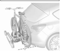
Align the bicycle in the longitudinal direction of the vehicle: Slightly loosen the pedal mount.
