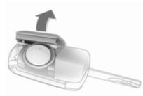
Extend the key and open the unit. Replace the battery (battery type CR 2032), paying attention to the installation position. Close the unit and synchronise.
