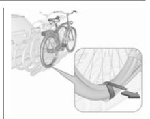
Additionally, secure both bicycle wheels of the fourth bicycle to the wheel recesses using the tensioning straps.
