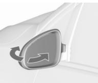
For pedestrian safety, the exterior mirrors will swing out of their normal mounting position if they are struck with sufficient force. Reposition the mirror by applying slight pressure to the mirror housing.
