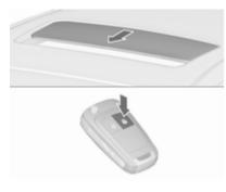
Press and hold <sup>®</sup> to close the sunroof. Release the button to stop the movement.
