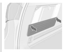
When assembling press the blind into the rubber grommets to reach full retention force.
