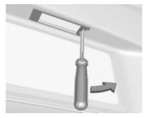
1. Insert screwdriver in recess of the cover, press to the side and release spring.
