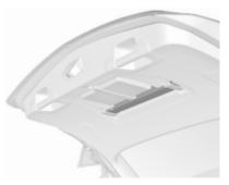
Fold down straps. Stow the warning triangle in the space behind the straps on the inside of the tailgate.
