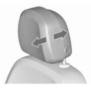
To adjust horizontally, pull the head restraint forwards. It engages in several positions.
