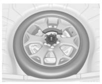
A damaged full size wheel must be stowed outside up in the spare wheel well secured with the wing nut.
