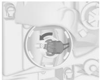
Rotate the bulb holder anticlockwise to disengage. Withdraw the bulb holder from the reflector.
