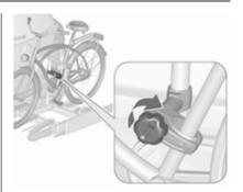
2. Attach the short mounting bracket to the bicycle frame. Turn the knob clockwise to fasten.
