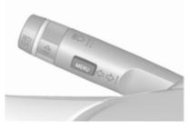
Press **MENU** to switch between the menus or to return from a submenu to the next higher menu level.
