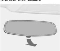
To reduce dazzle, adjust the lever on the underside of the mirror housing.
