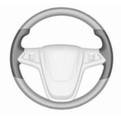
The recommended grip areas of the steering wheel are heated quicker and to a higher temperature than the other areas.
