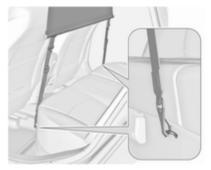
Attach strap to eyes underneath the rear seat cushion.
