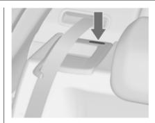
The backrests are properly engaged when the red marks on both sides near the release lever are no longer visible.
