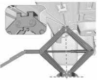
Set the jack to the necessary height. Position it directly below the jacking point in a manner that prevents it from slipping.
