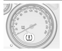
A detected low tyre pressure condition is indicated by control indicator  $\Leftrightarrow$  120.
