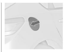
The fuel filler flap can only be opened if the vehicle is unlocked. Release the fuel filler flap by pushing the flap.
