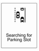
When the vehicle passes a row of cars and the system is activated, the advanced parking assist system begins searching for a suitable parking slot. When a suitable slot is detected, visual feedback in the Driver Information Centre and an acoustic signal are given. If the driver does not stop the vehicle within ten metres after a parking slot is proposed, the system starts to search for another suitable parking slot.
