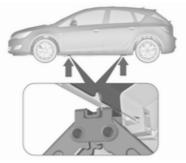
3. Ensure the jack is correctly positioned under the relevant vehicle jacking point.
