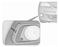
1. Disengage the cover with a screwdriver in the recess and remove the cover.
