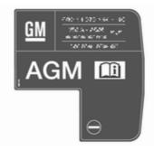
An AGM battery can be identified by the label on the battery. We recommend the use of an original Opel vehicle battery.
