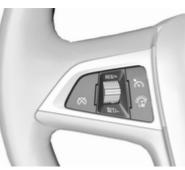
Press @. If cruise control or adaptive cruise control has been activated before, it is switched off when speed limiter is activated and control indicator (3) extinguishes.
