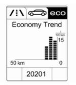
• Economy Trend: Displays the average consumption development over a distance of 50 km. Filled segments display the consumption in 5 km steps and shows the effect of topography or driving behaviour on fuel consumption.
