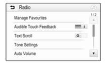
If you wish the text to be scrolled continually, activate **Text Scroll**. If you wish the text to be scrolled in blocks, deactivate the setting.
