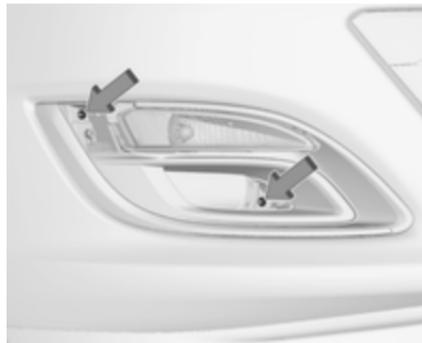
2. Unscrew both screws and remove light assembly from the bumper.
