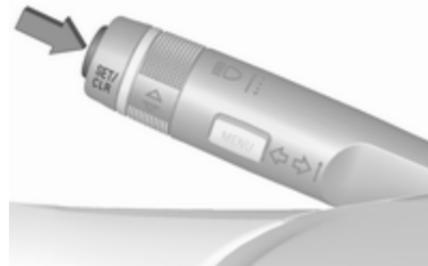
The alert function can be activated or deactivated in the Settings menu of the traffic sign assistant page by pressing **SET/CLR** on the turn signal lever.
