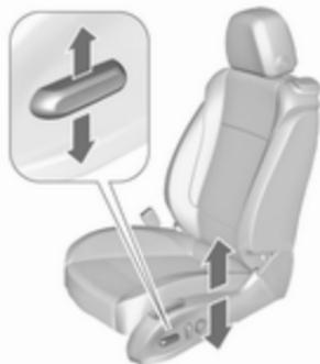
Move switch upwards/downwards.
