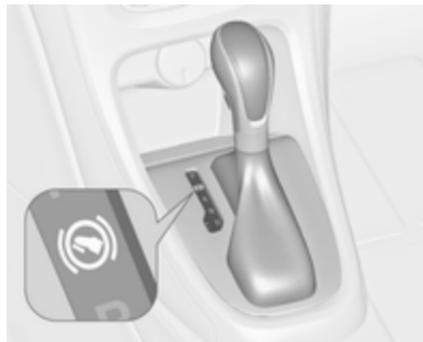
Without brake pedal applied, the control indicator (Ⓢ) illuminates.
