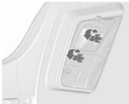
2. Unscrew both plastic securing nuts from the inside by hand.
