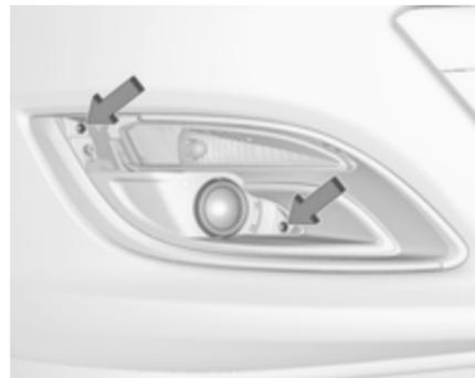
2. Unscrew both screws and remove turn light assembly from the bumper.
