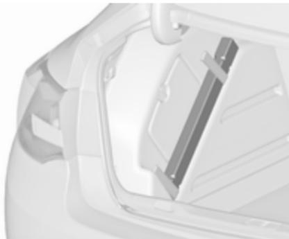
Stow the warning triangle in the recess on the left side of the load compartment.
