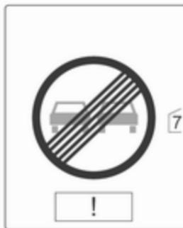
An exclamation mark in a frame indicates that there is an add-on sign detected which cannot be recognised by the system.
