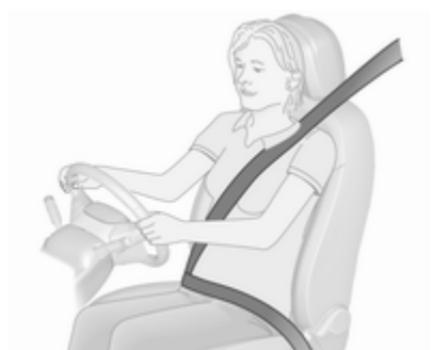
Pull out the seat belt and fasten in belt buckle. The seat belt must not be twisted and must fit close against the body. The backrest must not be tilted back too far (maximum approx. 25 °). To unfasten belt, press red button on belt buckle.
