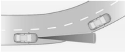
The adaptive cruise control calculates a predicted path based on the centrifugal force. This predicted path considers the current bend characteristic, but cannot consider a future bend change. The system may lose the current vehicle ahead or consider a vehicle which is not in the actual lane. This can happen when
