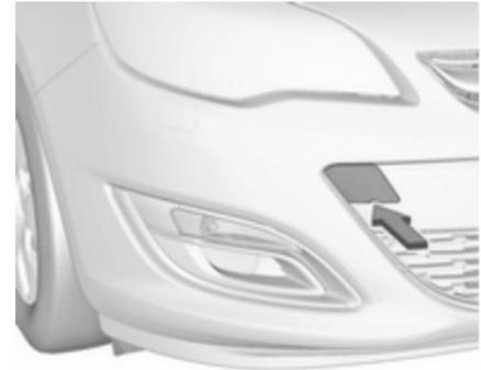
Insert a screwdriver in the slot at the lower part of the cap. Release the cap by carefully moving the screwdriver downwards.
