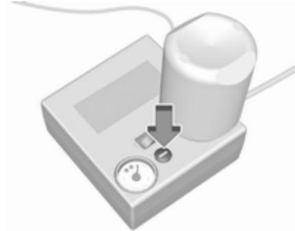
If the prescribed tyre pressure is not obtained within ten minutes, remove the tyre repair kit. Move the vehicle one tyre rotation. Reattach the tyre repair kit and continue the filling procedure for ten minutes. If the prescribed tyre pressure is still not obtained, the tyre is too badly damaged. Seek the assistance of a workshop. Drain excess tyre pressure with the button over the pressure indicator. Do not run the compressor longer than ten minutes.
