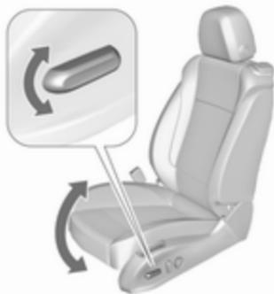
Move front of switch upwards/
