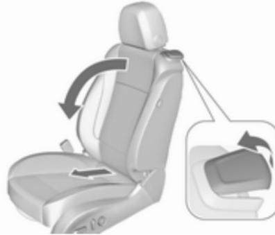
Lift release lever and fold backrest forwards. The seat slides automatically forwards to the stop.
