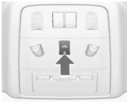
Switch off the monitoring of passenger compartment and vehicle inclination when animals are being left in the vehicle, because of high volume ultrasonic signals or movements triggering the alarm. Also switch off when the vehicle is on a ferry or train.
