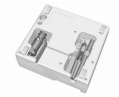
3. Remove the electrical connection cable and air hose from the stowage compartments on the underside of the compressor.
