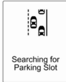
When the vehicle passes a row of cars and the system is activated, the advanced parking assist system begins searching for a suitable parking slot. When a suitable slot is detected, visual feedback in the Driver Information Centre and an acoustic signal are given.
