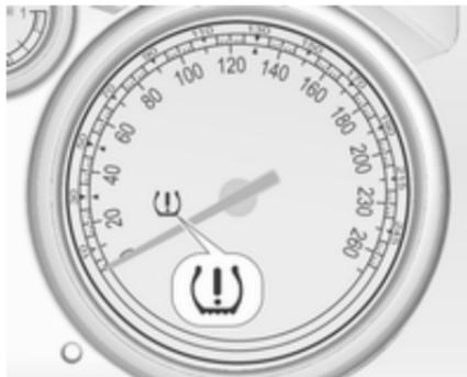
A detected low tyre pressure condition is indicated by illumination of control indicator (⚠) ⇨ 91.
