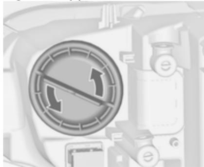
1. Rotate the cap (2) anticlockwise and remove it.
