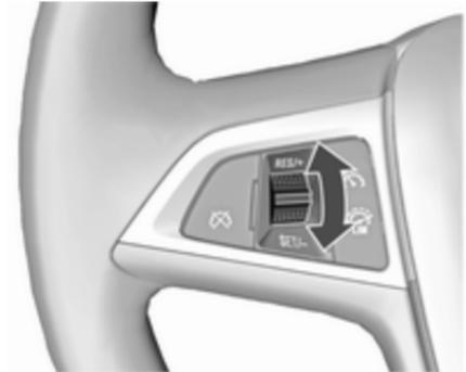
With speed limiter active, hold thumb wheel turned to **RES/+** or briefly turn to **RES/+** repeatedly until the desired maximum speed is displayed in the Driver Information Centre.
