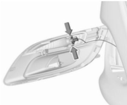
3. Disengage the bulb socket from the reflector housing by pressing both retaining lugs.
