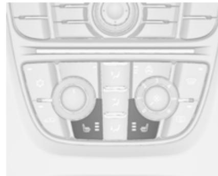
Adjust heating to the desired setting by pressing
