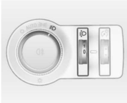
To adapt headlight range to the vehicle load to prevent dazzling: turn thumb wheel
