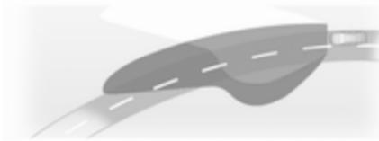
The light beam pivots based on steering wheel angle and speed, improving lighting in curves.
