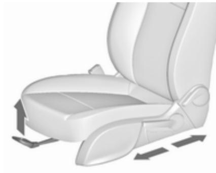
Pull handle, slide seat, release handle. Try to move the seat back and forth to ensure that the seat is locked in place.
