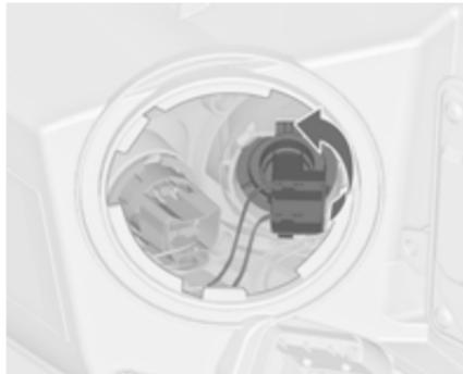
2. Rotate the bulb holder anticlockwise to disengage. Withdraw the bulb holder from the reflector.
