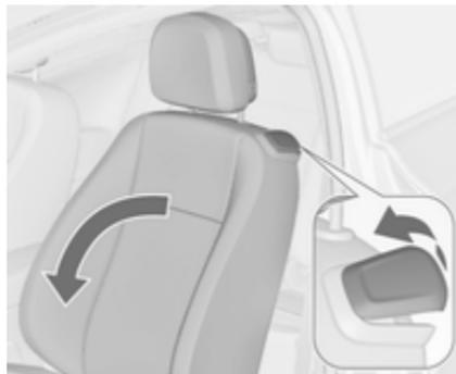
Lift release lever and fold backrest forwards, then slide seat forwards to the stop.
