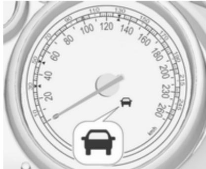
The green illuminated vehicle ahead control indicator
