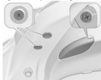
1. Open the tailgate and remove the covers on the respective side.
