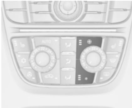
Press lower button to decrease or upper button to increase fan speed. The fan speed is indicated by the number of segments in the display.
