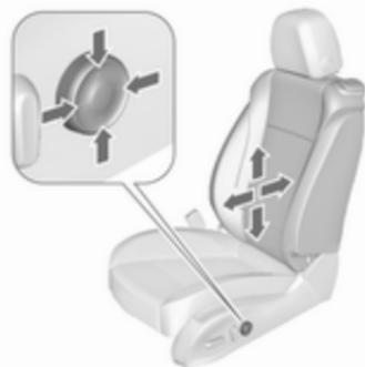
Adjust lumbar support using the four-way switch to suit personal requirements.
