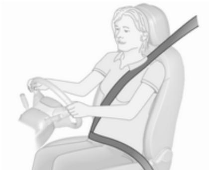
The seat belts are locked during hard acceleration or deceleration of the vehicle, holding the occupants in the seat position. Therefore the risk of injury is considerably reduced.
