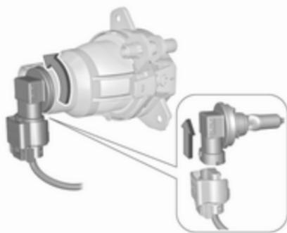
4. Turn the bulb socket anticlockwise and remove it from the reflector housing.
