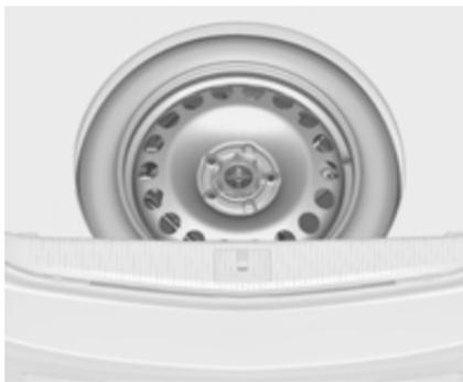
The spare wheel is located in the load compartment beneath the floor covering. It is secured with a wing nut.
