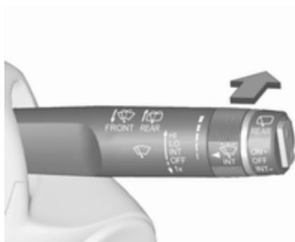
Push lever. Washer fluid is sprayed onto the rear window and the wiper wipes a few times.
