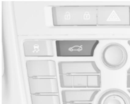
With the doors centrally locked, the boot lid cannot be opened by pressing
