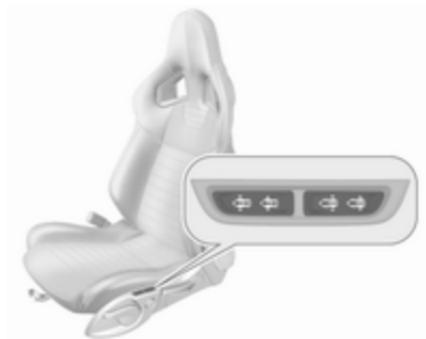
Adjust seat width and backrest width using the switches to suit personal requirements.
