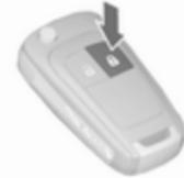
Press and hold
