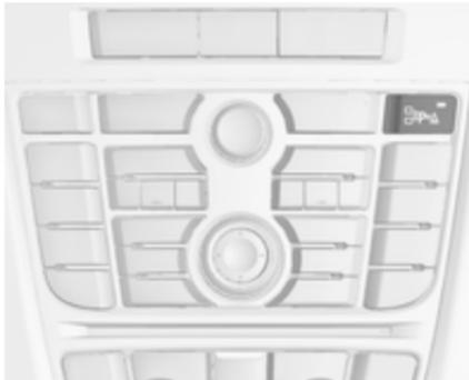
When searching for a parking slot, the system must be activated by pressing
