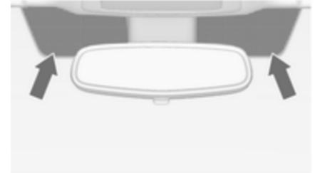
The marked areas on the windscreen are not covered with the coating. Devices for electronic data recording and fee payment must be attached in these areas. Otherwise data recording malfunctions may occur.
