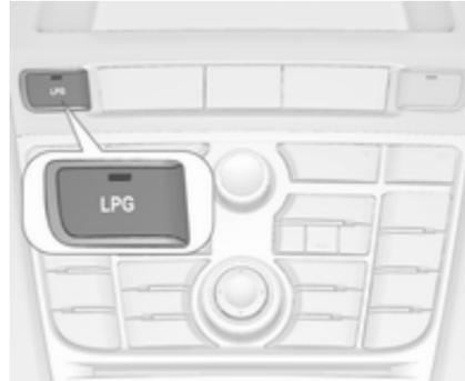
Pressing **LPG** switches between petrol and liquid gas operation as soon as the required parameters (coolant temperature, gas temperature and minimum engine speed) have been reached. The requirements are usually fulfilled after around 60 seconds (depending on exterior temperature) and the first firm press on the accelerator. The LED status shows the current operating mode.
