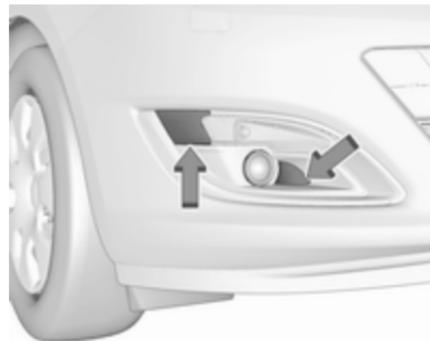
1. Release both caps with a screwdriver at the marked area.
