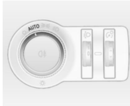
When the automatic light control function is switched on and the engine is running, the system switches between daytime running light and headlights automatically
