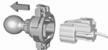
4. Disengage the plug connector from the bulb socket by pressing the retaining lug.
