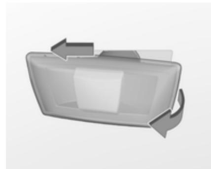
1. Slide lamp to its left side and remove at its right end.
