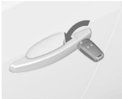
Manually unlock the driver's door by turning the key in the lock. Switch on the ignition and press the central locking button
