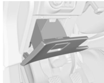
A storage compartment is located next to the steering wheel.
