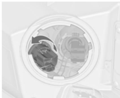
2. Rotate bulb socket anticlockwise to disengage and withdraw from the reflector housing.
