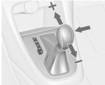
Move selector lever out of position **D** towards the left to select manual mode **M**.
