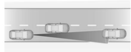
If another vehicle enters your driving path, adaptive cruise control will first consider the vehicle when it is completely in your path. Be ready to take action and depress the brake pedal, if you need to brake more quickly.
