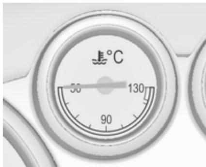
Displays the coolant temperature.
