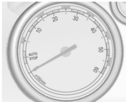
Displays the engine speed.
