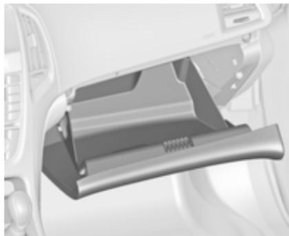
The glovebox features a pen holder, a credit card holder, a coin holder and an adapter for the locking wheel nuts.
