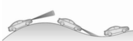
System performance on hills and when towing a trailer depends on your vehicle speed, vehicle load, traffic conditions and the road gradient. It may not detect a vehicle in your path while driving on hills. On steep hills, you may have to use the accelerator pedal to maintain your vehicle speed. When going downhill, especially when towing a trailer, you may have to brake to maintain or reduce your speed.
