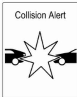
If a vehicle directly ahead is approached too quickly, a warning chime and alert in the Driver Information Centre is provided.
