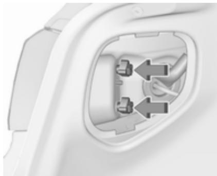
2. Unscrew two plastic securing nuts from the inside by hand.
