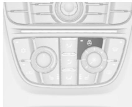
Activate heating by pressing
