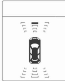
The distance to a front and rear obstacle is indicated by changing distance lines around the vehicle.
