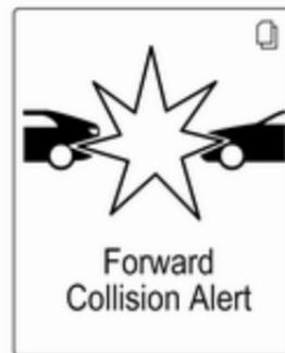
A green illuminated vehicle ahead control indicator illuminates in the instrument cluster when the system has detected a vehicle in the driving path. When the distance to a preceding moving vehicle gets too small or when approaching another vehicle too rapidly and a collision is imminent, the collision alert symbol pops-up in the Driver Information Centre. Simultaneously a warning chime sounds.
