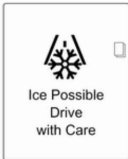
If outside temperature drops to 3 °C, a warning message is displayed in the Driver Information Centre with Uplevel-Combi-Display.
