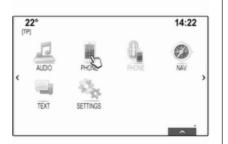
Place your finger on the pad. A hand cursor appears on the screen. Depending on the position of your finger, the system may highlight an element on the screen.
