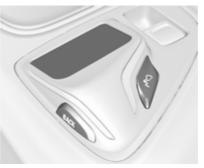
The touch pad has a touch-sensitive surface that allows additional functions for menu control on the centre display. It is located behind the gearshift lever.
