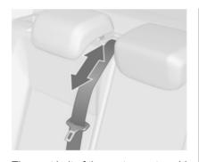
The seat belt of the centre seat could be blocked when the backrest is folded up too quickly. To unlock the retractor, push in the seat belt or pull it out by approx. 20 mm and then release.
