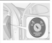
The front passenger airbag system can be deactivated via a keyoperated switch on the right side of the instrument panel. Use the ignition key to choose the position:
