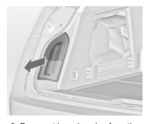
Press out lamp housing from the inside of the side trim panel.
