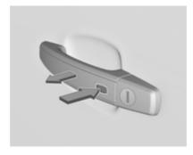
Press the button on any exterior door handle and pull the handle.
