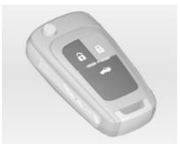
Press button 🖥 to unlock the doors and load compartment. Open the doors by pulling the handles. To open the tailgate, pull the button under the tailgate moulding.
