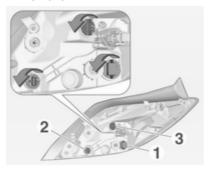
Turn bulb holder anticlockwise and remove. Replace bulb by withdrawing or turning:
