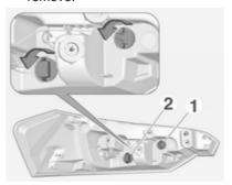
Turn bulb holder anticlockwise and remove. Replace bulb by withdrawing:
