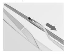
Disengage the wiper blade and remove.
