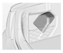
The fuse box is on the left side of the load compartment behind a cover. Remove the cover.
