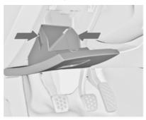
In left-hand drive vehicles, the fuse box is behind the storage compartment in the instrument panel. Open compartment, compress the locking tabs, fold compartment down and remove.
