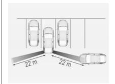
The system sensors cover a zone of approx. 20 metres to the left or right side behind the vehicle.
