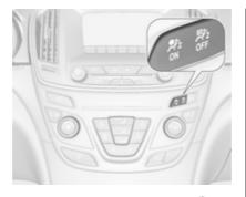
As long as the control indicator  $\frac{1}{2}$  is not illuminated, the airbag systems for the front passenger seat will inflate in the event of a collision.
