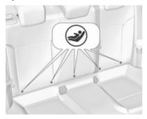
Fasten vehicle-approved ISOFIX child restraint systems to the ISOFIX mounting brackets. Specific vehicle ISOFIX child restraint system positions are marked in the table by IL ▷ 63.
