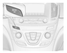
Deactivate the stop-start system manually by pressing the **eco** button. The deactivation is indicated when the LED in the button extinguishes.
