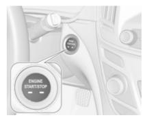
Electronic key must be inside the vehicle.
