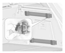
Fold open the handle plate, insert the adapter into the upper and lower groove of the rail and move to the required position. Turn the handle
