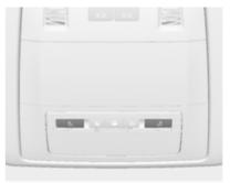
Operated with \( \sigma \) and \( \alpha \) buttons in front and rear courtesy lights.
