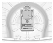
The tools and the towing eye are located together with the tyre repair kit in a tool box below the floor cover in the load compartment.
