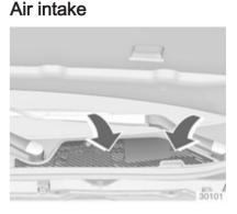
The air intake in front of the windscreen in the engine compartment must be kept clear to allow air intake. Remove any leaves, dirt or snow.
