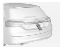
To open the tailgate, press the touchpad switch under the tailgate moulding until the tailgate starts to move.
