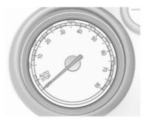
Displays the engine speed.
