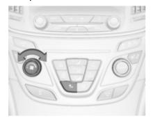
Turn controller %. The selected fan speed is indicated by the number of segments in the climate display. If the fan is switched off, the air conditioning is also deactivated.
