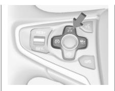
Press button J, the current setting is shown in the Driver Information Centre. Press button J, again to change the alert sensitivity. The setting is also displayed in the Driver Information Centre.
