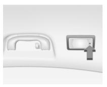
Switch on reading lights by pressing + on the cover.
