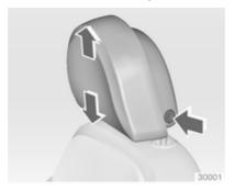
Press release button, adjust height, engage.
