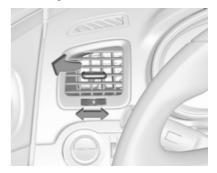
To close the vent, turn the adjuster wheel to **0**.
