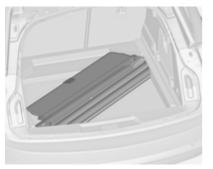
Put the load compartment cover into the hollow with the upper side downwards and with the release lever in the front right edge.
