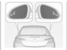
When the vehicle is started, both exterior mirror displays will briefly come on to indicate that the system is operating.
