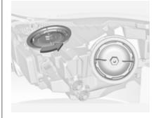
Rotate the cap anticlockwise and remove it.
