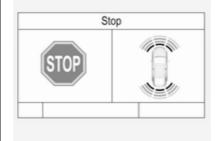
The suggestion of the system is accepted when the vehicle is stopped by the driver within 10 metres after the message is given. The system calculates the optimal route into the parking slot. Then it manoeuvres the driver into the slot by giving detailed instructions.
