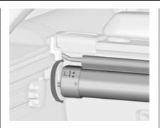
To unlock, turn cassette slightly backwards and remove it upwards from the retainers.
