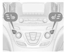
Adjust heating to the desired setting by pressing button # for the respective seat one or more times. The control indicator in the button indicates the setting.
