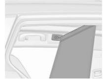
Front installation openings in the roof frame: latch rod of the net at one side, compress rod and latch at the other side.
