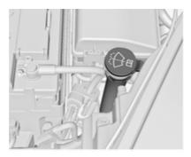
Fill with clean water mixed with a suitable quantity of windscreen washer fluid which contains antifreeze. For the correct mixing ratio refer to the washer fluid container.
