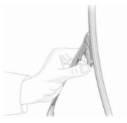
Lift the wiper arm. Press the two catches on the arm, disengage the wiper blade and remove.
