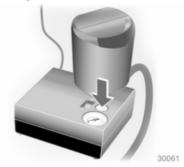
If the prescribed tyre pressure is not obtained within 10 minutes, remove the tyre repair kit. Move the vehicle one tyre rotation. Reattach the tyre repair kit and continue the filling procedure for 10 minutes. If the prescribed tyre pressure is still not obtained, the
