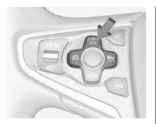
Press button 3%, the current setting is shown in the Driver Information Centre. Press button 3% again to change the following distance. The setting is also displayed in the Driver Information Centre.
