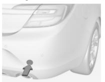
5-door Hatchback, 4-door Saloon, Sports Tourer, OPC: disengage cap at bottom and remove downwards.
