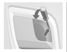
**OPC:** insert screwdriver in the slot at the upper bend of the cap. Release the cap by carefully moving the screwdriver downwards. To prevent damage it is recommended to place a cloth between the screwdriver and the frame.
