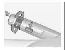
On Baselevel display, select **Settings** with the Menu button and select **Traffic sign detection** entry via the adjuster wheel on the turn signal lever \$ 107.
