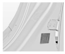
The identification label is located on the front left door frame.
