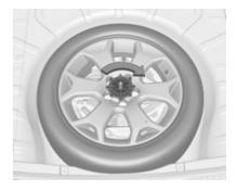
Store the tool box and the damaged wheel outside up in the spare wheel well and secure it by turning the wing nut clockwise on the bolt.
