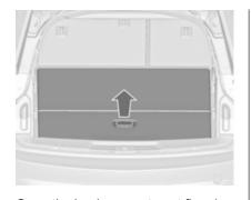
Open the load compartment floor by pulling the handle. Fold and place the floor behind the rear seats.
