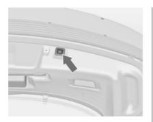
To close, press button in the open tailgate until the tailgate starts to move.
