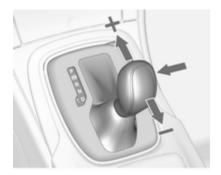
Move selector lever out of position **D** towards the left to select manual mode.
