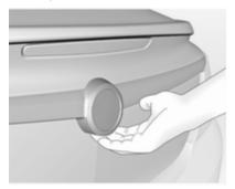
After unlocking, press the button under the tailgate moulding and open the tailgate manually.
