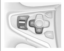
Press button @. The control indicator @ in the instrument cluster illuminates white. If cruise control or adaptive cruise control has been activated before, it is switched off when speed limiter is activated and the control indicator (\*\*) extinguishes.
