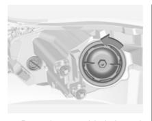
Rotate the cap anticlockwise and remove it.
