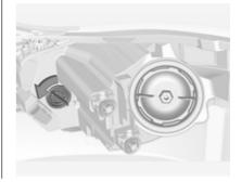
Rotate bulb socket anti-clockwise to disengage. Withdraw the bulb socket from the housing.
