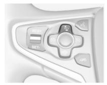
Press button ♣, the current setting is shown in the Driver Information Centre. Press button ♣ again to change the alert sensitivity.
