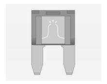
Depending on the type of fuse, a blown fuse can be recognized by its melted wire. Do not replace the fuse until the cause of the fault has been remedied.
