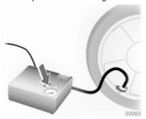
If tyre pressure is more than 1.3 bar, set it to the correct value. Repeat the procedure until there is no more loss of pressure.
