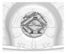
The jack with wheel wrench, the tools, an extension bolt for securing a damaged wheel and the towing eye are placed in the tool box below the spare wheel in the load compartment. Spare wheel ▷ 250.
