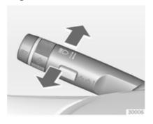
To switch from low to high beam, push lever.
