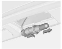
3. Remove bulb holder from lamp housing by turning anticlockwise.
