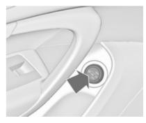
Press and hold button with until the tailgate starts to open or close.
