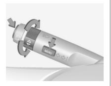
On Baselevel display select the **Settings** Menu by pressing the **MENU** button on the turn signal lever. Turn the adjuster wheel to select the **Remaining Oil Life** page.
