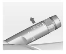
= automatic wiping with rain sensor
