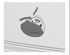
5-door Hatchback, 4-door Saloon, Sports Tourer, OPC: insert cap at the bottom, turn slightly clockwise and engage cap.
