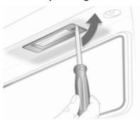
Insert screwdriver in bulb housing, press to the side and release spring.
