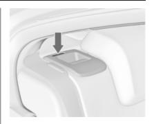
The backrests are properly engaged when both red marks on the side near the release lever are no longer visible.
