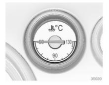
Displays the coolant temperature.
