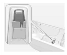
Open the centre console storage area by lifting up the armrest. Place the electronic key in the transmitter pocket. Depress the clutch pedal (manual transmission) or the brake pedal (automatic transmission) and press the **Engine Start/Stop** button.
