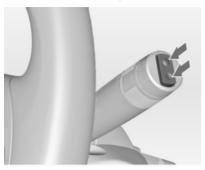
Push the rocker switch to activate the rear window wiper:
