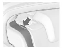
Put the seat belts of the outboard seats into the belt guides.
