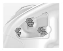
2. Unscrew three plastic securing nuts from the inside by hand.
