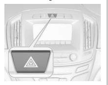
Operated with the <u>▲</u> button. Hazard warning flashers ▷ 128.
