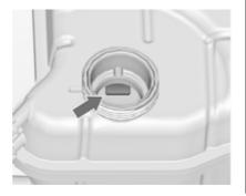
On another version the filling line mark is inside the filler opening. To check open the cap.
