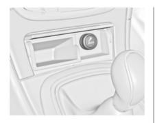
Press in cigarette lighter. It switches off automatically once the element is glowing. Pull out lighter.
