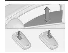
Press button d again for three seconds after unlocking: all windows will be opened.
