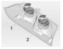
4. Rotate plastic nut anticlockwise and remove from the bulb holder.
