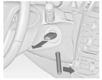
Turn special tool to the front and remove key from the ignition switch. Several attempts may be required to successfully remove the key.
