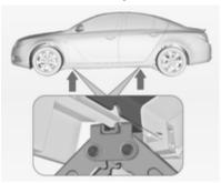
Ensure the jack is correctly positioned under the relevant vehicle jacking point.
