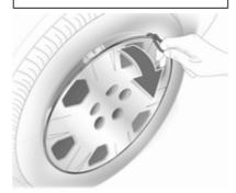
Alloy wheels: Disengage wheel nut caps with a screwdriver and remove. To protect the wheel, place a soft cloth between the screwdriver and the alloy wheel.
