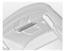
Stow the warning triangle in the space behind the straps on the inside of the tailgate.
