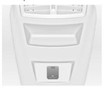
A 230 Volt power outlet is located in the rear centre console. If ignition is on and a device is plugged in, an LED in the outlet illuminates green.
