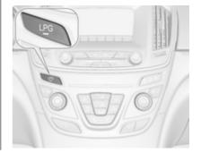
Press the **LPG** button to switch between petrol and liquid gas operation as soon as the required parameters (coolant temperature, gas temperature and minimum engine speed) have been reached. The requirements are usually fulfilled after around 60 seconds (depending on exterior temperature) and the first firm press on the accelerator. The LED status shows the current operating mode.
