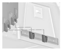
Alternatively install both hooks in the lower rail. Plug in the lower brackets of the box from above into the lower hooks.
