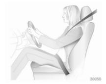
Sit with buttocks as far back against the backrest as possible. Adjust the distance between the seat and the pedals so that legs are slightly angled when pressing the pedals. Slide the front passenger seat as far back as possible.
