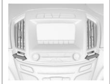
To open the vent, turn the adjuster wheel to I. Adjust the air amount at the vent outlet by turning the adjuster wheel.
