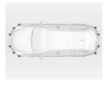
The advanced parking assist system manoeuvres the driver into a parking slot by giving instructions in the Driver Information Centre and acoustic signals.
