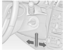
Insert the special tool into the opening below the ignition switch as far as it will go and swivel it slightly.
