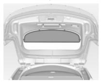
To cover the load compartment completely, mount the blind at four fixing points on the inside of the tailgate.
