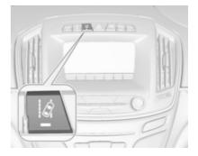
The lane departure warning system is activated by pressing the la button. The illuminated LED in the button indicates that the system is switched on. When the control indicator la in the instrument cluster illuminates green, the system is ready to operate.
