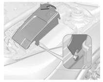
The vehicle battery is covered. Remove the cover to replace the battery. Lift up the cover at the rear and unlatch it at the front.
