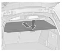
Push down the handle at the end of the cover. It rolls up automatically.
