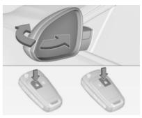
Press button ⓐ again after locking for one second to fold in mirrors.
