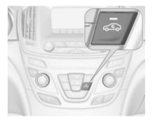
Press button \$\simes \text{to activate air recirculation mode. Activation is indicated by the LED in the button.}
