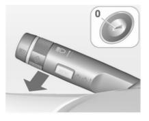
Headlights, tail lights and number plate lights illuminate the surrounding area for an adjustable time after leaving the vehicle.
