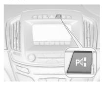
When looking for a parking slot, the system must be activated by pressing the per button.
