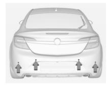
The front-rear parking assist measures the distance between the vehicle and obstacles in front and
