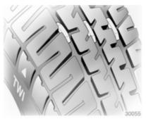
The legally permissible minimum tread depth (1.6 mm) has been reached when the tread has worn down as far as one of the tread wear
