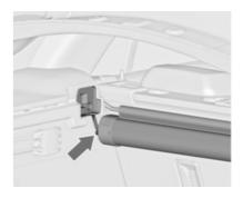
Insert the cassette into the retainers on left and right side. Note the signs  $\bf L$  (left side) and  $\bf R$  (right side) on the cassette as an installation hint.
