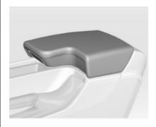
Push button and fold armrest upwards. Under the armrest there is a storage compartment.
