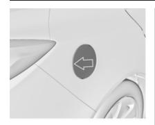
The fuel filler flap can only be opened if the vehicle is unlocked. Pull flap at the recess and open.
