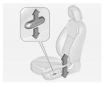
Move switch upwards/downwards.
