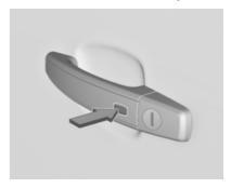
Electronic key system: Unlocking the vehicle by pressing the button on any exterior door handle deactivates antitheft alarm system.
