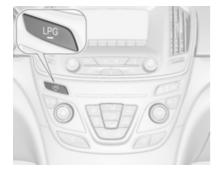
Pressing button **LPG** switches between petrol and liquid gas operation. The status LED — shows the current operating mode.
