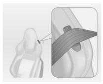
Feed seat belt through belt mount on backrest when fastening seat belt.
