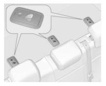
Open the flap of the required fastening eye, marked by the child seat symbol.
