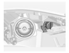
Rotate cap anticlockwise and withdraw from the reflector.
