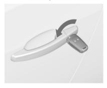
Manually unlock the driver's door by turning the key in the lock. Switch on the ignition and press the central locking button to unlock all doors, load compartment and fuel filler flap. By switching on the ignition, the antitheft locking system is deactivated.
