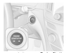
power button: press **Engine Start/ Stop** button and release
