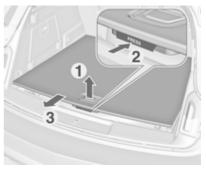
Press the button under the handle and pull out the floor cover until it engages.
