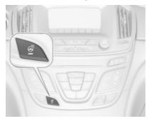
Activate heating by pressing **a** button. Activation is indicated by the LED in the button.
