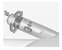
Press the **MENU** button to switch between the main menus or to return from a submenu to the next higher menu level.
