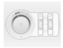
When the automatic light control function is switched on and the engine is running, the system switches between daytime running light and low/high beam automatically depending on the lighting conditions and information given by the rain sensor system.
