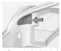
Remove cover from the inside of the load compartment.
