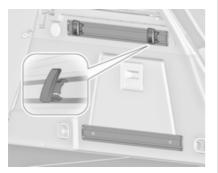
Insert the hook in the desired position first into the upper groove of the rail and then press into the lower groove. To remove, first pull out of the upper groove.
