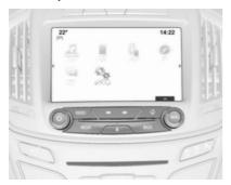
Press button  $\odot$  to switch on the display.
