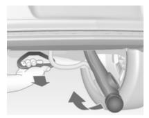
Pull the grip located left to the number plate under the rear bumper fascia at an angle of approx. 45° to the ground.
