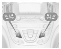
Adjust ventilation to the desired setting by pressing button ⋬ for the respective seat one or more times.
