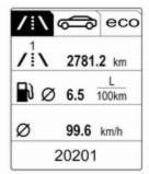
The menu pages of the Baselevel display are selected by pressing the **MENU** button on the turn signal lever. Main menu symbols are indicated in the top line of the display:
