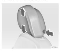
**Height adjustment**Press release button, adjust height, engage.
