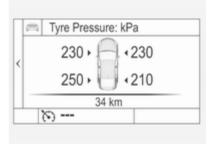
System status and pressure warnings are displayed by a message with the corresponding tyre flashing in the Driver Information Centre.
