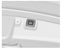
Press and hold the button on the inside of the open tailgate for 3 seconds.
