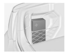
Stow the first aid kit in the space behind the mesh net on the left side of the load compartment.
