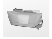
On left vehicle side, slide lamp to the front and remove it out of the fender with the rear end.
