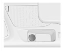
12 Volt power outlets are located in the front and rear centre console.
