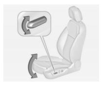
Move front of switch upwards/downwards.
