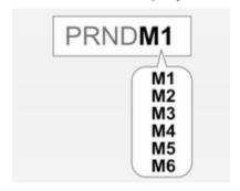
The driving programme in automatic mode or the selected gear in manual mode is indicated in the Driver Information Centre.
