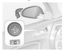
Switch control to ●, then push the control button ₹ down. Both exterior mirrors will fold.
