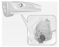
Turn the bulb holder anticlockwise and remove it from the reflector.
