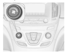
Adjust the air flow by turning the controller % to the desired speed. O means fan off.
