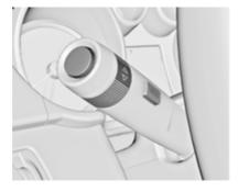
On Baselevel display press the **SET/ CLR** button, the **MENU** button or turn the adjuster wheel to confirm a message.
