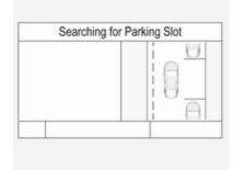
When the vehicle passes a row of cars and the system is activated, the advanced parking assist system begins looking for a suitable parking slot. When a suitable slot is detected,
