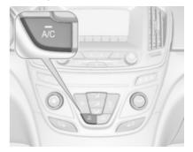
Press button **A/C** to switch on cooling. Activation is indicated by the LED in the button. Cooling is only functional when the engine is running and climate control fan is switched on.
