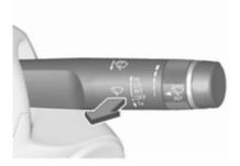
Pull lever. Washer fluid is sprayed onto the windscreen and the wiper wipes a few times.
