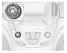
Adjust the air flow by turning the controller  $\Re$  to the desired speed. O means fan off.
