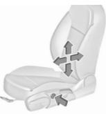
Adjust lumbar support using the fourway switch to suit personal requirements.
