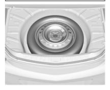
The spare wheel is located in the load compartment beneath the floor covering.
