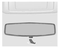
To reduce dazzle, adjust the lever on the underside of the mirror housing.
