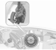
2. Rotate the bulb holder anticlockwise to disengage. Withdraw the bulb holder from the reflector.
