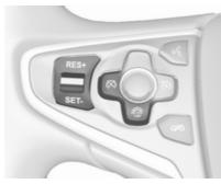
Press @. The control indicator @ in the instrument cluster illuminates white. If cruise control or adaptive cruise control has been activated before, it is switched off when speed limiter is activated and control indicator (%) extinguishes.
