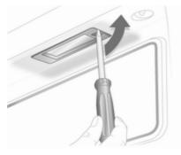
1. Insert screwdriver in bulb housing, press to the side and release spring.
