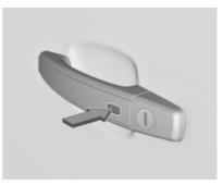
Electronic key system: Unlocking the vehicle by pressing the button on any exterior door handle deactivates antitheft alarm system. The system is not deactivated when unlocking the driver's door with the key or with the central locking button in the passenger compartment.
