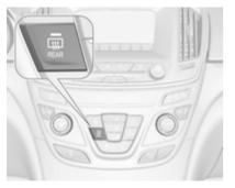
Heating is operated by pressing . Heated rear window  $\diamondsuit$  43. Demisting and defrosting the windows, air conditioning system
