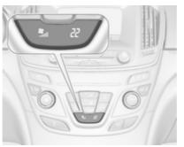
Settings of temperature and fan speed are indicated in the climate display.
