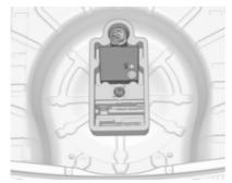
The tyre repair kit is in a compartment under the floor cover in the load compartment.
