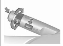
On Baselevel display, select **Settings**  ⇔ by pressing **MENU** and select **Traffic sign detection** entry with the adjuster wheel on the turn signal lever ¢ 111.
