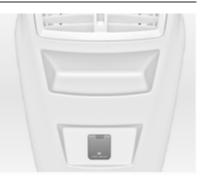
A 230 Volt power outlet is located in the rear centre console. If ignition is on and a device is plugged in, an LED in the outlet illuminates green.
