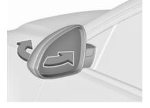
For pedestrian safety, the exterior mirrors will swing out of their normal mounting position if they are struck with sufficient force. Reposition the mirror by applying slight pressure to the mirror housing.
