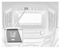
The lane departure warning system is activated by pressing lâ. The illuminated LED in the button indicates that the system is switched on. When the control indicator lâ in the instrument cluster illuminates green, the system is ready to operate.
