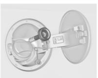
**ACME Adapter:** Screw the nut of the filling nozzle onto the adapter. Press locking lever on filler nozzle down.
