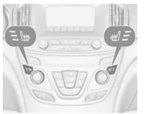
Prolonged use of the highest setting for people with sensitive skin is not recommended. Seat heating is operational when engine is running and during an Autostop.
