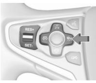
Press % to switch on adaptive cruise control. The control indicator  $\mathfrak{B}$  or  $\mathfrak{K}$  in the instrument cluster illuminates white.
