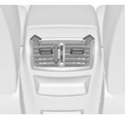
Air vents for rear passenger are in the centre console between the front seats.
