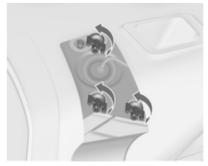
2. Unscrew three plastic securing nuts by hand.
