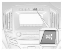
When searching for a parking slot, the system is ready to operate by pressing button P#2.
