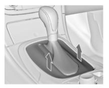
Release selector lever trim from centre console at rear, fold upwards and rotate to the left.
