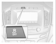
TC can be switched off when spinning of drive wheels is required:
