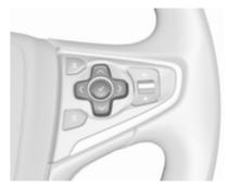
On Midlevel and Uplevel display select **Info** menu with the right steering wheel buttons and press ✓ to select **Traffic sign detection** ♀ 111.
