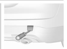
**Country Tourer:** insert a screwdriver in the slot at the lower edge of the cap. Release the cap by carefully moving the screwdriver downwards. To prevent damage, it is recommended to place a cloth between the screwdriver and the frame.
