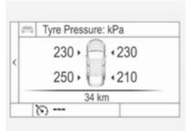
System status and pressure warnings are displayed by a message indicating the corresponding tyre in the Driver Information Centre.
