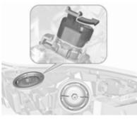
Rotate the bulb holder anticlockwise to disengage. Withdraw the bulb holder from the reflector.
