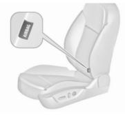
The side airbag system consists of an airbag in each front seat backrest and in the rear outboard seat backrests. This can be identified by the word **AIRBAG**.
