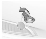
Screw in the towing eye as far as it will go until it stops in a horizontal position.
