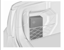
Stow the first aid kit in the space behind the mesh net on the left side of the load compartment.
