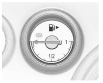
Displays the level in the fuel or gas tank depending on the operation mode.
