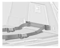
Insert the adapters of the strap set into a rail. Make sure that the belt is not twisted.
