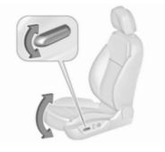
Tilt front of switch upwards/ downwards.
