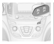
If the control indicator  $\Re_2$  illuminates, the front passenger airbag system will inflate in the event of a collision.
