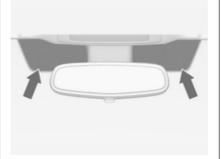
The marked areas on the windscreen are not covered with the coating. Devices for electronic data recording and fee payment must be attached in these areas. Otherwise data recording malfunctions may occur.
