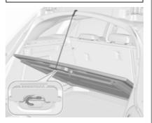
For access to the spare wheel or tyre repair kit, lift up the floor cover and attach the retaining strap at the upper edge of the tailgate recess. Lift up and attach the cover only without loading.
