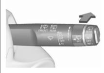
Push lever. Washer fluid is sprayed onto the rear window and the wiper wipes a few times.
