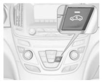
Press Solution to activate air recirculation mode. The LED in the button illuminates to indicate activation.
