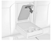
Pull grip and open the cover. Suitable for loading long, narrow objects.
