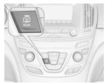
Operated by pressing . The LED in the button indicates activation. Heating works with the engine running and is switched off automatically after a short time.
