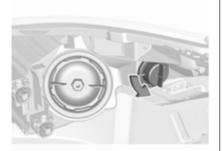
1. Rotate cap anticlockwise and withdraw from the reflector.
