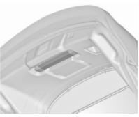
Stow the warning triangle in the space behind the straps on the inside of the tailgate.
