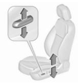
Move switch upwards/downwards.
