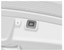
4. Press and hold the button on the inside of the open tailgate for 3 seconds.
