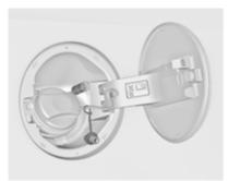
Screw the required adapter hand-tight onto the filler neck.
