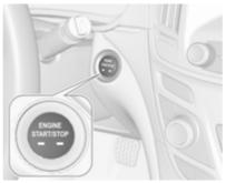
Power button: press **Engine Start/Stop** and release.
