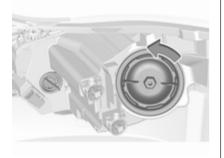
1. Rotate the cap anticlockwise and remove it.
