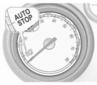
An Autostop is indicated by the needle at the **AUTOSTOP** position in the tachometer. On some versions, a control indicator in the instrument cluster illuminates when engine is in Autostop.
