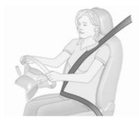
The seat belts are locked during heavy acceleration or deceleration of the vehicle holding the occupants in the sitting position. Thereby the risk of injury is considerably reduced.
