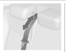
The seat belt of the centre seat could be blocked when the backrest is folded up too quickly. To unlock the retractor, push in the seat belt or pull it out by approx. 20 mm and then release.
