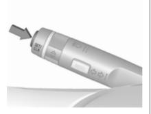
The alert function can be activated or deactivated in the setting menu of the traffic sign assistant page by pressing **SET/CLR** on the turn signal lever or  $\checkmark$  on the steering wheel.
