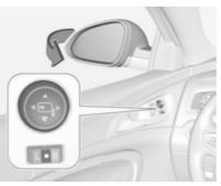
Switch control to  $\bullet$ , then push the control button  $\nabla$  down. Both exterior mirrors will fold.
