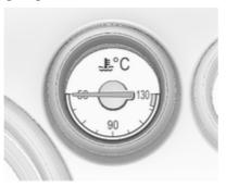
Displays the coolant temperature.
