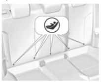
Fasten vehicle-approved ISOFIX child restraint systems to the ISOFIX mounting brackets. Specific vehicle ISOFIX child restraint system positions are marked in the table by IL ¢ 66.
