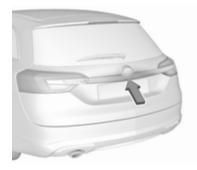
To open the tailgate, press the touchpad switch under the tailgate moulding until the tailgate starts to move.
