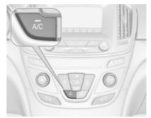
Press **A/C** to switch on cooling. Activation is indicated by the LED in the button. Cooling is only functional when the engine is running and climate control fan is switched on.
