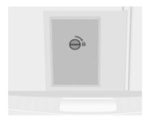
The closed cover can be secured from inside the load compartment. Turn knob by 90°:
