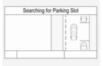
When the vehicle passes a row of cars and the system is activated, the advanced parking assist system begins looking for a suitable parking slot. When a suitable slot is detected, a visual feedback and acoustic signals are given in the Driver Information Centre.
