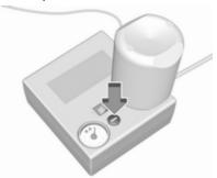
If the prescribed tyre pressure is not obtained within 10 minutes, remove the tyre repair kit. Move the vehicle one tyre rotation. Reattach the tyre repair kit and continue the filling procedure for 10 minutes. If the prescribed tyre pressure is still not obtained, the tyre is too badly damaged. Seek the assistance of a workshop.
