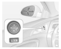
Select the relevant exterior mirror by switching the control to left mirror (L) or right mirror (R). Then swivel the control to adjust the mirror.
