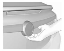
After unlocking, press the button under the tailgate moulding and open the tailgate manually.
