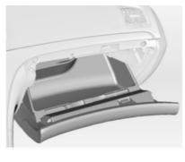
The glovebox features a pen holder, a coin holder and an adapter for the locking wheel nuts.
