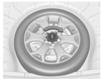
Store the tool box and the damaged wheel outside up in the spare wheel well and secure it by turning the wing nut clockwise on the bolt.
