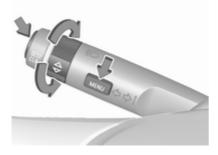
On Baselevel display select the **Settings** Menu by pressing **MENU** on the turn signal lever. Turn the adjuster wheel to select the **Remaining Oil Life** page.
