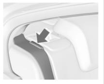
Put the seat belts of the outboard seats into the belt guides.
