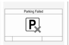
If an object is detected during parking instructions, **Stop** is indicated in the Driver Information Centre. Removing the object will resume the parking manoeuvre. If the object is not removed, the system will be deactivated. Press P#D to activate the system and search for a new parking slot.
