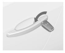
Manually unlock the driver's door by turning the key in the lock. Switch on the ignition and press the central locking button T to unlock all doors, load compartment and fuel filler flap. By switching on the ignition, the antitheft locking system is deactivated.
