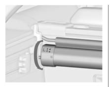
To unlock, turn cassette slightly backwards and remove it upwards from the retainers.
