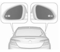
When the vehicle is started, both exterior mirror displays will briefly come on to indicate that the system is operating.
