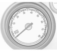
Displays the engine speed.
