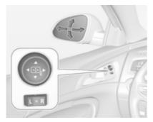
Select the relevant exterior mirror by switching the control to left mirror (L) or right mirror (R), then adjust.
