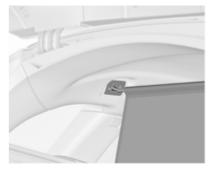
Pull out the net from the cassette and latch the rod of the net at one side into the rear installation opening in the roof frame. Compress the rod and latch at the other side.
