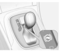
Without applied brake pedal the control indicator (S) illuminates.
