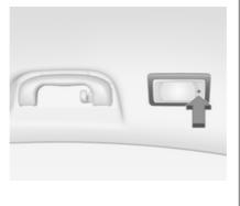
Switch on reading lights by pressing + on the cover.
