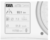
The recorded distance since the last reset is displayed on the trip computer page. Two trip odometer are selectable for different trips.
