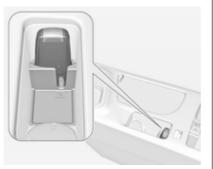
Open the centre console storage area by lifting up the armrest. Place the electronic key in the transmitter pocket.
