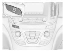
Press **LPG** to switch between petrol and liquid gas operation as soon as the required parameters (coolant temperature, gas temperature and minimum engine speed) have been reached. The requirements are usually fulfilled after approximately 60 seconds (depending on exterior temperature) and the first firm press on the accelerator. The status LED shows the current operating mode.
