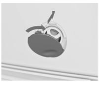
5-door Hatchback, 4-door Saloon, Sports Tourer, OPC: insert cap at the bottom, turn slightly clockwise and engage cap.
