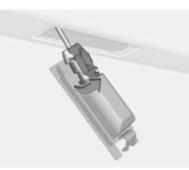
2. Remove lamp downwards, taking care not to pull on the cable.
