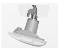
2. Turn bulb holder anticlockwise and remove from housing.
