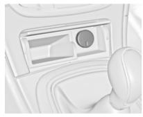
A 12 Volt power outlet is behind the storage cover below the climate controls. Press cover to open.
