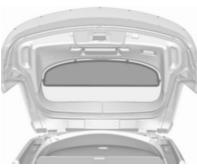
To cover the load compartment completely, mount the blind at four fixing points on the inside of the tailgate.
