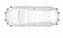
The advanced parking assist system manoeuvres the driver into a parking slot by giving instructions on the Driver Information Centre and acoustic signals. The driver must control acceleration, braking, steering and gear shifting.
