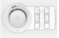
When the automatic light control function is switched on and the engine is running, the system switches between daytime running light and low/high beam automatically depending on the lighting conditions and information given by the rain sensor system.
