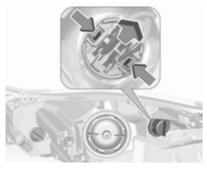
Press snap-in tongues together and move socket out of the housing.
