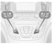
Adjust ventilation to the desired setting by pressing ≝ for the respective seat one or more times.
