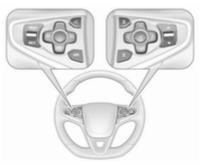
Driver Information Centre, some driver assistance systems, Infotainment system and a connected mobile phone can be operated via the controls on the steering wheel.
