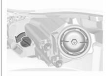
1. Rotate bulb socket anticlockwise to disengage. Withdraw the bulb socket from the housing.
