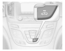
Press So to activate air recirculation mode. The LED in the button illuminates to indicate activation.
