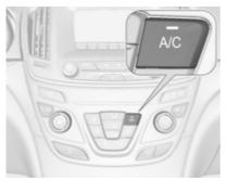
Press **A/C** to switch on cooling. The LED in the button illuminates to indicate activation. Cooling is only functional when the engine is running and climate control fan is switched on.
