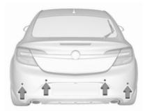
The front-rear parking assist measures the distance between the vehicle and obstacles in front and behind the vehicle. The system gives acoustic signals and display messages.
