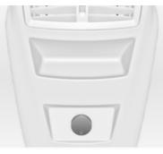
Do not exceed the maximum power consumption of 120 watts.
