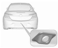
The camera is mounted between the number plate lights and has a viewing angle of 130°.
