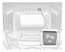
An illuminated LED in the parking assist button  $\mathbf{P}$ <sup>w</sup> indicates that the system is ready to operate.
