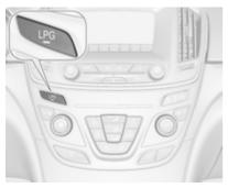
Pressing LPG switches between petrol and liquid gas operation. The status LED — shows the current operating mode.
