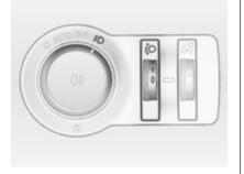
To adapt headlight range to the vehicle load to prevent dazzling: turn thumb wheel <sup>€D</sup> to required position.
