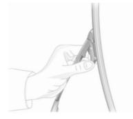
Lift the wiper arm. Press the two catches on the arm, disengage the wiper blade and remove.
