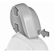
Height adjustment Press release button, adjust height, engage.
