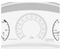
Depending on settings of the Uplevel display, gauges for "Oil temperature", "Oil pressure" or "Battery voltage" are also displayed on the left and right of the speedometer.
