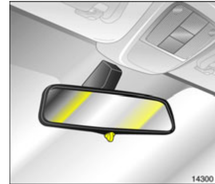
Interior mirror Swivel mirror housing to adjust. Manual anti-dazzle interior mirror To reduce dazzle, swivel the lever on the underside of the mirror housing.
