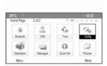
Press the multifunction knob (Navi 950 / Navi 650: press the outer ring) to display the second **Home**Page with further applications.
