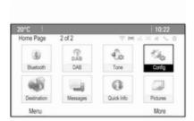
Press the multifunction knob (Navi 950: press the outer ring) to display the second **Home Page** with further applications.
