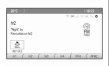
Each waveband has 2 autostore lists (AS 1, AS 2), in each of which 6 stations can be stored.
