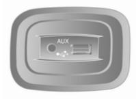
In the Infotainment unit (or in the centre console) there is a USB socket  $\Psi$  for the connection of external audio sources.
