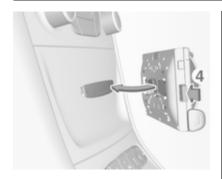
Attach the phone holder to the power connector and press both locking shifters (4) to lock.
