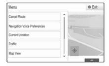
Select **Current Location** to display the respective submenu indicating details on the nearest address, the coordinates, and Points of interest (\$\dip\$ 50) around the current location.
