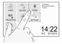
Touch and hold the element you wish to move until red boxes appear around the icons. Move your finger to the desired location and release the element
