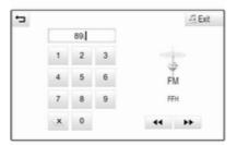
Touch the **Direct Tune** field and then enter the desired frequency. Confirm your input.
