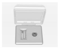
In the centre console there is an AUX socket for the connection of external audio sources.
