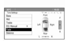
To adjust the volume distribution between the front and rear speakers in the vehicle, select the **Fade** menu item. Adjust the setting as desired.
