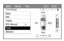
To adjust the volume distribution between the front and rear speakers in the vehicle, select **Fade**. Adjust the setting as desired.
