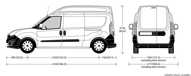
Maximum load length Panel Van 2170 (85.4) Maximum load width 1714 (67.5) At widest point Between wheel arches 1230 (48.4) Maximum load height Maximum height 1550 (61.0) Rear and side load door(s) 1455 (57.2) Rear door aperture height Rear door aperture width 1231 (48.5) Side door aperture height 1175 (46.2) Side door aperture width 700 (27.5) Loading height Unladen 545 (21.4)
