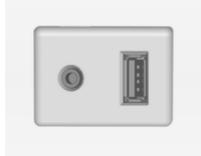
In the centre console below the climate controls, there is an AUX socket and a USB socket for the connection of external audio data sources.
