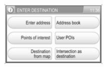
The ENTER DESTINATION menu is the main entry point for entering and/or selecting destinations, see "Entering an address directly" and subsequent paragraphs below.
