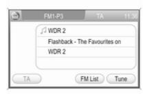
Example FM radio menu: buttons TA, FM List and Tune can only be selected/activated via the touch screen.
