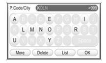
Successively select the letters for the desired city name. During this process the system will automatically block letters that cannot occur next in the city name.
