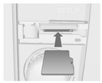
Push the SD card with the labelled side upward, and the cut-outs on the right side (see image above), carefully into the SD card slot until the card engages.
