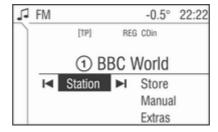
The items within a menu are selected by using a cursor moved by turning the multifunction knob. The cursor has the shape of a frame (bar). The cursor indicates which menu item is being selected.
