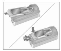
Insert the mobile telephone into the adapter
