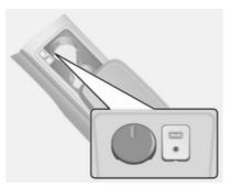
In the centre console there is an USB socket for the connection of external audio data sources.
