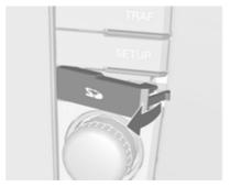
The cover can be removed, e.g., with means of a small paper clip or similar items.
