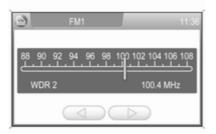
Press the ◄ or ► button (on the instrument panel) and keep it pressed. Release the button when the required frequency has almost been reached on the scale.
