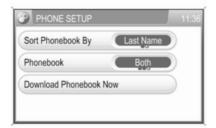
To open the PHONE SETUP menu: press the SETUP button, select the Bluetooth & telephone menu item and then select the Telephone settings menu item.
