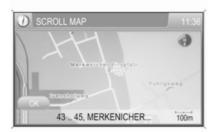
If required, you can move the visible map section in an arbitrary direction by moving your finger on the screen, and change the map scale by turning the multifunction knob.
