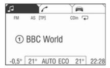
The main menu is the display which only provides information. Three different main menu views can be selected: audio, Mobile phone portal and on-board computer.
