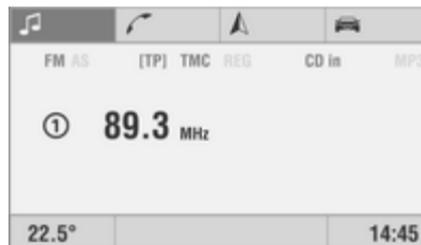
Information about the currently selected audio source (e.g. waveband, station name or frequency or CD track and track number, etc.).
