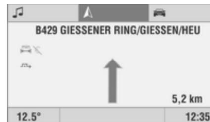
After the route has been calculated, guidance takes place by means of voice output and directional arrows.
