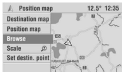
If the position map or the destination map is displayed, the cursor shown can be moved using the rocker switch.
