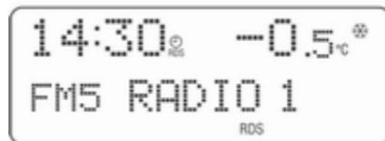
If the station currently selected is not an RDS station, the radio searches automatically for the next receivable RDS station.
