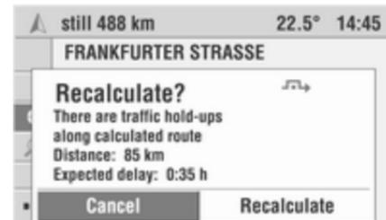
With dynamic guidance, the whole of the current traffic situation that is received by the Infotainment system via RDS TMC is incorporated into the calculation of the route.
