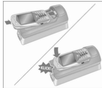
Insert the mobile telephone into the adapter
