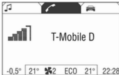
When the mobile telephone is slotted in the adapter, the telephone menu or **Bluetooth™** menu appear on the display.
