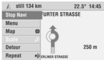
On the left-hand side of the guidance screen a small menu bar with symbols is displayed. The menu with the complete menu texts expands when you turn the multifunction knob.
