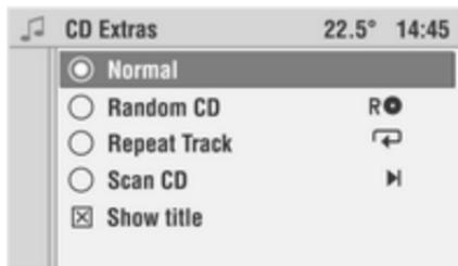
Various further functions for CD/MP3 playback can be set using the **CD Extras** menu.
