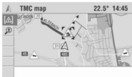
Traffic messages which the Infotainment system is currently receiving via RDS TMC can be displayed on the **TMC map** as symbols. In addition, detailed information on each of the traffic problems displayed on the map can be recalled.
