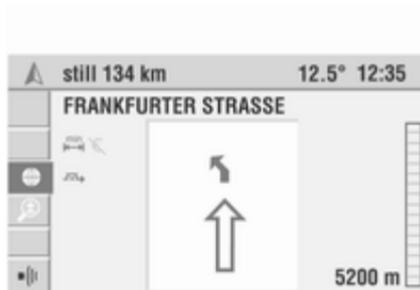
If the "detailed arrows" function is active, an additional and simplified early warning is displayed above the directional arrow that informs you about the next change in driving direction well in advance.
