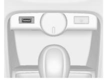
In the centre console there is a USB socket for the connection of external audio data sources.
