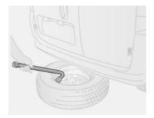
4. Withdraw spare wheel from beneath the vehicle.
