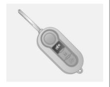
Press button € : Front doors are unlocked.
