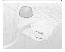
If the cooling system is cold, the coolant level should be between the **MIN** and **MAX** mark. Top up if the level is low.
