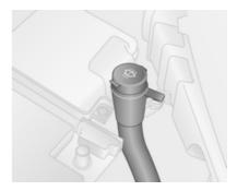
Fill with clean water mixed with a suitable quantity of windscreen washer fluid which contains antifreeze.
