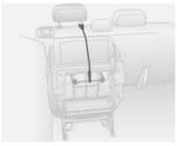
Secure the folded seat in the upright position by attaching the flexible cord located on the seat frame, to the rear seat head restraint.
