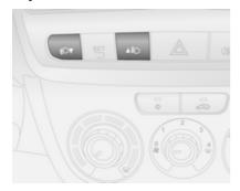
To adapt headlight range to the vehicle load to prevent dazzling of other road users: Press ♥○ or ♠○ buttons until the required setting is displayed in the Driver Information Centre ♀ 79.
