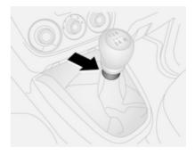
To engage reverse, with the vehicle stationary, wait 3 seconds after depressing the clutch pedal, pull up the collar on the selector lever and engage the gear.
