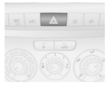
Operated with the <u>▲</u> button. Hazard warning flashers ♀ 90.
