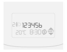
Displays the recorded distance in km. **H** may appear in the display until the vehicle has travelled 100 km.
