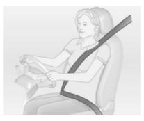
Pull out the seat belt and engage in belt buckle. The seat belt must not be twisted and must fit close against the body. The backrest must not be tilted back too far (maximum approx. 25°).
