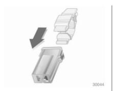
Place the fuse extractor on the various types of fuse from the top or side, and withdraw fuse.
