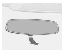
Adjust the lever on the underside to reduce dazzle.
