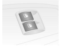
Operate the switch for the respective window by pushing to open or pulling to close.
