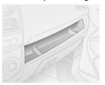
Storage compartments are located in the instrument panel.
