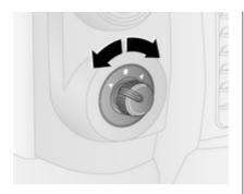
Select the relevant exterior mirror by turning the control to left ◀ or right ►. Then swivel the control to adjust the mirror.
