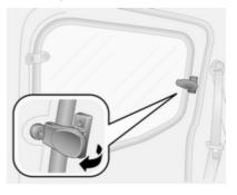
To open, move lever outwards until the window is fully open.
