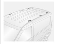
To fasten a roof rack, insert the mounting bolts in the holes indicated in the illustration.
