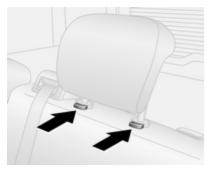
Pull the head restraint upwards or press the catch to release and push the head restraint downwards.
