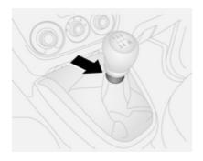
Reverse: with the vehicle stationary, wait 3 seconds after depressing the clutch pedal, pull up the collar on the selector lever and engage the gear. If the gear does not engage, set the lever to neutral, release the clutch pedal and depress again; then repeat gear selection.
