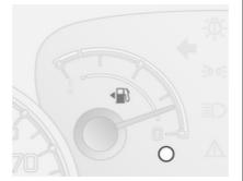
Displays the fuel level or gas level in the tank depending on the operation mode. During natural gas operation, the system automatically switches over to petrol operation when the gas tanks are empty ⊅ 70. Fuel selector ⊅ 119.
