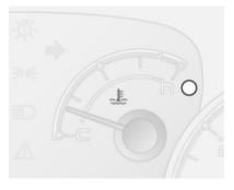
Displays the coolant temperature.
