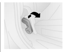
Pull lever to release, the seat base is tensioned and will start to rise automatically.
