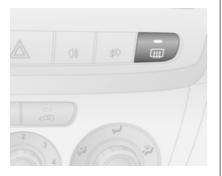
Operated by pressing the wbutton. Heating works with the engine running and is switched off automatically after a short time.
