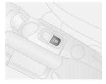
ASR can be switched off when spinning of drive wheels is required: press button **ASR OFF** briefly.
