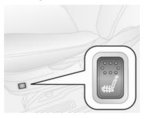
Activate seat heating by pressing button # for the respective front seat with the ignition on.
