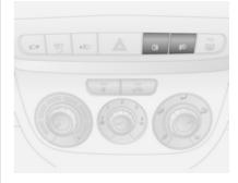
Operated by pressing the \$D button. Switching on front fog lights will switch sidelights on automatically. Press the button again to turn the front fog lights off.
