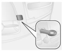
Release the cap by carefully lifting with a screwdriver. To prevent damage, it is recommended to place a cloth between the screwdriver and the frame.
