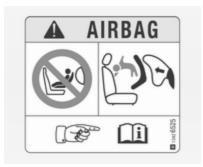
EN: NEVER use a rear-facing child restraint system on a seat protected by an ACTIVE AIRBAG in front of it, DEATH or SERIOUS INJURY to the CHILD can occur.
