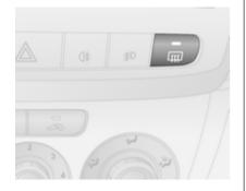
The heating is operated by pressing the ## button.
