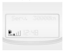
In natural gas operation mode, the four vertical bars next to **CNG** correspond to the methane level in the cylinders. As the fuel level diminishes, the bars in the CNG fuel gauge disappear.
