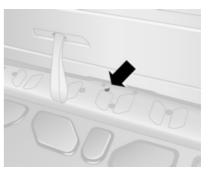
An access hole (arrowed) enables the tailgate latch to be released using a suitable tool. Push lever to the right to unlock and open the tailgate.
