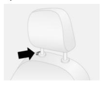
Press the button, adjust height and engage.
