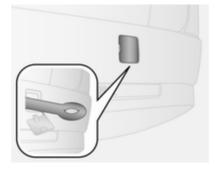
Insert a screwdriver in the slot at the side of the cap. Release the cap by carefully levering the screwdriver. To prevent damage it is recommended to place a cloth between the screwdriver and the frame.
