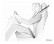
Sit with buttocks as far back against the backrest as possible. Adjust the distance between the seat and the pedals so that legs are slightly angled when pressing the pedals. Slide the front passenger seat as far back as possible.
