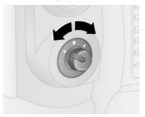
Select the relevant exterior mirror by turning the control to left ◀ or right ►. Then swivel the control to adjust the mirror.
