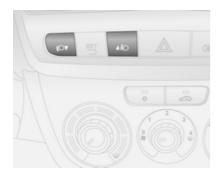
Press the **\( \)** button to scroll up the screen and the menu options or to increase the displayed value. Press and hold to increase value rapidly (press again to stop on the required value).
