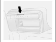
Depending on model variant, the removable rear courtesy light may illuminate when the rear doors / tailgate or sliding side doors are opened and the central switch is in the middle position.
