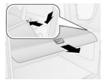
Pull the cover towards the rear using the handle and engage it in the retainers at the sides.
