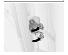
The doors are retained in the 90° position by locking stays. To open the doors to 180°, push the latch and swing open to the desired position.
