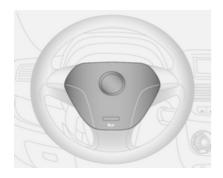
The front airbag system is triggered in the event of a front-end impact of a certain severity. The ignition must be switched on.
