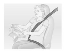
The seat belts are locked during heavy acceleration or deceleration of the vehicle holding the occupants in the sitting position. Therefore the risk of injury is considerably reduced.
