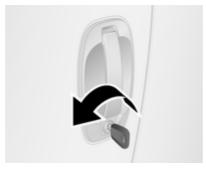
Turn the key in the driver's door lock towards the front of the vehicle.
