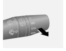
Pull lever briefly, washer fluid is sprayed onto the windscreen and the wiper wipes a few times.
