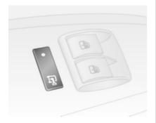
Press button 🗗: The load compartment (rear doors / tailgate and sliding side doors) are unlocked. When the load compartment is locked, the LED in the button is illuminated.
