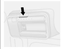
1. Press the button at the top of the lamp assembly to release it.
