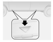
3. Vehicle jacking points are located at the front and rear.
