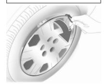
Disengage wheel nut caps with a screwdriver and remove. Pull off the wheel cover using a suitable tool. Attach wheel wrench securely and loosen each wheel nut by half a turn.
