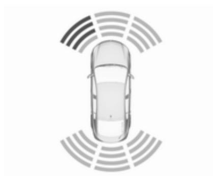
The distance to obstacles is shown on the Colour Info Display by coloured zones in front of or behind the vehicle ↻ 101.
