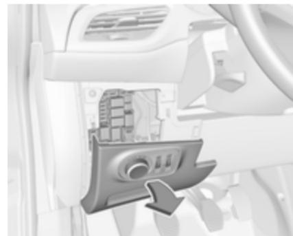
The fuse box is behind the light switch in the instrument panel. Hold the handle, then pull and fold down the light switch.
