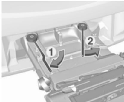
Swivel the left clamping lever (1) first, followed by the right clamping lever (2) until they stop. Both clamping levers must point backwards, otherwise safe functionality is not guaranteed.
