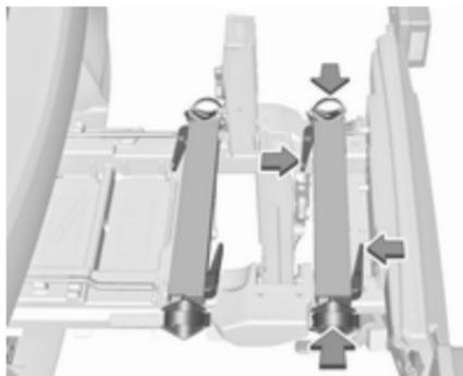
Press release lever and slide in wheel recesses all the way as far as they will go.
