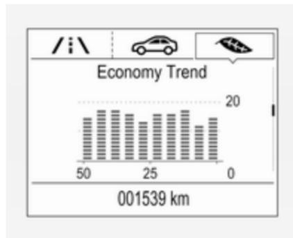
Displays the average consumption development over a distance of 50 km. Filled segments display the
