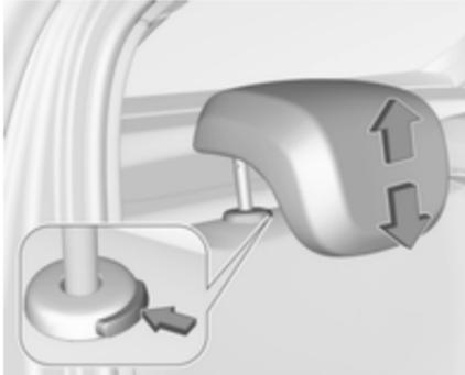
Pull the head restraint upwards and let engage. To move downwards, press the catch to release and push the head restraint downwards.
