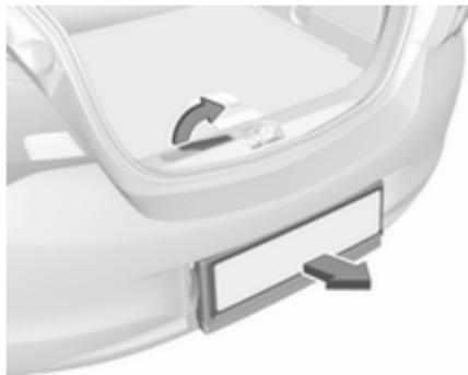
Pull release lever up. The system disengages and travels quickly out of the bumper.
