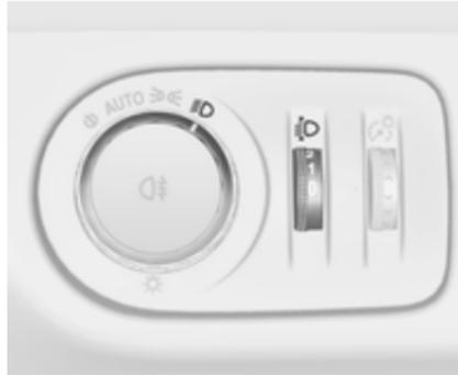
To adapt headlight range to the vehicle load to prevent dazzling: turn thumb wheel
