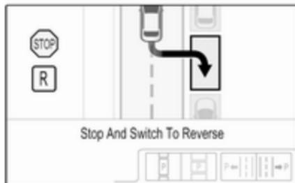
When a slot is detected, a visual feedback on the Colour Info Display and an acoustic signal is given.
