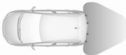
The system has four ultrasonic parking sensors in the rear bumper.
