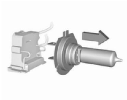
3. Detach the bulb from the bulb holder and replace the bulb.
