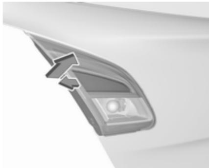
2. Move light assembly slightly to the outside, then withdraw from the tailgate.
