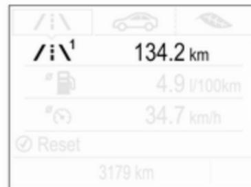
Two trip odometer pages are selectable for different trips.
