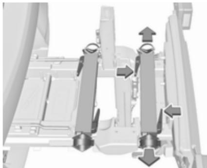
Press the release lever and withdraw the wheel recesses.
