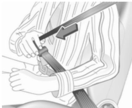
Withdraw the belt from the retractor, guide it untwisted across the body and insert the latch plate into the
