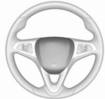
The front airbag system is triggered in the event of a front-end impact of a certain severity. The ignition must be switched on.
