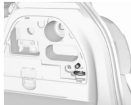
The tools and the towing eye are located on the right side of the load compartment behind a cover.
