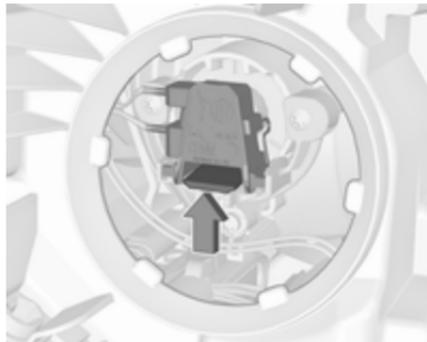
2. Press the clip to disengage bulb holder. Withdraw the bulb holder from the reflector.
