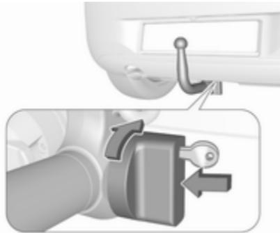
Insert the key in the lock and unlock the coupling ball bar.
