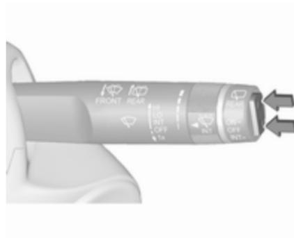
Press the rocker switch to activate the
