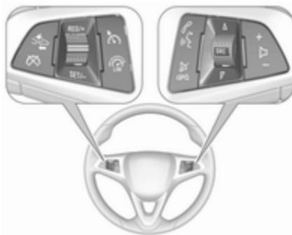
Cruise control and speed limiter are operated via the controls on the left side of the steering wheel.
