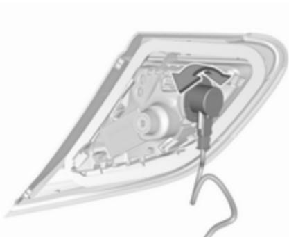
3. Remove the bulb holder by turning.
