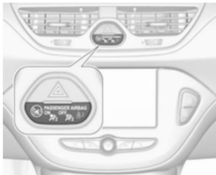
If control indicator
