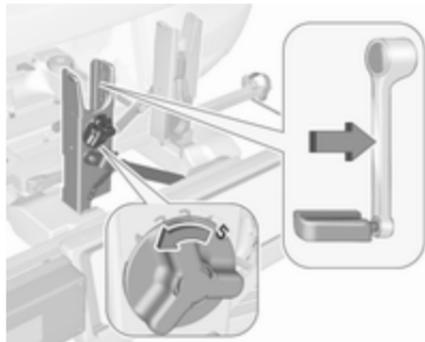
With the rotary lever on the pedal crank recess, roughly adapt the adjustable pedal crank unit to the protrusion of the pedal crank.
