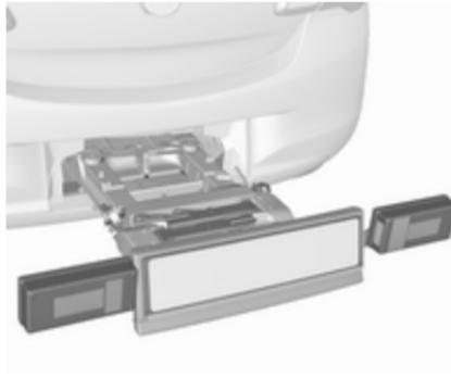
Check the cable and lamp position to ensure these are correctly installed and are securely located.
