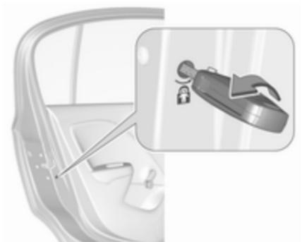
Using a key or suitable screwdriver, turn switch on rear door lock to the horizontal position. The door cannot be opened from inside.
