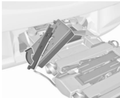
Open out the lamp support on the back of the tail lamp completely until it engages.
