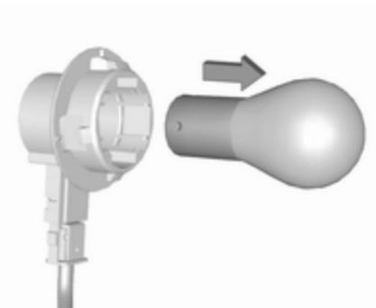
4. Remove the bulb by pushing slightly into the socket and rotating anticlockwise. Replace the bulb.
