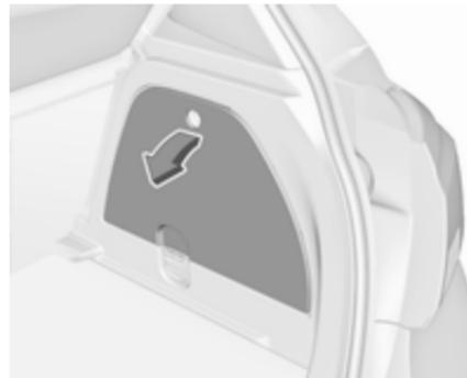
To open the compartment, disengage the cover and open it.
