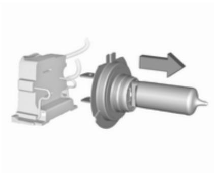
3. Detach the bulb from the bulb holder and replace the bulb.
