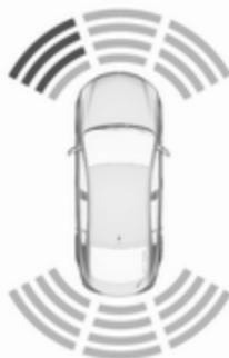
The distance to obstacles is shown on the Colour Info Display by coloured zones in front of or behind the vehicle ↪ 101.
