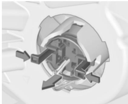
2. Press both clips together and withdraw the bulb socket from the headlamp housing.
