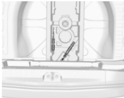
The tools are located together with the towing eye in the load compartment below the floor cover.
