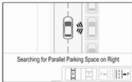
Select parallel or perpendicular parking slot by tapping the respective icon on the Info Display.
