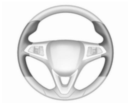
The highlighted grip areas of the steering wheel are heated quicker and to a higher temperature than the other areas.
