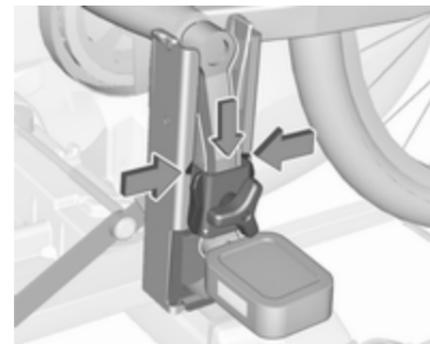
Insert pedal crank mount into outer rail of each pedal crank recess from above and slide downwards until at least underneath the notching.
