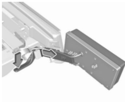
Push the clamping lever down and pull both lamp supports out of the recesses.
