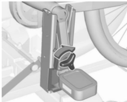
Attach the pedal crank by rotating the attachment screw on the pedal crank mount.
