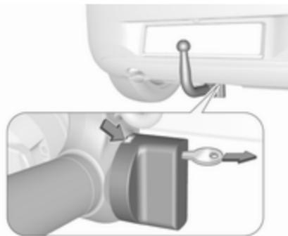
Green marking on the rotary knob is visible.
