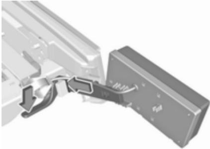
Push the clamping lever down and push the lamp support into the retainer until it engages.
