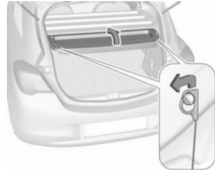
To remove rear cover, unhook retaining strings from tailgate.
