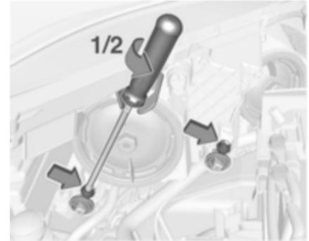
There are two adjuster elements on each headlight housing.
