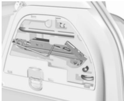
The jack, wheel bolt wrench and some tools are located on the right side of the load compartment, behind a cover ↷ 70.
