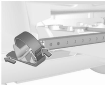
Insert the strap retainer and pull tightly downwards as far as possible.
