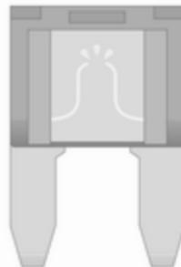
Depending on the type of fuse, a blown fuse can be recognized by its melted wire. Do not replace the fuse until the cause of the fault has been remedied.
