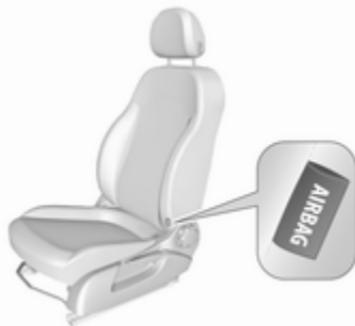
The side airbag system consists of an airbag in each front seat backrest. The location is identified by the word **AIRBAG**.
