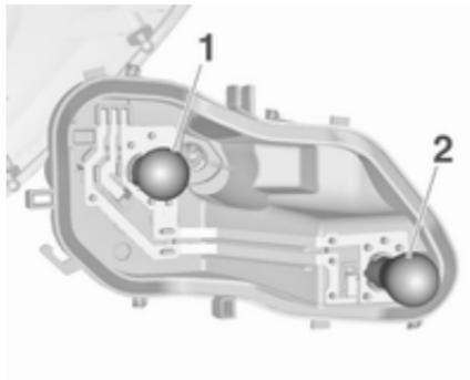
5. Remove the bulb by pushing the bulb slightly into the socket and rotating anticlockwise:
