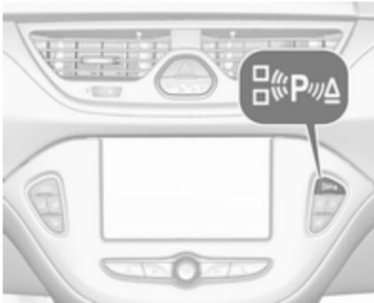
When searching for a parking slot, the system is ready to operate with a long press of **SET/CLR**.
