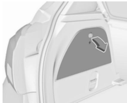
1. Release the cover in the load compartment on the respective side and remove.
