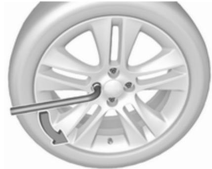
2. Install the wheel wrench ensuring that it locates securely and loosen each wheel bolt by half a turn.
