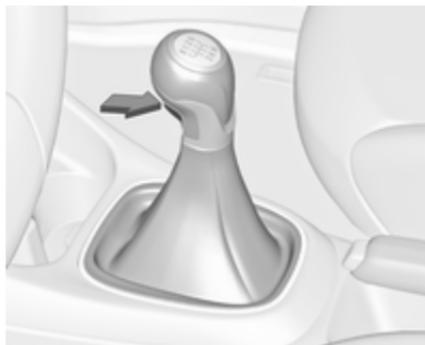
Reverse: with the vehicle stationary, depress clutch pedal and press the release button on the selector lever and engage the gear.
