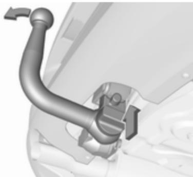
Insert the tensioned coupling ball bar in the opening and push firmly upwards until it audibly engages.
