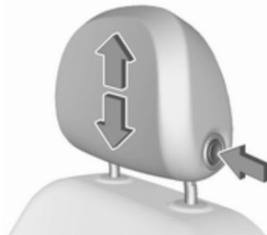
Press release button, adjust height, engage.
