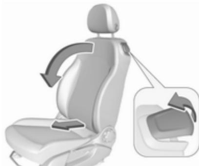
Pull release lever towards the front and fold backrest forwards. Then slide seat forwards to the stop.
