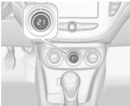
If the minimum temperature **Lo** is set, the climate control system runs at maximum cooling if cooling
