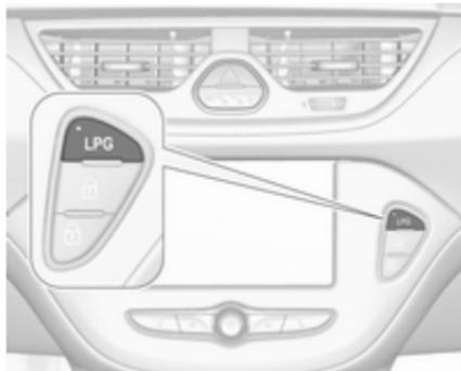
Pressing **LPG** switches between petrol and liquid gas operation as soon as the required parameters (coolant temperature, gas temperature and minimum engine speed) have been reached. The requirements are usually fulfilled after approx. 60 seconds (depending on exterior temperature) and the first firm press on the accelerator. The LED status shows the current operating mode.
