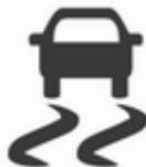
ESC is operational after each engine start as soon as the control indicator extinguishes.
