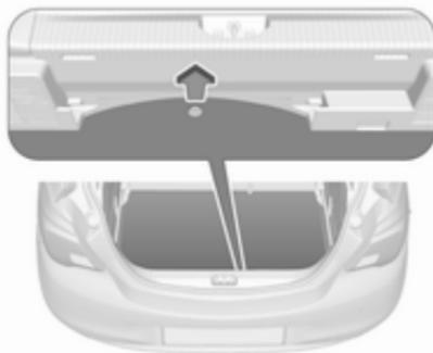
Lift up rear floor cover to gain access to emergency breakdown equipment.
