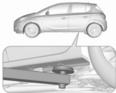
Rear arm position of the lifting platform located centrally under the recess of the sill.
