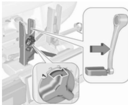
If the bicycle has curved pedal cranks, screw in the pedal crank unit all the way (position 1).
