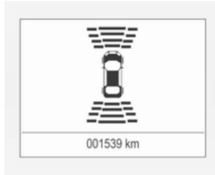
The distance indication can be inhibited by vehicle messages with a higher priority. After dismissing the message, distance indication appears again.
