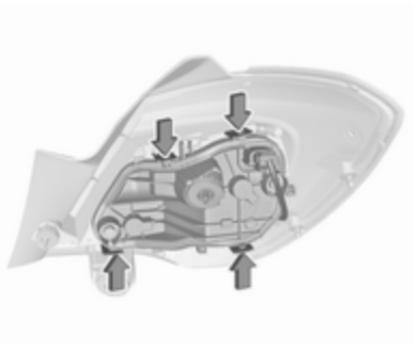
4. Press the retaining lugs and remove the bulb carrier from the light assembly.
