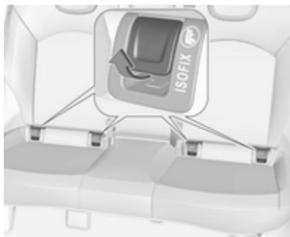
Fasten vehicle-approved ISOFIX child restraint systems to the ISOFIX mounting brackets. Specific vehicle ISOFIX child restraint system positions are marked in the table by IL ⇨ 54.
