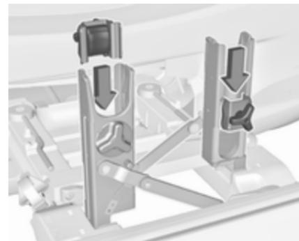
Push the pedal crank mounts into the pedal crank recess as shown in the illustration.
