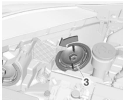
1. Rotate the cap (3) anticlockwise and remove it.
