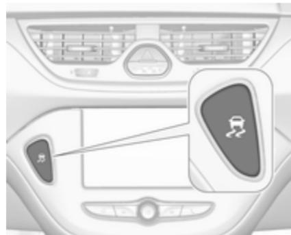
TC can be switched off when spinning of drive wheels is required: press
