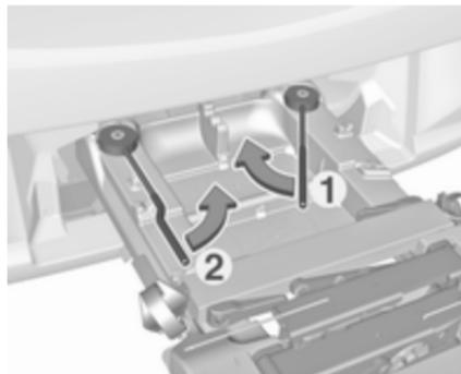
Swivel first the right clamping lever (1) forwards, followed by the left clamping lever (2), until they can be engaged in their respective recesses.
