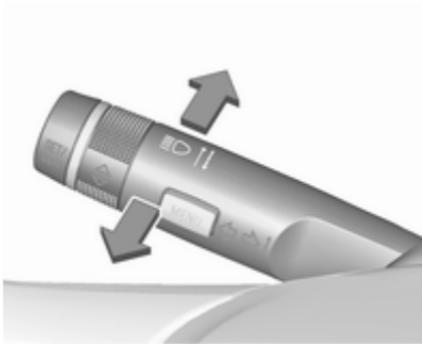
To switch from low to high beam, push stalk.
