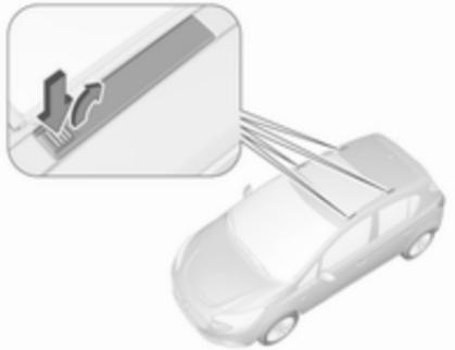
Disengage covers concealing roof rack mounts by pushing sliders in direction of arrow and remove upwards. To close roof rack mounts, first insert covers at front and engage sliders at rear.
