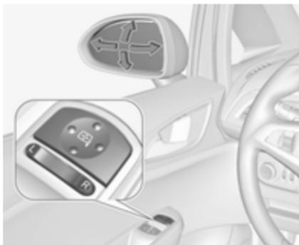
Select the relevant exterior mirror by pressing the rocker switch to the left (**L**) or right (**R**). Then swivel the control
