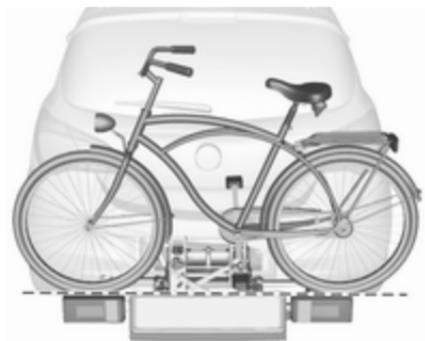
Place the wheel recesses so that the bicycle is roughly horizontal. Here, the distance between the pedals and the tailgate should be at least 5 cm.
