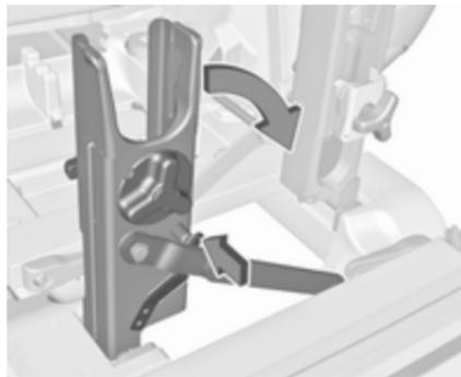
Disengage the locking lever on the diagonal support and fold both pedal crank recesses down.
