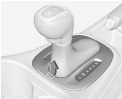
2. Release the selector lever trim from the centre console; Poke with a finger into the leather socket in front of the selector lever and push the trim upwards at the front rim from below, as shown in the illustration. Rotate trim to the left.
