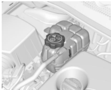
If the cooling system is cold, the coolant level should be above the filling line mark.
