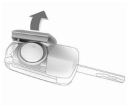
Extend the key and open the unit sideways. Replace the battery (battery type CR 2032), paying attention to the installation position. Close the unit and synchronise.
