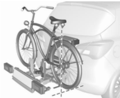
Align the bicycle in the longitudinal direction of the vehicle: Slightly loosen the pedal mount.
