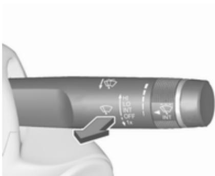
Pull lever. Washer fluid is sprayed onto the windscreen and the wiper wipes a few times.
