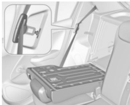
If the vehicle is to be loaded via a rear door, take the seat belt out of the seat backrest guide and insert the latch plate in the recess as shown in the illustration.
