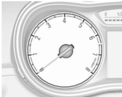
Displays the engine speed.
