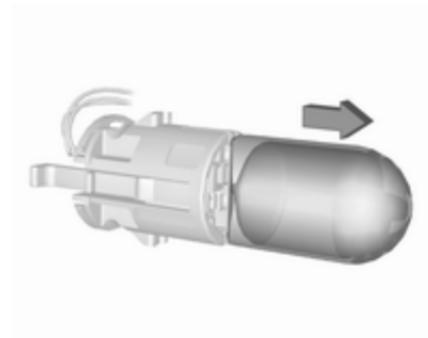
3. Remove the bulb from the socket by pulling.
