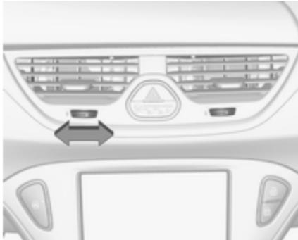
Adjust the air amount at the vent outlet by turning the adjuster wheel. The vent is closed when the adjuster wheel is turned close to the left or right.
