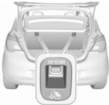
In addition to the ISOFIX mounting brackets, fasten the Top-tether strap to the Top-tether anchors.
