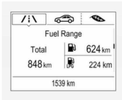
Display of the approximate total fuel range for each fuel tank (LPG and petrol). A low fuel level in either tank is indicated by **Low** in the respective section.
