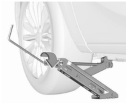
Attach jack handle and with the jack correctly aligned rotate handle until wheel is clear of the ground.
