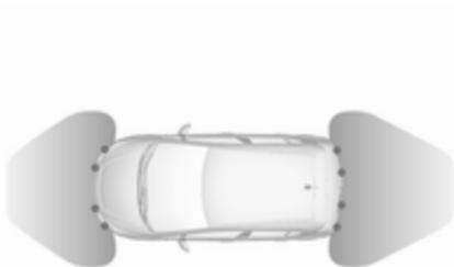
The system has four ultrasonic parking sensors each in the rear and front bumper.
