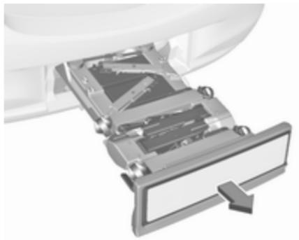
Completely pull out the rear carrier system until you hear it engage. Ensure that it is not possible to push in the rear carrier system without pulling the release lever again.
