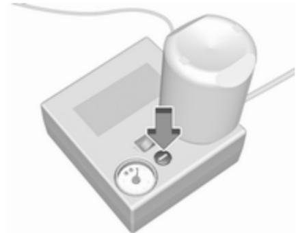
If the prescribed tyre pressure is not obtained within 10 minutes, remove the tyre repair kit. Move the vehicle one tyre rotation. Reattach the tyre repair kit and continue the filling procedure for 10 minutes. If the prescribed tyre pressure is still not obtained, the tyre is too badly damaged. Seek the assistance of a workshop.
