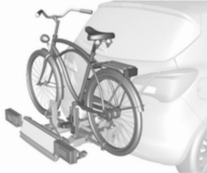
The rear carrier system (Flex-Fix system) allows bicycles to be attached to an extendable carrier integrated into the vehicle floor. The transportation of other objects is not permitted.
