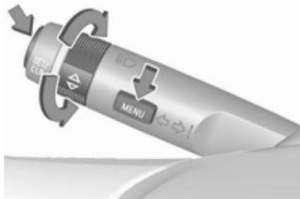
Press **MENU** to switch between the main menus or to return from a submenu to the next higher menu level.
