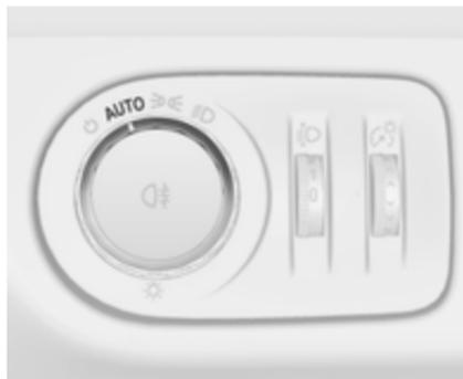
When the automatic light control function is switched on and the engine is running, the system switches between daytime running light and headlights automatically depending on the lighting conditions and information given by the rain sensor system.
