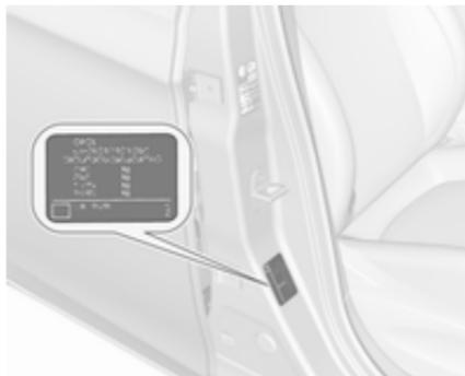
The identification plate is located on the left or right door frame.
