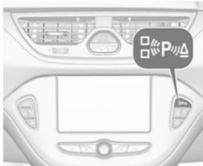
An illuminated LED in the parking assist button
