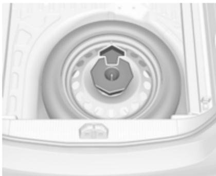
Remove spacer above the spare wheel, lift the wheel, move to a vertical position and remove from above.
