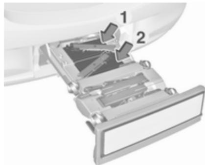
Fold in the lamp supports on the backs of the tail lamps.
