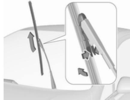
Lift the wiper arm until it stays in the raised position. Press the catches on both sides, tilt wiper blade at a 90° angle to the wiper arm and remove upwards.
