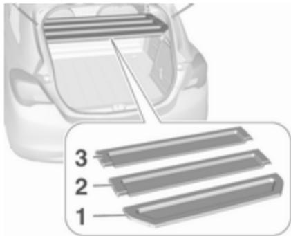
To remove the three other segments (order 1 to 3) lift at the rear, disengage, twist and remove.
