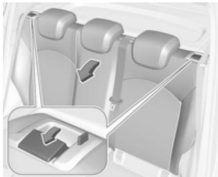
Guide the seat belts through side supports to protect them against damage. When folding the backrest, pull the seat belts along with it.
