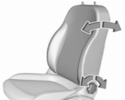
Turn handwheel to adjust inclination.
