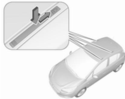
Push covers for concealing roof rack mounts down and push backwards.
