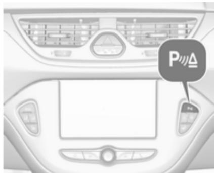
An illuminated LED in the parking assist button **P** with a triangle symbol indicates that the system is ready to operate.
