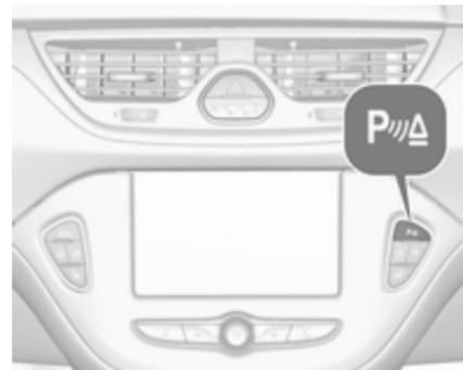
The system automatically switches off when reverse gear is disengaged. Manual deactivation is also possible by pressing the parking assist button **P**
