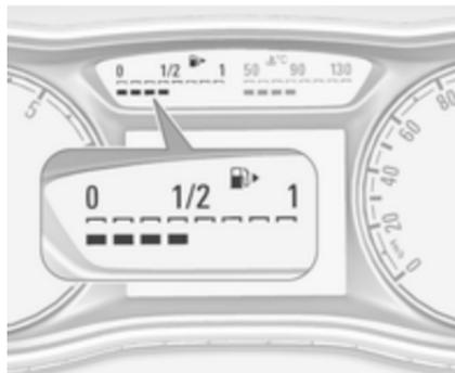
Displays the fuel level or gas content in the tank depending on the operation mode.
