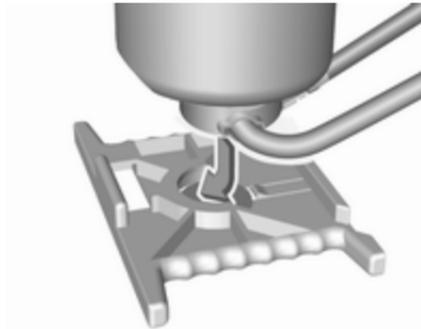
3. Position the sealant bottle on the bracket. Make sure that the bottle does not fall.
