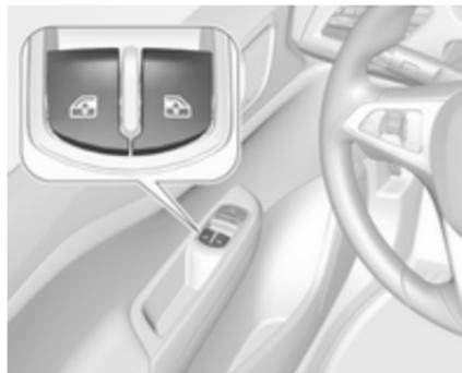
Operate the switch in the door trim for the respective window. Push to open or pull to close.
