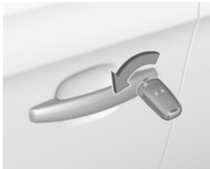
Manually unlock the driver's door by turning the key in the lock. Switch on the ignition and press the central locking button
