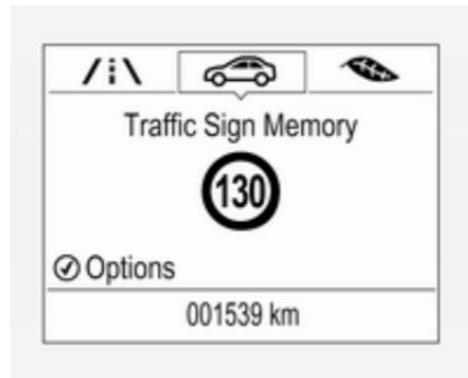
Once activated and when the traffic sign detection page is currently not displayed, newly detected speed limit and no passing signs are displayed as pop-up alerts in the Driver Information Centre.
