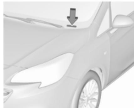
The Vehicle Identification Number may be embossed on the instrument panel, visible through the windscreen, or in the engine compartment on the right body panel.
