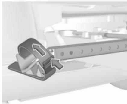
Push the release lever on the strap retainer and remove the strap retainer.
