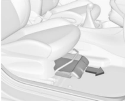
Lift at recessed edge and pull out.
