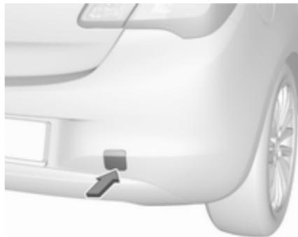
Wrap a cloth around the tip of a flat screwdriver to prevent paint damage. Insert the screwdriver in the slot at the lower part of the cap. Release the cap by carefully moving the screwdriver downwards.
