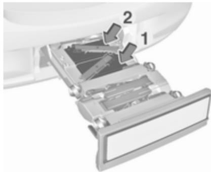
First remove the rear (1), then the front (2) tail lamp from the recesses.
