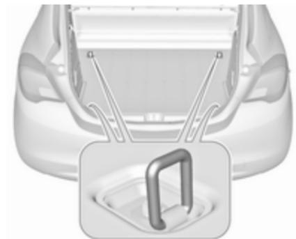
Loads can be secured using four lashing eyes in the load compartment
