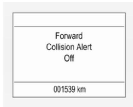
If the forward collision alert was deactivated, alert sensitivity is set to "medium" when ignition is switched on next time.
