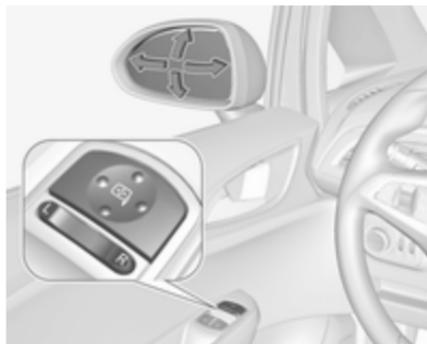
Select the relevant exterior mirror with the rocker switch and adjust the mirror with the control
