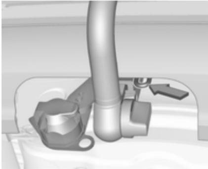
Attach breakaway stopping cable to eye.
