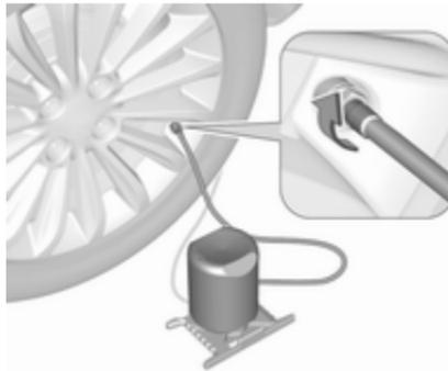
4. Unscrew valve cap from defective tyre.
