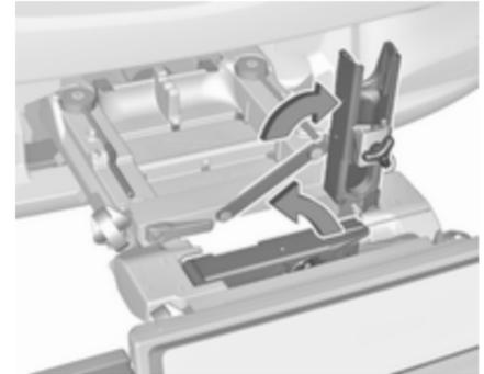
Fold one or both pedal crank recesses upwards until the diagonal support engages.
