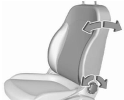
Turn handwheel. Do not lean on backrest while adjusting.
