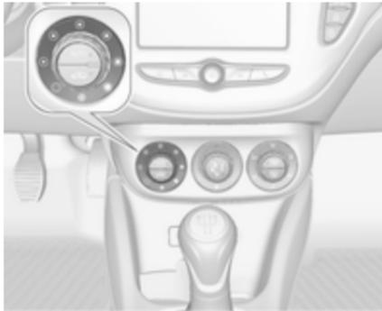
Turn left rotary knob to decrease or increase fan speed. The fan speed is indicated in the Info Display.
