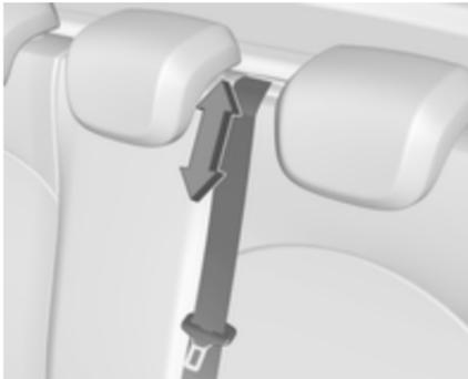
The seat belt of the centre seat could be blocked when the backrest is folded up too quickly. To unlock the retractor, push in the seat belt or pull it out by approx. 20 mm then release.
