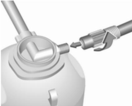
2. Detach air hose from bracket and screw onto sealant bottle connection.
