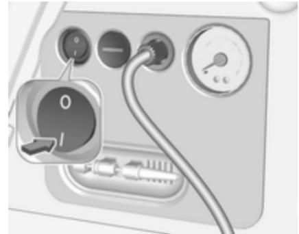
8. Press on/off switch on the compressor. The tyre is filled with sealant.
