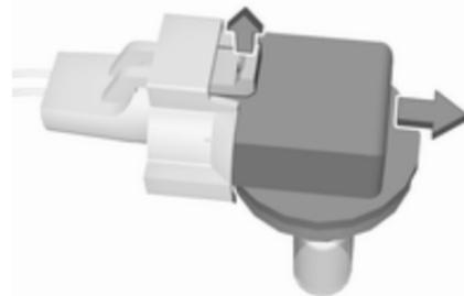
3. Remove the bulb from the plug connector by disengaging and pulling.
