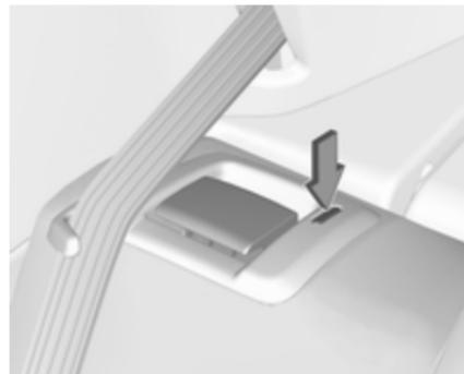
The backrest is properly engaged when the red marks on both sides near the release lever are no longer visible.
