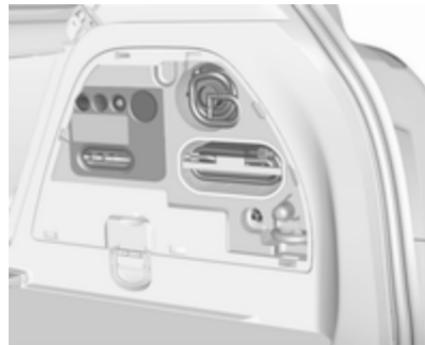
1. Take the sealant bottle and bracket with air hose from the insert.
