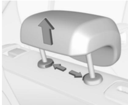
Press both catches, pull the head restraint upwards and remove.
