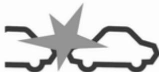
When the time to a potential collision with a vehicle in front gets too small and a collision is imminent, the collision alert symbol pops-up in the Driver Information Centre and the driver gets notified by a flashing red LED stripe which is projected on the windscreen in the driver's field of view.
