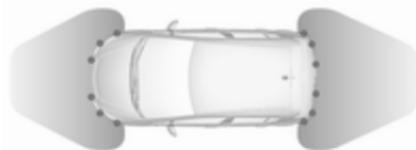
Advanced parking assist is always combined with front-rear parking assist. Both systems use the same sensors in the front and rear bumper.
