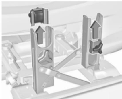
Remove the pedal crank mounts from the pedal crank recesses.
