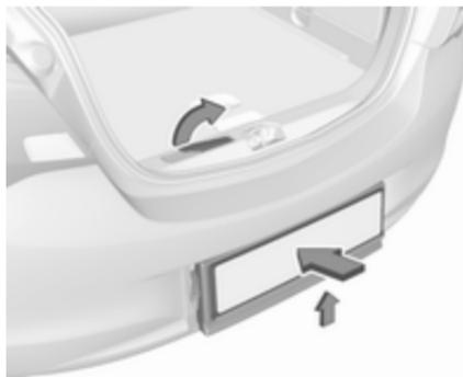
Push the release lever up and hold. Lift the system slightly and push it into the bumper until it engages.
