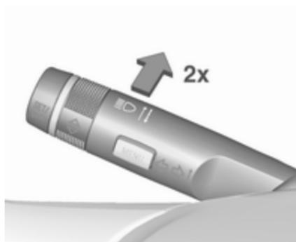
The high beam assist is activated by pushing the stalk twice at a speed above 40 km/h.
