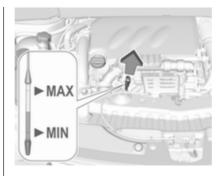
Pull out the dipstick, wipe it clean, reinsert it fully, pull out and read the engine oil level.
