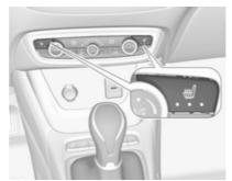
Adjust heating to the desired setting by pressing # for the respective seat one or more times. The control indicator in the button indicates the setting.
