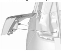
2. Remove the light assembly by pulling it straight back.
