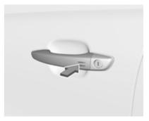
Press with a finger or thumb on one of the door handles (at the markings) or press the tailgate touchpad.
