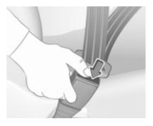
To release belt, press red button on belt buckle.
