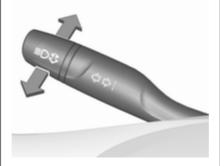
Push lever to switch from low to high beam.
