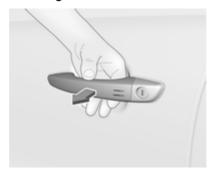
Pass your hand behind any door handle to unlock the vehicle or press the tailgate touchpad.
