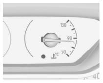
Displays the coolant temperature.
