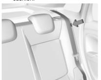
When folding the backrests, insert the seat belts in the guiding latches and pull the seat belts along with them.
