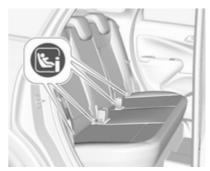
Fasten vehicle-approved ISOFIX child restraint systems to the ISOFIX brackets. Specific vehicle ISOFIX child restraint system positions are marked in the ISOFIX table ♦ 61.
