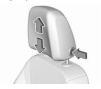
Press release button, adjust height, engage.
