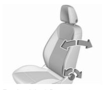
Turn handwheel. Do not lean on backrest when adjusting.
