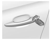
Manually lock the driver's door by inserting and turning the key in the lock cylinder.
