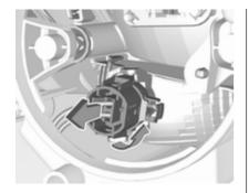
Rotate the lower bulb holder anticlockwise to disengage.
