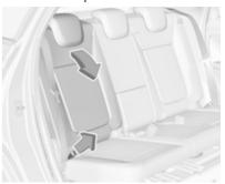
Pull the loop and fold down the backrest onto the seat cushion.
