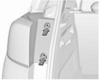
1. Unscrew the two screws that secure the light assembly.
