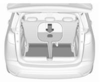
The rear floor cover can be removed. Raise cover at the recess and remove.
