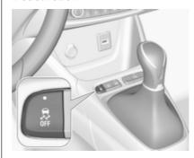
Electronic Stability Control and Traction Control can be deactivated, everytime it is required: press #.
