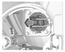
2. Withdraw the upper bulb holder from the reflector housing.
