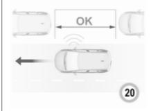
When a free slot is detected, a visual feedback on the Colour-Info-Display and a first acoustic signal is given. Drive slowly forwards. When the second acoustic signal is given, stop the vehicle, select reverse gear, release the steering wheel and start moving without exceeding 7 km/h.
