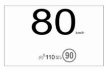
Press **MEM** on the steering wheel to request saving of the suggested speed.
