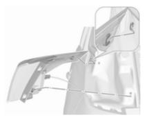
Attach the light assembly to the vehicle body as shown in the illustration and secure with the two screws.
