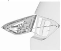
Carefully withdraw the light assembly from the recesses and remove.
