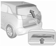
After unlocking, press the touchpad switch above the licence plate and open the tailgate.
