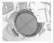
1. Rotate the cap (1) anticlockwise and remove it.
