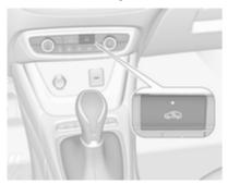
Press \$\sigma\$ to activate air recirculation mode, LED is indicated.
