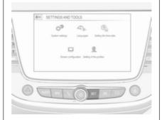
Press **SET** to open settings menu. Use touch buttons to operate the display.
