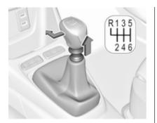
To engage reverse on 6-speed transmission, depress the clutch pedal, pull the ring under the selector lever and move the selector lever to the left and front.
