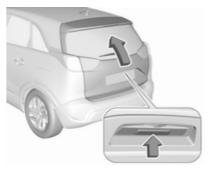
After unlocking, press the touchpad switch above the licence plate and open the tailgate.
