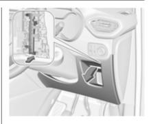
In right-hand drive vehicles, the fuse box is behind a cover in the instrument panel. Disengage cover at the side and remove.
