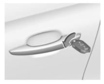
Manually unlock the driver's door by inserting and turning the key in the lock cylinder.
