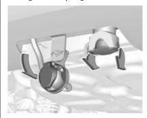
Swivel the connecting socket downwards. Remove the sealing plug from the opening for the coupling ball bar and stow it.
