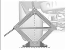
4. Set the jack to the necessary height. Position it directly below
