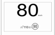
Press **MEM** on the steering wheel to request saving of the suggested speed.
