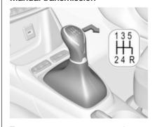
To engage reverse on 5-speed transmission, depress the clutch pedal and then push and move the selector lever to the right and rear.
