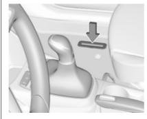
The Vehicle Identification Number may be stamped on the identification plate and on the floor pan, under the floor covering, visible under a cover.
