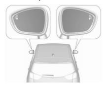
When the system detects a vehicle in the side blind zone while driving forwards, a round LED will illuminate in the relevant exterior mirror.
