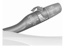
Wiper lever in position **AUTO**. Turn the adjuster wheel to adjust the sensitivity of the rain sensor.
