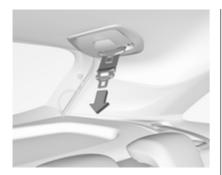
Pull latch plates with the belt out of belt holder in the roof.
