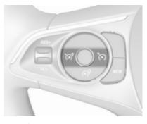
Press © on the steering wheel: symbol © and Pause are indicated in the Driver Information Centre. The system is still not active.
