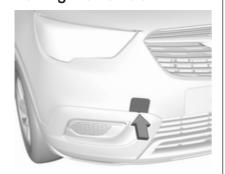
Insert a screwdriver in the slot at the bottom of the cap. Release the cap by carefully moving the screwdriver downwards.
