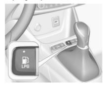
Pressing LPG switches between petrol and liquid gas operation as soon as the required parameters (coolant temperature, gas temperature and minimum engine speed) have been reached. The requirements are usually fulfilled after approximately 60 seconds (depending on exterior temperature) and the first firm press on the accelerator. The status LED shows the current operating mode.
