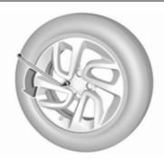
Fold out the wheel wrench and install ensuring that it locates securely and loosen each wheel bolt by half a turn.
