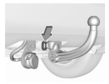
Attach breakaway stopping cable to eye.
