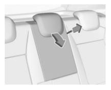
Pull the loop to fold down the rear armrest.
