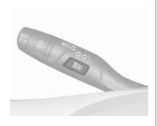
Activate this function pressing a button on the turn and lane change lever. The LED of the button illuminates if the high beam assist is activated. The high beam is switched on automatically at a speed above 25 km/h.
