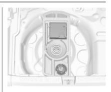
The tyre repair kit is in the load compartment below the floor cover.
