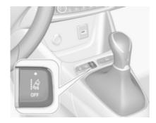
The lane departure warning system is activated by pressing \(\mathbb{g}\). The system is switched on when the LED in the button is not illuminated.
