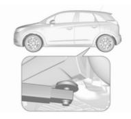
Rear arm position of the lifting platform at the underbody.
