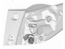
Remove the bulb socket from the light assembly by turning it anticlockwise.
