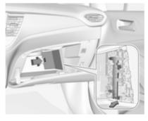
In left-hand drive vehicles, the fuse box is located behind a cover in the glovebox. Open the glovebox and remove the cover. Remove the bracket.
