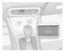
Press A/C to switch on cooling. Activation is indicated by the LED in the button. Cooling is only functional when the engine is running and climate control fan is switched on.
