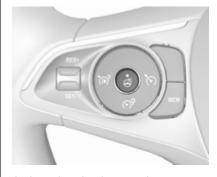
Activate heating by pressing **a**. Activation is indicated by the LED in the button.
