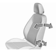
Turn handwheel. Do not lean on backrest when adjusting.
