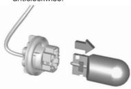
Remove the bulb from the socket by pulling it straight out.
