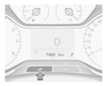
A required service due is displayed in the Driver Information Centre for seven seconds after switching on the ignition.
