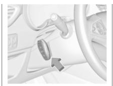
Hold the electronic key with buttons outside at the marking on the steering column cover as shown in the illustration.
