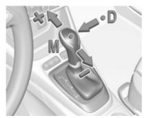
Move selector lever out of position **D** towards the left in position **M**.
