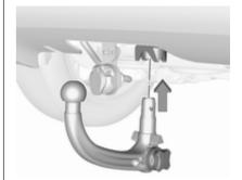
Insert the tensioned coupling ball bar in the opening and push firmly upwards until it audibly engages.
