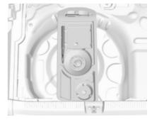
The screwdriver and the towing eye are located in a box below the floor cover in the load compartment.
