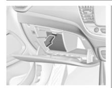
In right-hand drive vehicles, the fuse box is located behind a cover in the glovebox. Open the glovebox and remove the cover.
