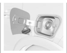
The fuel filler cap can be attached to the hook on the fuel filler flap.
