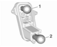
Remove the bulb by pulling and replace.
