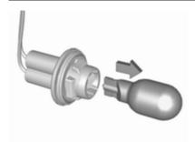
Remove the turn signal light bulb from the socket by pulling it straight out.
