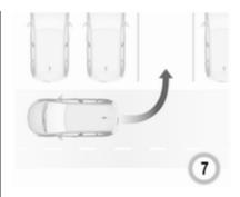
Move forwards and backwards as instructed by observing the warnings of the Parking assist and paying attention to the acoustic signals until the end of manoeuvre is indicated. When finished, Pe extinguishes in the instrument cluster.
