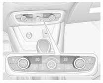
Set the preselected temperatures separately for driver and front passenger to the desired value using the left and right control dials. The dial on the passenger side changes the temperature for the passenger side. The dial on the driver's side changes the temperature for the driver's side or for both sides depending on activation of synchronisation MONO in the climate settings menu. Press MENU to enter the menu.
