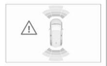
Additionally, the distance to rear and front obstacles is displayed by changing distance lines in the Info-Display ♀ 98.
