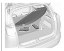
Lift cover, slightly angle and turn it. Remove the cover.
