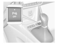
The system is switched off when reverse gear is disengaged. Press P™ OFF to deactivate the system manually. The LED in the button illuminates when the system is deactivated.
