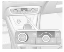
Adjust the air flow by turning rotary knob % to the desired speed. Turn left to decrease or turn right to increase. Fan speed can also be changed by touch buttons in the climate settings display. Press **MENU** to enter the menu.
