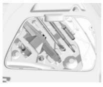
The jack, tools, a strap for securing a damaged wheel and the towing eye are placed in the tool box in the right wall of the load compartment. Spare wheel ♀ 216.
