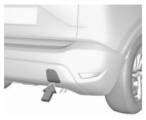
Insert a screwdriver in the slot at the bottom of the cap. Release the cap by carefully moving the screwdriver downwards.
