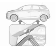
Ensure the jack is correctly positioned under the relevant vehicle jacking point.
