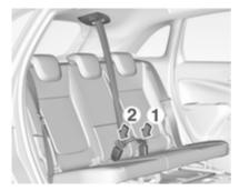
Insert lower latch plate into left-hand buckle (1) at the centre seat. Guide the upper latch plate with the belt over the lap area and the shoulder (do not twist) and insert it into right-hand buckle (2) at centre seat.
