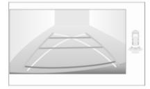
The vertical lines represent the general direction of the vehicle and the distance between the vertical lines corresponds to the width of your vehicle without mirrors. The first horizontal line represents a distance of about 30 cm beyond the edge of vehicle's rear bumper. The upper horizontal lines represent distances of about 1 and 2 metres beyond the
