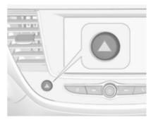
When braking in an emergency, the hazard warning flashers are switched on automatically depending on the force of deceleration. They are switched off automatically the first time you accelerate if you press <u>A</u>.
