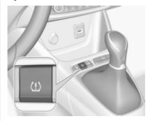
After tyre pressure correction or wheel change, the system must be initialised to learn new circumference reference values:
