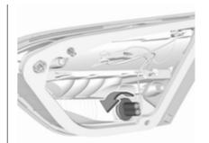
Remove the bulb socket from the light assembly by turning it anticlockwise.
