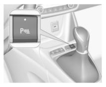
The system is ready to operate when the LED in the parking assist button P<sup>\*</sup> does not illuminate.
