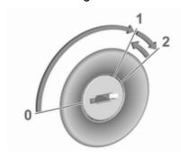
Turn key to position 1 to release the steering wheel lock.
