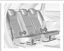
Pull handle, slide seat, release handle and allow seat to engage.
