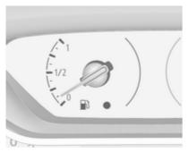
Displays the fuel level in the tank.
