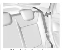
When folding the backrests, insert the seat belts in the guiding latches and pull the seat belts along with them.
