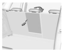
The armrest can also be folded down from the rear by pulling the loop.
