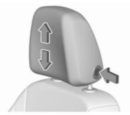
Press release button, adjust height, engage.
