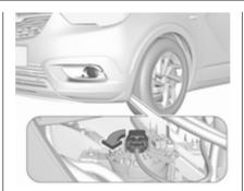
Turn the bulb holder anticlockwise and remove it from the reflector housing.
