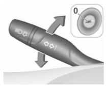
When the vehicle is parked, the parking lights on one side can be activated:
