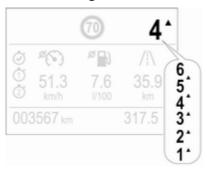
▲ with the number of a higher gear is indicated, when upshifting is recommended for fuel saving reasons.
