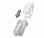
Place the fuse extractor on the various types of fuse from the top or side, and withdraw fuse.
