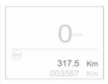
Trip odometer counts up to 9,999 km and then restarts at 0.
