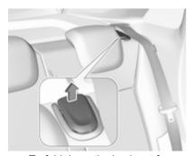
To fold down the backrest from the load compartment, lift the release lever.
