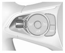
Accelerate to the desired speed and move thumb wheel briefly to **SET/-**. The current speed is stored as maximum speed.
