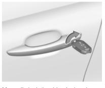
Manually lock the driver's door by inserting and turning the key in the lock cylinder. With working central locking system the vehicle will be locked.
