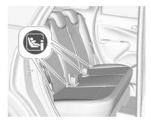
Fasten vehicle-approved ISOFIX child restraint systems to the ISOFIX brackets. Specific vehicle ISOFIX child restraint system positions are marked in the ISOFIX table ♀ 58.
