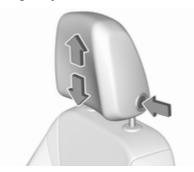
Press release button, adjust height, engage.
