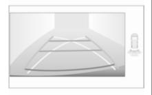
The vertical lines represent the width of the vehicle without mirrors and the general direction of the vehicle. The horizontal lines represent a distance of about 30 cm, 1m and 2 m beyond the rear bumper. The crossing curves represent the maximum turning circle.
