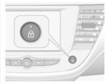
With the ignition on, press \( \text{\pm} \) until an audible signal starts and a corresponding message is displayed.
