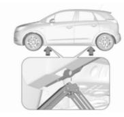
Ensure the jack is correctly positioned under the relevant vehicle jacking point.
