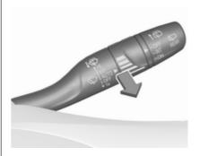
Pull lever. Washer fluid is sprayed onto the windscreen and the wiper wipes a few times.
