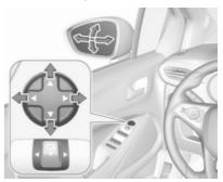
Select the relevant exterior mirror by pushing the mirror button to the left or right.
