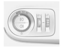
When the automatic light control function is switched on and the engine is running, the system switches between daytime running lights and headlights automatically depending on the external lighting conditions and information given by the wiper system.
