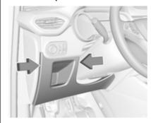
In left-hand drive vehicles, the fuse box is behind a cover in the instrument panel. Disengage cover at the side and remove.
