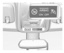
If the control indicator **ON** illuminates for approx. 60 seconds after the ignition is switched on, the front passenger airbag system will inflate in the event of a collision.
