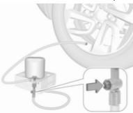
Drain excess tyre pressure with the button on the air hose.
