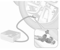
16. Continue driving immediately so that sealant is evenly distributed in the tyre. After driving approx. 5 km (but no more than 10 min), stop and check tyre pressure. Screw compressor air hose directly onto tyre valve when doing this. Fill tyre as described
