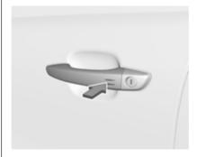
Electronic key system: Unlocking the vehicle by pressing marking on one of the front door handles deactivates the anti-theft alarm system.
