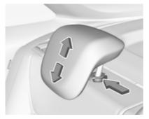
Pull the head restraint upwards or press the catch to release and push the head restraint downwards.
