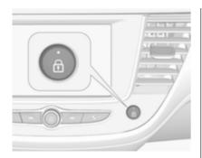
Press  $frac{a}{2}$  to lock. The LED in the button illuminates.
