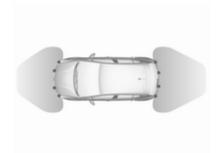
The system operates with ultrasonic parking sensors in the rear and front bumper.
