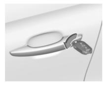
Manually unlock the driver's door by inserting and turning the key in the lock cylinder. With working central locking system the vehicle will be unlocked.
