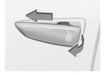
1. Slide the lamp housing forward and remove it at the back.
