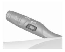
Activate high beam assist by pressing ©. The LED of the button illuminates.
