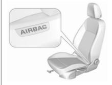
The side airbag system consists of an airbag in each front seat backrest. This can be identified by the word AIRBAG.
