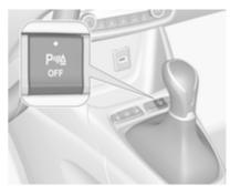
The system is deactivated automatically when vehicle speed exceeds 10 km/h or if the vehicle stops for more than 3 seconds in a forward gear or if no further obstacles are detected.
