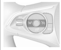
Press (5) on the steering wheel: symbol (5) and a message are indicated in the Driver Information Centre. The system is still not active.
