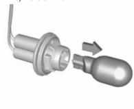
Pull straight out to remove from the socket and replace.
