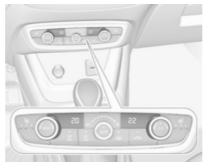
Set the preselected temperatures separately for driver and front passenger to the desired value using the left and right controls. The dial on the passenger side changes the temperature for the passenger side. The dial on the driver's side changes the temperature for the driver's side or for both sides depending on activation of synchronisation MONO in the climate settings menu. Press MENU to enter the menu.
