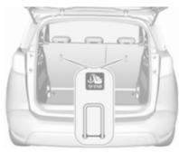
In addition to the ISOFIX brackets, fasten the Top-tether strap to the Top-tether anchors.
