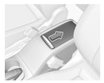
Depending on the version, the storage compartment is located under a cover.
