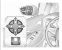
Select the relevant exterior mirror by pushing the mirror button to the left or right. Adjust respective mirror by the four-way control.
