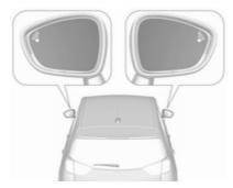
When the system detects a vehicle in the side blind zone while driving forwards, an LED will illuminate in the relevant exterior mirror.
