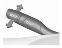
Push to switch from low to high beam.
