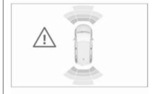
Additionally, the distance to rear and front obstacles is displayed by changing distance lines in the Info Display ♀ 90.
