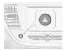
Hazard warning flashers are switched on automatically in the following situations:
