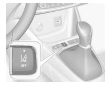
The lane departure warning system is activated by pressing \( \mathbb{G} \). The system is switched on when the LED in the button is not illuminated.
