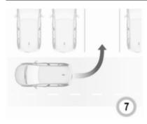
Move forwards and backwards as instructed by observing the warnings of the parking assist and paying attention to the acoustic signals until the end of manoeuvre is indicated. When finished, Po extinguishes in the instrument cluster.
