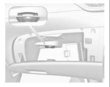
The air vent can be opened or closed by turning.
