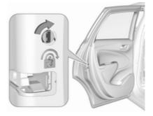
Turn the red child lock in the rear doors to the horizontal position by using a key. The door cannot be opened from the inside.
