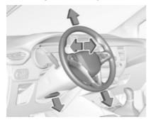
Unlock lever, adjust steering wheel, then engage lever and ensure it is fully locked.
