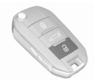
Press to unlock the vehicle. Open the doors by pulling the handles.
