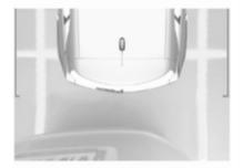
The camera records the vehicle's surroundings during the manoeuvre in order to reconstruct a view from above the rear of the vehicle in its near surroundings, allowing the vehicle to be manoeuvred around obstacles nearby. This view is available with auto mode or in the view selection menu.
