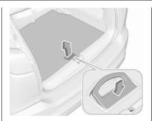
To remove, press the handle to unlock the load floor and lift it up while using the handle.
