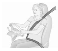
The seat belts are locked during heavy acceleration or deceleration of the vehicle, holding the occupants in the seat position. Therefore the risk of injury is considerably reduced.
