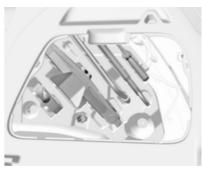
The jack, tools, a strap for securing a damaged wheel and the towing eye are placed in the tool box in the right wall of the load compartment.
