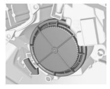
Rotate the cap anticlockwise and remove it.
