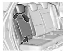
Pull the loop, adjust inclination and release loop. Do not lean on backrest when adjusting.
