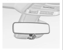
To reduce dazzle, adjust the lever on the underside of the mirror housing.
