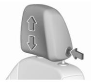
Press release button, adjust height, engage.
