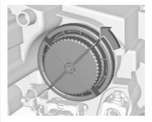
Rotate the cap anticlockwise and remove it.
