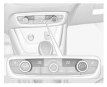
Press **A/C** to switch on cooling. The LED in the button illuminates to indicate activation. Cooling is only functional when the engine is running and climate control fan is switched on. Press **A/C** again to switch off cooling.
