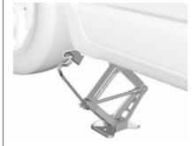
Attach wheel wrench and with the jack correctly aligned rotate wheel wrench until wheel is clear of the ground.
