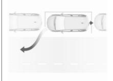
Move forwards and backwards while observing the warnings of the parking assist until the end of manoeuvre is indicated. The manoeuvre is complete when the vehicle's front wheels are out of the parking slot and  $P_{\Theta}$  extinguishes in the instrument cluster.
