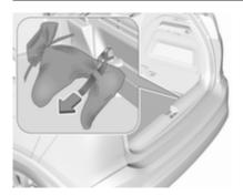
Place the strap through the rear right lashing eye, wrap around twice and tighten the strap to secure the bag.
