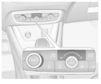
Adjust the air flow by turning rotary knob % to the desired speed.
