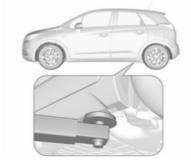
Rear arm position of the lifting platform centrically under the relevant vehicle jacking point.
