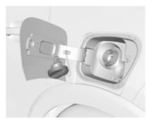
The fuel filler cap can be attached to the hook on the fuel filler flap.
