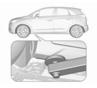
Front arm position of the lifting platform centrically under the relevant vehicle jacking point.
