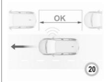
When a free slot is detected, a visual feedback on the Colour Info Display and a first acoustic signal is given. Drive slowly forwards. When the second acoustic signal is given, stop the vehicle, select reverse gear, release the steering wheel and start moving without exceeding 7 km/h.
