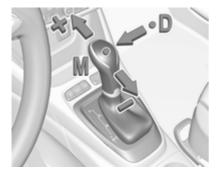
Move selector lever out of position  ${\bf D}$  towards the left in position  ${\bf M}$ .
