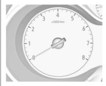
Displays the engine speed.
