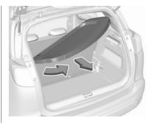
Lift cover, slightly angle and turn it. Remove the cover.
