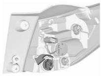
Remove from the light assembly by turning it anticlockwise.
