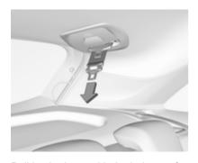
Pull latch plates with the belt out of belt holder in the roof.
