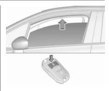
Press and hold  $\widehat{\ }$  to close windows. Release button to stop window movement.
