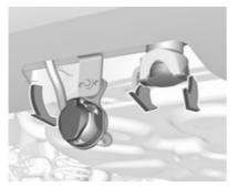
Swivel the connecting socket downwards. Remove the sealing plug from the opening for the coupling ball bar and stow it.
