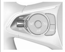
Accelerate to the desired speed and move thumb wheel briefly to **SET/-**. The current speed is stored and maintained. Accelerator pedal can be released.
