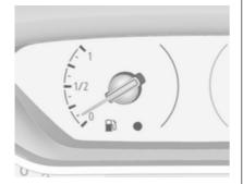
Displays the fuel level in the tank.
