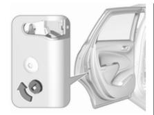
To lock the other doors, first remove the black cover by inserting a key and turning clockwise.
