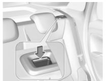
The backrests are properly engaged when the red mark near the lever is no longer visible.
