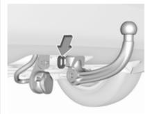
Attach breakaway stopping cable to eye.
