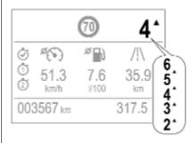
▲ with the number of a higher gear is indicated, when upshifting into this gear is recommended for fuel saving reasons.
