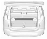
Stow the warning triangle in the space at the rear of the load compartment and secure it with the Velcro® fastener.
