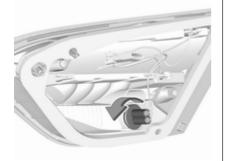
Remove the reverse light bulb socket from the light assembly by turning it anticlockwise.
