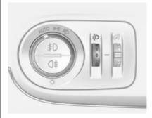
To adapt headlight range to the vehicle load to prevent dazzling: turn thumb wheel position.
