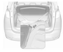
The load compartment cover can be stored behind the rear seat backrests.
