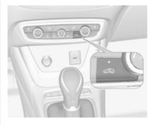
Press to activate the air recirculation mode. The LED in the button illuminates to indicate activation.
