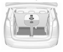
Raise cover at the recess to gain access to emergency breakdown equipment.
