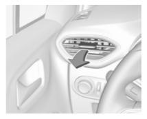
Direct the flow of air by tilting and swivelling the slats.
