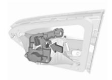
Press latch to release and remove bulb socket.
