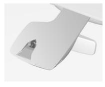
Do not attach stickers such as toll road stickers or similar on the windscreen in the area of the interior mirror. Keep the sensor free from dust, dirt and ice. Otherwise the detection zone of the rain sensor / light sensor and the view area of the camera in the mirror housing could be restricted.
