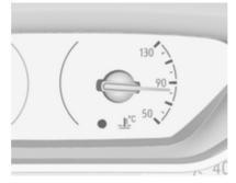
Displays the coolant temperature.
