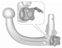
Unlock coupling ball bar by turning key to position .
