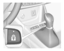
Remotely operated system to prevent opening of the rear doors using the interior handles.
