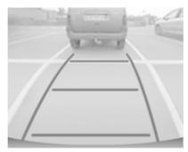
The area behind the vehicle is displayed in the screen. The vertical lines represent the width of the vehicle with mirrors unfolded. The direction of the lines changes with the steering angle.
