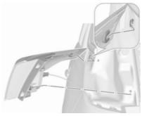
Attach the light assembly to the vehicle body and secure with the two screws. Light assembly in the tailgate
