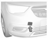
Wrap a cloth around the tip of a flat screwdriver to prevent paint damage. Insert a screwdriver in the slot at the bottom of the cap. Release the cap by carefully moving the screwdriver downwards
