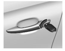
Turn key in the driver's door lock cylinder.
