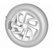
Fold out the wheel wrench and install ensuring that it locates securely and loosen each wheel bolt by half a turn.
