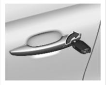
Turn key in the driver's door lock cylinder.
