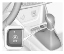
Deactivate the stop-start system manually by pressing a. The deactivation is indicated when the LED in the button illuminates.
