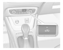
Press so to activate air recirculation mode. LED is indicated.
