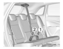
Insert lower latch plate into left-hand buckle (1) at the centre seat. Guide the upper latch plate with the belt over the lap area and the shoulder (do not twist) and insert it into right-hand buckle (2) at centre seat.
