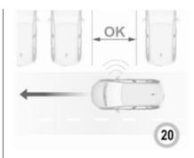
When a free slot is detected, a visual feedback on the Colour Info Display and an acoustic signal is given. Stop the vehicle, select reverse gear, release the steering wheel and start moving without exceeding 7 km/h.
