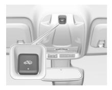
Switch off the monitoring of passenger compartment and vehicle inclination when animals are being left in the vehicle, because of high volume ultrasonic signals and because movements could trigger the alarm. Also switch off when the vehicle is on a ferry or train.
