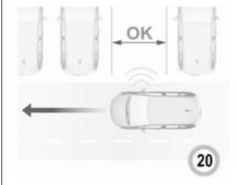
When a free slot is detected, a visual feedback on the Info Display and an acoustic signal is given. Stop the vehicle, select reverse gear, release the steering wheel and start moving without exceeding 7 km/h.
