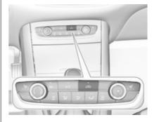
Press So to activate air recirculation mode. The LED in the button illuminates to indicate activation.
