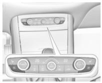
Activate ventilation by pressing  $\overset{\mbox{\ensuremath{\mathbb Z}}}{=} for$  the respective front seat.
