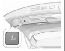
Press button  $\mathfrak{Z}_{\mu}$  in the open tailgate, the whole vehicle will be locked after hands-free closing of the tailgate.
