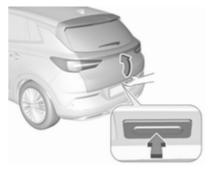
To open the tailgate, press the tailgate button until the tailgate starts to move. If the vehicle is locked, the electronic key must be outside the vehicle, within a range of approx. 1 m of the tailgate.
