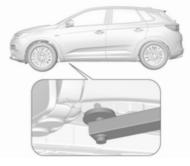
Front arm position of the lifting platform centrically under the relevant vehicle jacking point.
