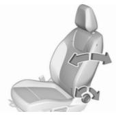
Turn handwheel. Do not lean on backrest when adjusting.
