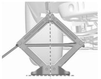
4. Set the jack to the necessary height. Position it directly below the jacking point in a manner that prevents it from slipping.
