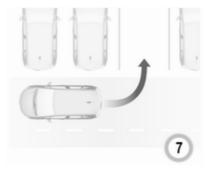
Move forwards and backwards as instructed by observing the warnings of the parking assist and paying attention to the acoustic signals until the end of manoeuvre is indicated. When finished,  $P_{\Theta}$  extinguishes in the instrument cluster.
