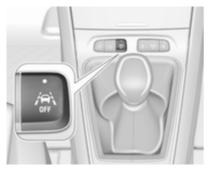
If the system is activated, the LED in the button # is not illuminated. To activate the system when the system is deactivated, press #. The system is operational at vehicle speeds between 65 km/h and 180 km/h and if lane markings are detectable. The driver must hold the steering wheel with both hands. The Electronic Stability Control system must be activated.
