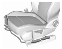
Pull handle, slide seat, release handle. Try to move the seat back and forth to ensure that the seat is locked in place.
