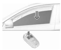
Press and hold <sup>®</sup> to close windows. Release button to stop window movement.
