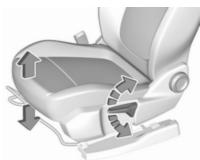
Lever pumping motion up : seat higher down : seat lower Seat position ▷ 46.
