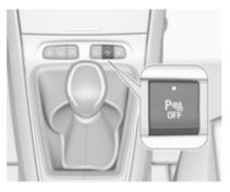
The system is ready to operate when the LED in the parking assist button <sup>™</sup> is not illuminated.
