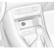
A 12 V power outlet is located behind the storage cover. Press cover to open.
