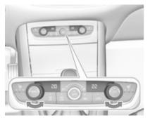
Set the preselected temperatures separately for the driver and the front passenger to the desired value using the left and right rotary ring. The rotary ring on the passenger side changes the temperature of the passenger side. The rotary ring on the driver's side changes the temperature of the driver's side or of both sides, depending on activation of synchronisation **MONO** in the climate settings menu. Press **MENU** to enter the menu.
