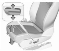
Move switch upwards / downwards.
