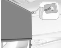
• There are installation openings on both sides in the roof frame above the front seats: suspend and engage rod of net at one side, compress rod and suspend and engage at the other side.
