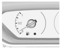
Displays the level in the fuel tank.
