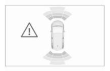
Additionally, the distance to rear and front obstacles is displayed by changing distance lines in the Info Display  $\diamondsuit$  103.
