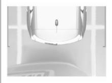
The camera records the vehicle's surroundings during the manoeuvre in order to reconstruct a view from above the rear or the front of the vehicle in its near surroundings.Thus, the vehicle can be manoeuvred around obstacles nearby. This view is available with auto mode or in the view selection menu.
