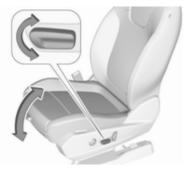
Move front of switch upwards / downwards.
