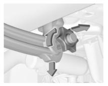
Open the protective flap and turn the key to position to unlock the coupling ball bar.
