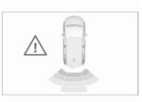
Additionally, the distance to rear obstacles is displayed by changing distance lines in the Info Display ⇔ 103. When the obstacle is very close,  $\triangle$  for danger is displayed.
