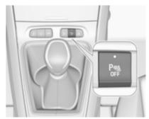
The system is switched off when reverse gear is disengaged. Press <sup>the</sup> to deactivate the system manually. The LED in the button illuminates when the system is deactivated. If the system has been deactivated manually, it is not reactivated automatically the next time the ignition is switched on.
