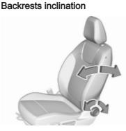
Turn handwheel. Do not lean on backrest when adjusting. Seat position  $\diamondsuit$  46. Manual seat adjustment  $\diamondsuit$  47.
