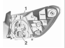
7. Detach the bulb from the bulb socket and replace the bulb.
