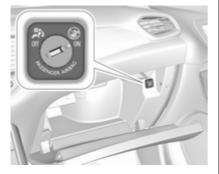
The front passenger airbag system can be deactivated via a keyoperated switch in the glovebox. Use the ignition key to choose the position:
