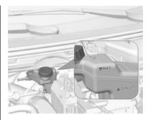
The brake fluid level must be between the **DANGER** and **MAX** marks.
