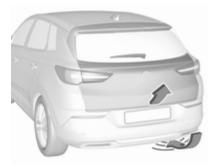
To open or close the tailgate move the foot below the rear bumper back and forth in the area below the number plate. The key must be within a range of 1 m. Do not hold the foot longer or move too slow below the bumper. The electronic key must be outside the vehicle, within a range of approx. 1 m of the tailgate.
