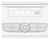
Press **MENU** to open the menu page. Use four-way button to operate the display: Select <sup></sup>H<sup>®</sup> **Personalisation**configuration, **→** OK.
