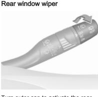
Turn outer cap to activate the rear window wiper:
