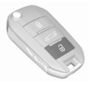
Press 🕆 to unlock the vehicle. Open the doors by pulling the handles. Press 🖘 to unlock the tailgate only. Tailgate
