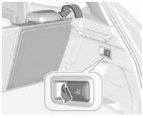
Alternatively fold seat backrests from the load compartment: pull switch on left or right sidewall of the load compartment to fold the corresponding part of the rear seat backrest.
