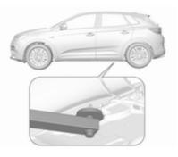
Rear arm position of the lifting platform centrically under the relevant vehicle jacking point.
