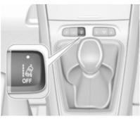
After ignition is switched on, the lane departure warning system is activated. If the system is activated, the LED in the button ﷺ is not
