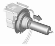
3. Detach the bulb from the bulb socket and replace the bulb.
