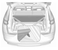
To hold the load compartment cover in an upright positon, lift it up past the retractable stops.
