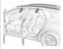
Fasten the roof rack in the roof railing above the mounting points located in each door frame of the vehicle body.
