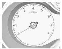
Displays the engine speed.
