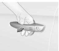
Pass a hand behind the door handle of one of the front doors to unlock the vehicle or press the tailgate button.
