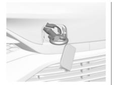
Screw in the towing eye as far as it will go until it stops in a horizontal position.
