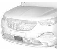
The radar unit is located in the middle of the front bumper.
