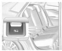
Fasten vehicle-approved ISOFIX child restraint systems to the ISOFIX mounting brackets. Specific vehicle ISOFIX child restraint system positions are marked in the ISOFIX table \$ 65.
