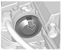
1. Remove the protective cover by pulling the tab.
