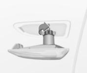
2. Turn bulb socket clockwise and remove from housing.
