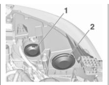
High beam (1) inner bulb. Low beam (2) outer bulb.
