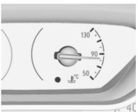
Displays the coolant temperature.
