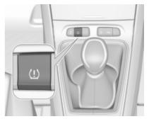
After tyre pressure correction or wheel change, the system must be initialised to learn new circumference reference values:
