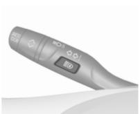
Activate the high beam assist by pressing ≣Ø. The LED of the button illuminates if the high beam assist is activated. High beam is switched on automatically at a speed above 25 km/h. High beam is switched off at a speed below 15 km/h, but high beam assist remains active.
