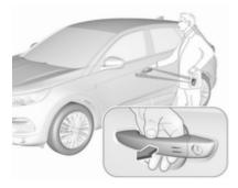
The electronic key must be outside the vehicle, within a range of approx. one metre of the relevant door side.
