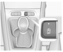
Deactivate the stop-start system manually by pressing <sup>(a)</sup>. The deactivation is indicated when the LED in the button illuminates.
