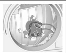
2. Press retaining clip upwards and pull the bulb socket toward the rear.
