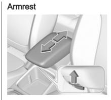
The armrest can be slid forwards by 10 cm. Pull the handle to slide the armrest. Under the armrest there is a storage compartment.
