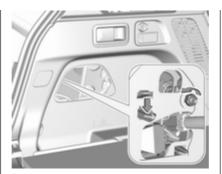
2. Slacken the lamp fixing nut using a box spanner or socket.
