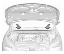
The air intake in front of the windscreen in the engine compartment must be kept clear to allow air intake. Remove any leaves, dirt or snow.
