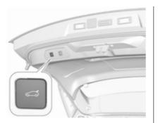
To close, press  $\iff$  in the open tailgate until the tailgate starts to move.
