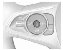
Activate heating by pressing **\***. Activation is indicated by the LED in the button.
