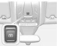
Press a gently to the first detent at the rear: the sunblind is opened as long as the switch is operated.
