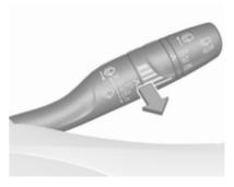
Pull lever. Washer fluid is sprayed onto the windscreen and the wiper wipes a few times. Washer fluid ⇔ 207.
