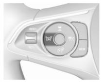
Press (b), the adaptive cruise control is in pause mode and a message is displayed. The vehicle is driven without adaptive cruise control.
