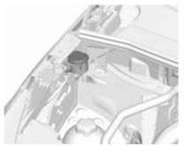
Fill with clean water mixed with a suitable quantity of approved windscreen washer fluid which contains antifreeze.
