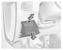
In left-hand drive vehicles, the fuse box is behind a cover in the instrument panel at the left side. Open the cover and remove it by pressing the lock.
