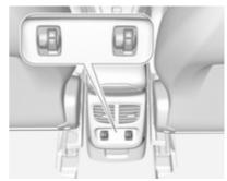
Adjust seat heating by turning thumb wheel # for the respective rear outer seat to the desired setting.
