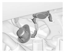
Disengage and fold down the socket. Remove the sealing plug from the opening for the coupling ball bar and stow it.
