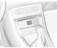
A USB port is located behind the storage cover. Press cover to open.
