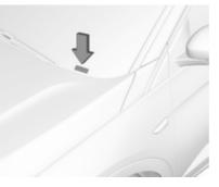
The Vehicle Identification Number may be embossed on the instrument panel, visible through the windscreen, or in the engine compartment on the right body panel.
