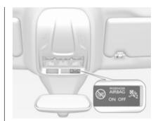
If the control indicator  $\circledast$  illuminates for approx. 60 seconds after the ignition is switched on, the front passenger airbag system will inflate in the event of a collision.
