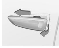
1. Slide lamp to its left side and remove with its right end.
