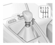
To engage reverse on 6-speed transmission, depress the clutch pedal, pull the ring under the selector lever and move the selector lever quite to the left and front.
