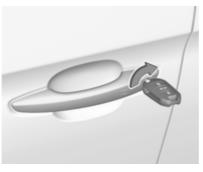
Manually lock the driver's door by inserting and turning the key in the lock cylinder.
