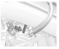
Attach breakaway stopping cable to eye.
