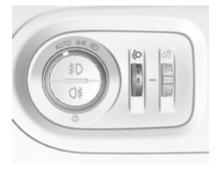
To adapt headlight range to the vehicle load to prevent dazzling, turn thumb wheel <sup>€D</sup> to required position.
