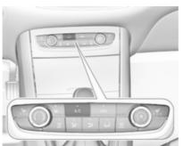
Press **A/C** to switch on cooling. The LED in the button illuminates to indicate activation. Cooling is only functional when the engine is running and fan is switched on.
