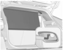
There are installation openings on both sides in the roof frame above the rear seats: suspend and engage rod of net at one side, compress rod and suspend and engage at the other side.
