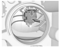
2. Press retaining clip downwards and pull the bulb socket toward the rear.
