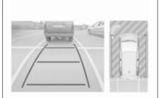
The screen in the Info Display is divided into two parts. On the right there is a view from above the vehicle and on the left there is the view from the rear or the front displayed. The parking sensors complete the information on the view from above the vehicle.
