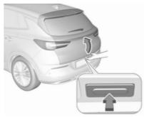
After unlocking, press the tailgate button and open the tailgate. Radio remote control  $\diamondsuit$  22. Central locking system  $\diamondsuit$  24. Electronic key system  $\diamondsuit$  23. Load compartment  $\diamondsuit$  30.
