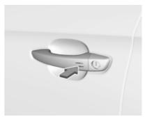
Press with a finger or thumb on one of the door handles (at the markings) or press the tailgate button.
