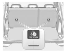
In addition to the ISOFIX mounting brackets, fasten the Top-tether strap to the Top-tether anchors.
