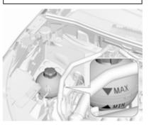
If the cooling system is cold, the coolant level should be above the **MIN** mark. Top up if the level is low.
