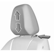
Press release button, adjust height, engage.
