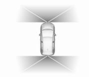
The 180° view facilitates reversing out of a parking bay, making it possible to see the approach of vehicles, pedestrians and cyclists. This view is not recommended for carrying out a complete manoeuvre. It is made up of three areas: left 1, centre 2 and right 3. This view is available from the view selection menu only.
