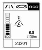
Shift indication: Current gear is indicated inside an arrow. The figure above recommends upshifting for fuel saving reasons.
