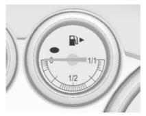
Displays the fuel level or gas level in the tank depending on the operation mode.
