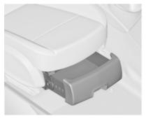
Press button in the recess and pull out drawer. Maximum load: 3 kg. To close, push in and engage.
