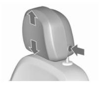
Press release button, adjust height, engage.
