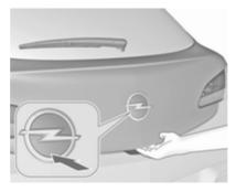
Press on radio remote control or push the brand emblem at the bottom half to unlock and open the tailgate.
