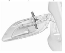
Disengage the bulb socket from the reflector housing by pressing both retaining lugs.
