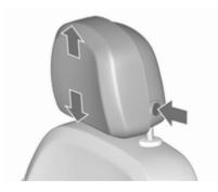
**Height adjustment**Press release button, adjust height, engage.
