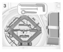
The jack and the tools are in the tool box below the spare wheel in the load compartment. The wheel wrench, the towing eye and an extension bolt for securing a damaged wheel (only vehicles with temporary spare wheel) are in the tool bag located in the spare wheel well near the tool box. Spare wheel ▷ 242
