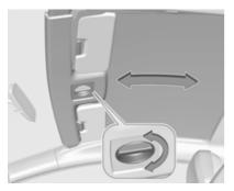
Turn the handle and move the roof cover to a suitable position.
