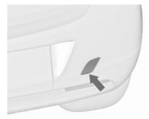
Insert a screwdriver in the slot at the lower bend of the cap. Release the cap by carefully moving the screwdriver downwards.
