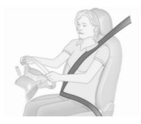
Pull out the seat belt and fasten in belt buckle. The seat belt must not be twisted and must fit close against the body. The backrest must not be tilted back too far (maximum approx. 25°). To unfasten belt, press red button on belt buckle.
