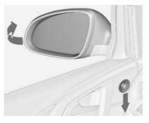
Turn control to 0, then push the control down. Both exterior mirrors will fold.
