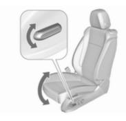
Move front of switch upwards/downwards.
