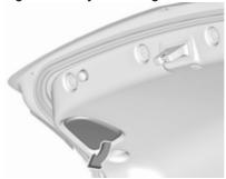
1. Open the tailgate and remove the cover on the respective side.
