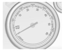
Displays the engine speed.
