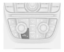
Press So to activate the air recirculation mode. The LED in the button illuminates to indicate activation.
