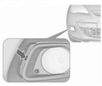
Disengage the cover with a screwdriver in the recess and remove the cover.
