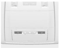
Operated by pressing  $\stackrel{\wedge}{\simeq}$  and  $\stackrel{\partial}{\simeq}$  in front and rear courtesy lights.
