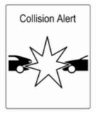
If a vehicle directly ahead is approached too quickly, a warning chime and alert in the Driver Information Centre is provided.
