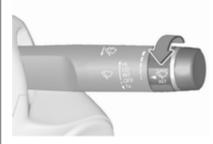
Turn the adjuster wheel to adjust the sensitivity:
