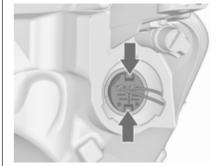
Press latches together and withdraw the bulb holder from the reflector.
