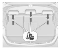
On hatchback version, anchors are on the backside of the rear seats.
