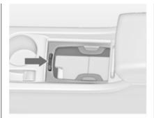
Press button to remove the frame of the cupholder. The frame can be stowed in the glovebox.
