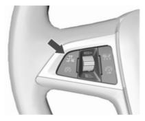
Press %; the current setting is shown in the Driver Information Centre. Press % again to change the following distance. The setting is also displayed in the top line of the Driver Information Centre.
