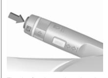
The alert function can be activated or deactivated in the Settings menu of the traffic sign assistant page by pressing **SET/CLR** on the turn signal lever.
