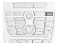
When searching for a parking slot, the system must be activated by pressing for approx. one second.
