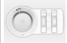
When the automatic light control function is switched on and the engine is running, the system switches between daytime running light and headlights automatically
