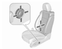
Adjust lumbar support using the four-way switch to suit personal requirements.
