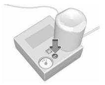
If the prescribed tyre pressure is not obtained within ten minutes, remove the tyre repair kit. Move the vehicle one tyre rotation. Reattach the tyre repair kit and continue the filling procedure for ten minutes. If the prescribed tyre pressure is still not obtained, the tyre is too badly damaged. Seek the assistance of a workshop.
