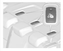
On Notchback version, open the flap of the required fastening eye on the placement area behind the head restraints, marked by the child seat symbol.
