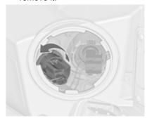
Rotate bulb socket anticlockwise to disengage and withdraw from the reflector housing.
