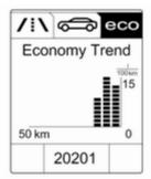
Economy Trend: Displays the average consumption development over a distance of 50 km. Filled segments display the consumption in 5 km steps and shows the effect of topography or driving behaviour on fuel consumption.
