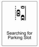
When the vehicle passes a row of cars and the system is activated, the advanced parking assist system begins searching for a suitable parking slot. When a suitable slot is detected, visual feedback in the Driver Information Centre and an acoustic signal are given.
