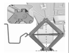
Set the jack to the necessary height. Position it directly below the jacking point in a manner that prevents it from slipping.
