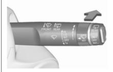
Push lever. Washer fluid is sprayed onto the rear window and the wiper wipes a few times.
