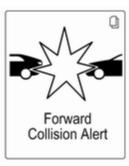
A green illuminated vehicle ahead control indicator illuminates in the instrument cluster when the system has detected a vehicle in the driving path. When the distance to a preceding moving vehicle gets too small or when approaching another vehicle too rapidly and a collision is imminent, the collision alert symbol pops-up in the Driver Information Centre. Simultaneously a warning chime sounds.
