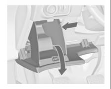
In left-hand drive vehicles, the fuse box is behind the storage compartment in the instrument panel. Open the compartment and push it to the left to unlock. Fold the
