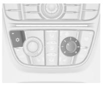
Press to switch on cooling. The LED in the button illuminates to indicate activation. Cooling is only functional when the engine is running and climate control fan is switched on.
