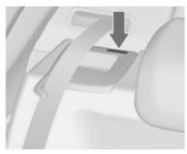
The backrests are properly engaged when the red marks on both sides near the release lever are no longer visible.
