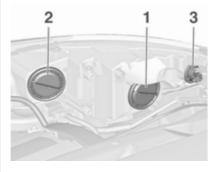
Halogen headlights with separate bulbs for low beam and high beam.
