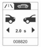
Following Dist.: Displays the distance to a moving vehicle ahead
