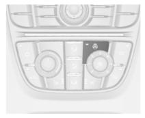
Activate heating by pressing **a**. Activation is indicated by illumination of the LED in the button.
