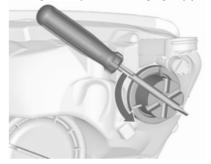
Rotate the cap (3) anticlockwise and remove it. Use the screwdriver to rotate the cap.
