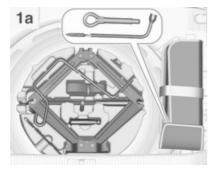
The jack, the tools and a strap for securing a damaged wheel are in the tool box below the spare wheel in the load compartment. The wheel wrench and the towing eye are in the tool bag located in the spare wheel well near the tool box. Spare wheel ▷ 242.
