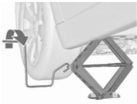
Attach jack handle and with the jack correctly aligned rotate
