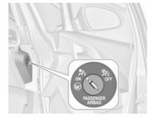
The front passenger airbag system can be deactivated via a keyoperated switch on the passenger side of the instrument panel. Use the ignition key to choose the position:
