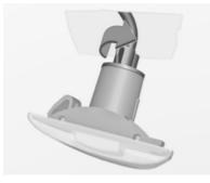
2. Turn bulb holder anticlockwise and remove from housing.
