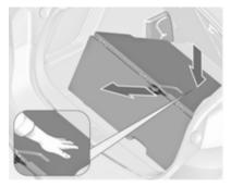
To lower the cover, pull the strap backwards and push down the front centre of the cover at the same time.
