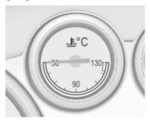
Displays the coolant temperature.
