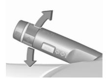
lever up : right turn signal lever down : left turn signal
