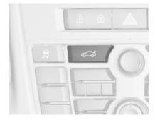
With the doors centrally locked, the boot lid cannot be opened by pressing in the centre console.
