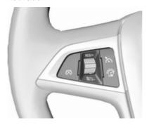
Press @. If cruise control or adaptive cruise control has been activated before, it is switched off when speed limiter is activated and control indicator \( \omega \) extinguishes.
