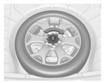
A damaged full size wheel must be stowed outside up in the spare wheel well secured with the wing nut.
