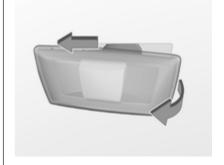
1. Slide lamp to its left side and remove at its right end.
