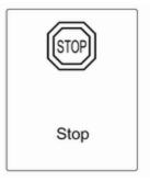
The parking slot suggestion of the system is accepted when the vehicle is stopped by the driver within ten metres after the "Stop" message is given. The system calculates the optimal route into the parking slot. Then it manoeuvres the driver into the slot by giving detailed instructions.
