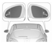
Side blind spot alert is active from speeds of 10 km/h up to 140 km/h. Driving faster than 140 km/h deactivates the system, indicated by low lighting warning symbols and in both exterior mirrors. Reducing the speed again will extinguish the
