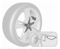
Alloy wheels with centre wheel bolt cap: Disengage centre cap by inserting and pulling the extractor in the recess of the brand emblem. Vehicle tools ♀ 227.
