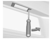
Insert screwdriver in recess of the cover, press to the side and release spring.
