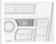
The lane departure warning system is activated by pressing la. The illuminated LED in the button indicates that the system is switched on. When control indicator la in the instrument cluster illuminates green, the system is ready to operate.
