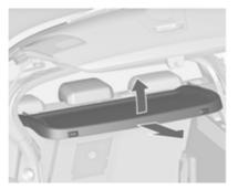
Lift cover at the rear and push it upwards at the front.
