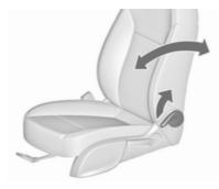
Pull lever, adjust inclination and release lever. Allow the backrest to engage audibly.
