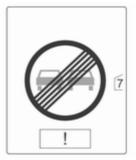
An exclamation mark in a frame indicates that there is an add-on sign detected which cannot be recognised by the system.
