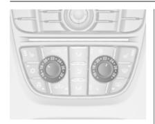
If the minimum temperature **Lo** is set, the climate control system runs at maximum cooling, if cooling **\$\tilde{x}\$** is switched on.
