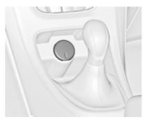
A 12 Volt power outlet is located in the front console.
