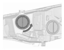
Rotate the cap anticlockwise and remove it.
