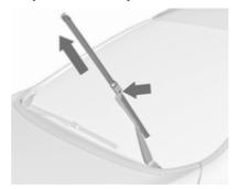
Lift the wiper arm until it stays in the raised position, press button to disengage the wiper blade and remove.
