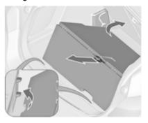
To lift the cover to a higher level, pull the loop backwards and lift the rear edge of the cover onto the corresponding supports.
