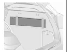
Stow the warning triangle in the space behind the strap on the right side of the load compartment.
