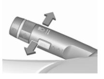
headlight flash: pull lever high beam: push lever
