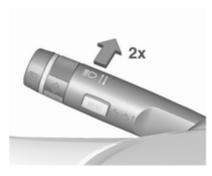
Intelligent light ranging and automatic high beam activation are switched on together by pushing the indicator lever twice. They can be switched on with ignition on.
