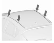
Detach the cover from each mounting point by using a coin.
