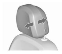
To adjust horizontally, pull the head restraint forwards. It engages in several positions.
