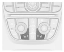
Adjust heating to the desired setting by pressing # for the respective seat one or more times. The control indicator in the button indicates the setting.
