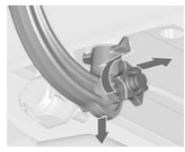
Open the protective flap and turn the key to position  $\widehat{\exists}$  to unlock the coupling ball bar.
