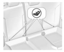
Fasten vehicle-approved ISOFIX child restraint systems to the ISOFIX mounting brackets. Specific vehicle
