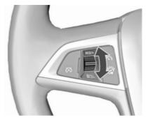
With speed limiter active, hold thumb wheel turned to RES/+ or briefly turn to RES/+ repeatedly until the desired maximum speed is displayed in the Driver Information Centre.
