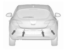
The system has four ultrasonic parking sensors in the rear bumper.
