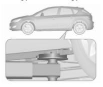
Rear arm position of the lifting platform centrically under the recess of the sill.
