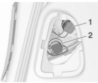
2. Remove the bulb holder by turning and replace the bulb by
