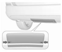
All versions except 3-door hatchback: Press fastenings inward and fold the cover downward at the front. Remove cover.
