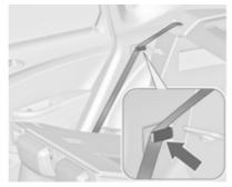
Take the seat belt out of the seat backrest guide and put it behind the retainer as shown in the illustration.
