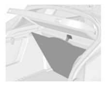
The rear floor cover can be lifted. Hang the loop on the hook on the lower side of the load compartment cover.
