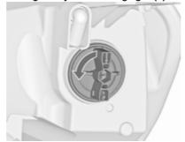
Rotate bulb socket (2) anticlockwise to disengage. Withdraw the bulb socket from the reflector.
