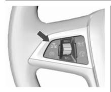
Press F; the current setting is shown in the Driver Information Centre. Press F again to change the alert sensitivity. The setting is also displayed in the top line of the Driver Information Centre.
