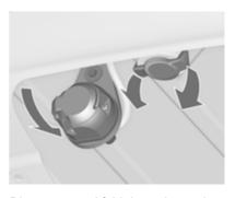
Disengage and fold down the socket. Remove the sealing plug from the opening for the coupling ball bar and stow it.
