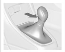
To engage reverse, with the vehicle stationary, depress clutch pedal, press the release button on the selector lever and engage the gear.
