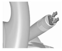
Press the rocker switch to activate the rear window wiper:
