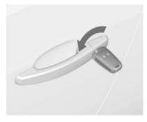
Manually unlock the driver's door by turning the key in the lock. Switch on the ignition and press the central locking button to unlock the other doors, load compartment and fuel filler flap. By switching on the ignition, the anti-theft locking system is deactivated.
