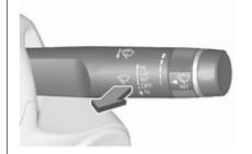
Pull lever. Washer fluid is sprayed onto the windscreen and the wiper wipes a few times.
