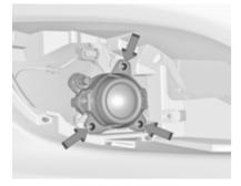
Unscrew three screws and remove fog light assembly from the bumper.
