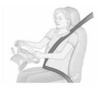
The seat belts are locked during hard acceleration or deceleration of the vehicle, holding the occupants in the seat position. Therefore the risk of injury is considerably reduced.
