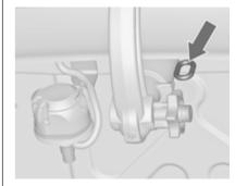
Attach breakaway stopping cable to eye.
