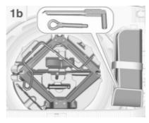
Same content as variant **1a**, but with a foldable wheel wrench instead of the rigid wheel wrench located in the tool bag.
