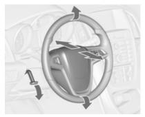
Unlock the lever, adjust the steering wheel, then engage the lever and ensure it is fully locked.
