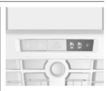
If the control indicator  $\aleph_2$  illuminates for approx. 60 seconds after the ignition is switched on, the front passenger airbag system will inflate in the event of a collision.
