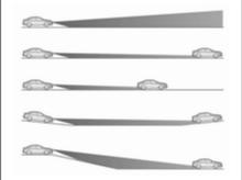
A special topographical evaluation function detects preceding vehicles on hills or slopes by recognising the rear light moving ahead. The system adjusts the height of the light range to ensure optimum illumination on the road ahead without dazzling.
