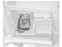
In right-hand drive vehicles, the fuse box is located behind a cover in the glovebox. Open the glovebox, then open the cover and fold it down.
