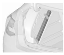
Stow the warning triangle in the recess on the left side of the load compartment.
