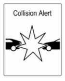
When the distance to a preceding moving vehicle gets too small or when approaching another vehicle too rapidly and a collision is imminent, the collision alert symbol pops-up in the Driver Information Centre.
