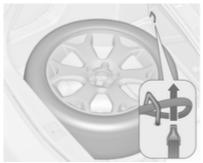
2. Place the loop end of the strap through the front lashing eye on the appropriate side.
