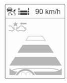
Note that the alert timing sensitivity setting is shared with the following distance setting of the adaptive cruise control. So changing the alert timing sensitivity changes the adaptive cruise control following distance setting.
