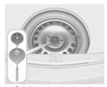
Only 3-door hatchback: position the excentric conus in the recess of the spare wheel before tightening the wing nut.
