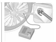
If tyre pressure is more than 1.3 bar, set it to the correct value. Repeat the procedure until there is no more loss of pressure. If the tyre pressure has fallen below 1.3 bar, the vehicle must not be used. Seek the assistance of a workshop.
