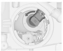
Rotate the bulb holder anticlockwise to disengage. Withdraw the bulb holder from the reflector.
