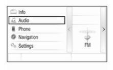
In the Driver Information Centre, Infotainment related information and menus are shown. The menus on the Driver Information Centre are operated via the five-way controller on the right-hand side of the steering wheel.
