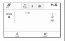
Activating the radio function Press the RADIO button.
