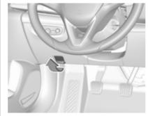
Pull the release lever and return it to its original position.
