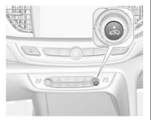
Press so to activate the air recirculation mode. The LED in the button illuminates to indicate activation.
