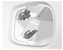
2. Unscrew the two plastic securing nuts from the inside by hand.
