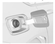
Place the nozzle in straight position to the filler neck and press with slight force to insert.
