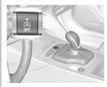
Deactivate the stop-start system manually by pressing . Deactivation is indicated when the LED in the button illuminates.
