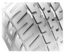
The legally permissible minimum tread depth (1.6 mm) has been reached when the tread has worn down as far as one of the tread wear indicators (TWI). Their position is indicated by markings on the sidewall.
