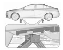
Ensure the jack is correctly positioned under the relevant vehicle jacking point.
