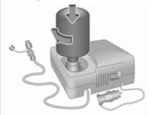
Type 2: remove screw plug from the compressor and from the sealant bottle. Screw the bottle on the compressor without removing the tinfoil from the bottle.
