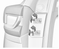
Open the covers with screwdriver. Unscrew and remove both screws.
