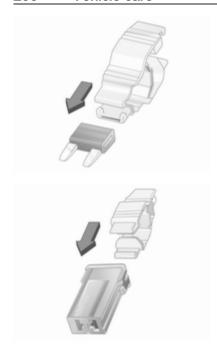
Place the fuse extractor on the various types of fuse from the top or side, and withdraw fuse.
