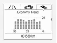
Displays the average consumption development over a distance of 50 km. Filled segments display the consumption in 5 km steps and shows the effect of topography or driving behaviour on fuel consumption.
