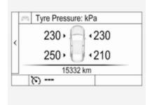
System status and pressure warnings are displayed by a message indicating the corresponding tyre in the Driver Information Centre.
