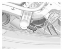
Rotate the cap anticlockwise and remove it.
