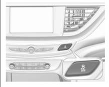
TC can be switched off when spinning of drive wheels is required: press \$\mathbb{B}\$ briefly.
