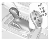
P: park position, wheels are locked, engage only when the vehicle is stationary
