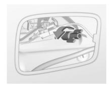
2. Unscrew the plastic securing nut by hand.
