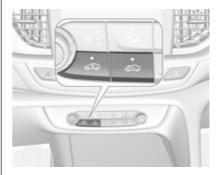
Press \$\simeta\$ to activate external air mode, LED is indicated.
