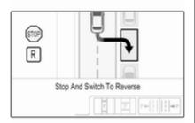
When a slot is detected, a visual feedback on the Colour-Info-Display and an acoustic signal is given.
