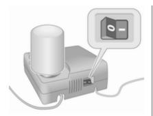
Type 2 indicated by the on/off switch at the side of the compressor.
