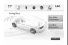
On 8" Info Display a Flex Ride visualisation menu can be displayed by touching 🎓 on the screen. On this page the selected drive mode and active setup are displayed.
