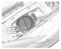
1. Rotate the cap anticlockwise and remove it.
