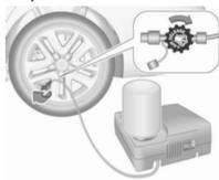
**Type 2:** remove protection cap from filler hose and screw the filler hose to the tyre valve. The air
