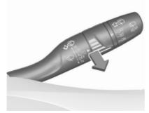
Pull lever. Washer fluid is sprayed onto the windscreen and the wiper wipes a few times.
