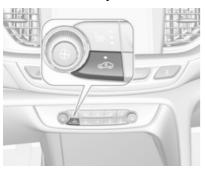
Press so to activate air recirculation mode, LED is indicated.
