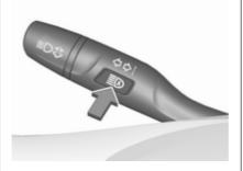
The green control indicator **E** illuminates continuously when the assist is activated, the blue one **E** illuminates when high beam is on.
