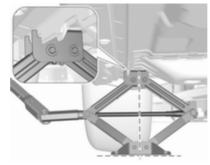
Set the jack to the necessary height. Position it directly below the jacking point in a manner that prevents it from slipping.
