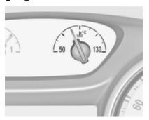
Displays the coolant temperature.
