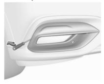
Wrap a cloth around the tip of the flat screwdriver to prevent paint damage. Lever out the faceplate by inserting the screwdriver in the recess and remove it.
