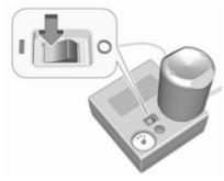
Set the rocker switch on the compressor to I. The tyre is filled with sealant.
