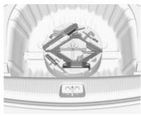
The jack with wheel wrench, the tools, an extension bolt for securing a damaged wheel and the towing eye are placed in the tool box below the spare wheel in the load compartment. Spare wheel ▷ 276.
