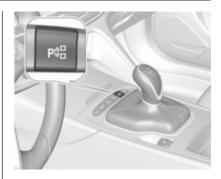
When searching for a parking slot, the system is ready to operate with a short press of P#G.
