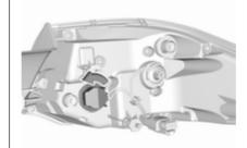
Turn the turn signal light bulb socket anticlockwise and remove it from the light assembly.
