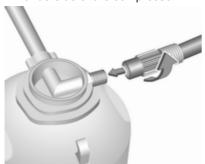
Type 1: screw the compressor air hose to the connection on the sealant bottle and fit the sealant bottle into the retainer on the compressor.
