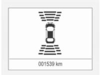
The distance indication can be inhibited by vehicle messages with a higher priority. After dismissing the message distance indication appears again.
