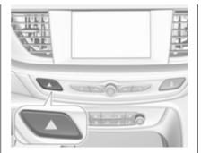
In the event of an accident with airbag deployment, the hazard warning flashers are activated automatically.
