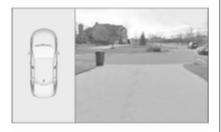
The screen in the Info Display is divided into two parts: on the left there is a view from above the vehicle, and
