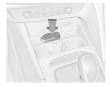
Open the cover of the centre console in front of the gear shift lever. Place the electronic key across with buttons upside in the transmitter pocket beside the power outlet, as shown in the illustration. Other objects, e.g. other keys, transponder, tags, coins etc. must be removed from the pocket.
