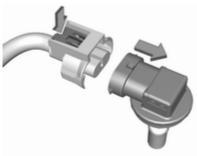
5. Disengage the plug connector by pressing the retaining lug.
