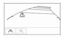
7" Colour-Info-Display: Activation or deactivation of the visual guiding lines and the warning symbols can be changed via touch buttons in the lower zone of the display.
