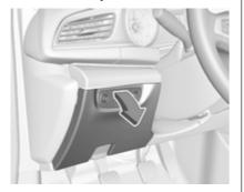
In left-hand drive vehicles, the fuse box is behind a cover in the instrument panel.
