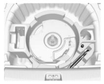
The screwdriver and the towing eye are located below the floor cover in the load compartment, beside the round speaker system component.
