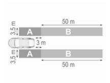
The system sensors cover a zone of approx. 3.5 metres parallel on both vehicle sides and approx. 3 metres rearwards on side blind zone alert (A) and approx. 50 metres rearwards on lane change alert (B) on parallel lanes. The zones start at each exterior mirror. The height of the zone is approx. between 0.5 metres and 2 metres off the ground.
