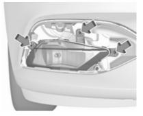
Undo three screws with the torx screwdriver and remove the light assembly to the front.
