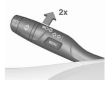
The high beam assist is activated by pushing the turn signal lever twice at a speed above 40 km/h.
