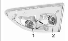
Turn the bulb socket anticlockwise and remove it from the light assembly.
