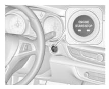
Electronic key must be inside the vehicle.
