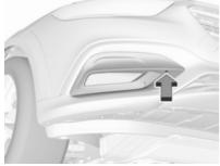
Undo the screw with a torx screwdriver.
