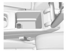
Depending on the infotainment system, one or two USB ports for charging devices are located below the foldable armrest. These ports have also a data connection to the Infotainment system. For further information, see Infotainment manual.
