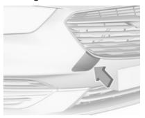
Wrap a cloth around the tip of a flat screwdriver to prevent paint damage. Insert the screwdriver in the slot at the edge of the cap. Release the cap by levering it out carefully.
