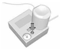
If the pressure is obtained within 10 minutes, correct to the prescribed tyre pressure by using the compressor to increase or decrease with the button over the pressure indicator.
