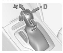
Move selector lever out of position **D** towards the left in position **M**.
