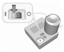
Type 1 indicated by the on/off switch at the top of the compressor.
