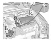
Open the positive terminal protection caps of both vehicle batteries.
