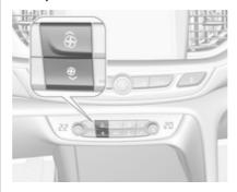
Press upper button  $\hat{*}$  to increase or lower button  $\hat{*}$  to decrease fan speed. The fan speed is indicated as pop-up in the Info Display. Fan speed can also be changed by touch buttons in the climate setting display. Press **Climate** to enter the menu.
