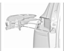
Carefully withdraw tail light assembly from recess and remove. Take care that the cable duct remains in position.
