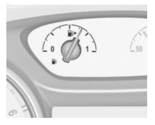
Displays the level in the fuel tank.
