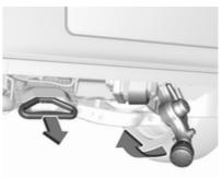
Pull the grip located left to the number plate under the rear bumper fascia at an angle of approx. 45° to the ground.
