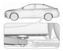
Rear arm position of the lifting platform centrically under the relevant vehicle jacking point.
