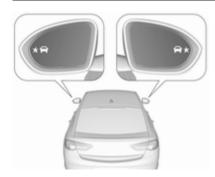
When the vehicle is started, both exterior mirror displays will briefly illuminate to indicate that the system is operating.
