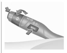
On Baselevel display select by pressing **MENU** on the turn signal lever. Turn the adjuster wheel to select the **Remaining Oil Life** page.
