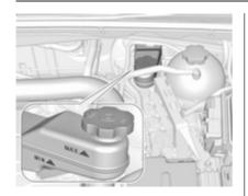
The brake fluid level must be between the **MIN** and **MAX** marks.
