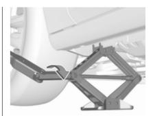
Attach wheel wrench and with the jack correctly aligned rotate wheel wrench until wheel is clear of the ground.
