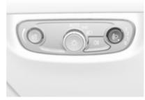
To adapt headlight range to the vehicle load to prevent dazzling: push and then turn to to required position.
