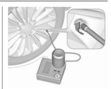
5. **Type 1:** screw the filler hose to the tyre valve.
