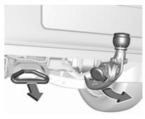
Pull the grip located left of the number plate under the rear bumper fascia at an angle of approx. 45° to the ground.
