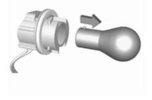
5. Remove and replace the turn signal light bulb.
