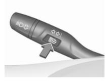
Activate high beam assist by pressing once. High beam is switched on automatically at a speed above 50 km/h. High beam is switched off at a speed below 35 km/h, but high beam assist remains active.
