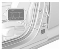
The identification label is located on the front left or right door frame.
