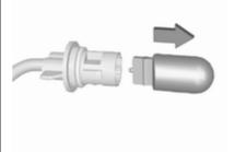
3. Pull bulb from bulb holder and replace it.
