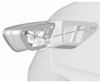
Carefully withdraw the light assembly from the recesses and remove. Take care that the cable duct remains in position.
