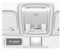
press 來 on/off : interior lights are switched on or off manually
