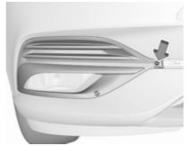
Undo screw with the torx screwdriver and remove the faceplate.
