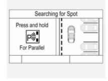
Select parallel or perpendicular parking slot in Driver Information Centre by long press on P#B.
