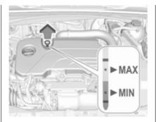
Pull out the dipstick, wipe it clean, reinsert fully, pull out and read the engine oil level.
