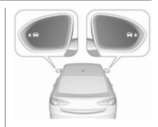
When the vehicle is started, both exterior mirror displays will briefly come on to indicate that the system is operating.
