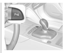
An illuminated LED in the parking assist button P<sup>\*</sup> indicates that the system is ready to operate.
