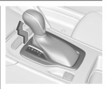
2. Release the selector lever trim. from the centre console. Poke with a finger into the leather socket beside the selector lever and pull the trim up carefully, there is a cable attached to it. Slide trim slightly forward as it is hinged on its rear side. Tilt loose trim to the left side to aviod tensioning the cable.
