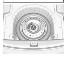
The spare wheel is located in the load compartment beneath the floor covering.
