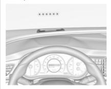
When approaching a detected pedestrian too quickly, a red flashing LED alert or the pop-up symbol ≯ in the head-up display is projected on the windscreen in the driver's field of view. A warning chime is provided. The brake system may prepare for driver braking to occur more rapidly which can cause a brief, mild deceleration. Continue to apply the brake pedal as required.
