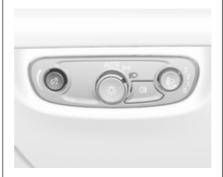
Brightness of the following lights can be adjusted in position AUTO when the light sensor detects night conditions, or in position ≫ or ■D.
