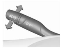
Push lever to switch from low to high beam.
