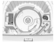
On vehicles with audio speaker system, the tyre repair kit is stowed together with the tools.
