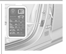
The tyre pressure information label on the left door frame indicates the original equipment tyres and the correspondent tyre pressures.
