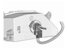
Turn the bulb socket anticlockwise and remove it from the light assembly.
