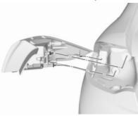
Carefully withdraw tail light assembly from recess and remove. Take care that the cable duct remains in position.
