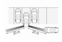
The system sensors cover a zone of approx. 20 metres at 90° to the left or right side behind the vehicle. Rear cross traffic alert is active up to 10 km/h and issues alerts within cross traffic travelling between 0 and 36 km/h.
