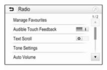
Touch the screen button next to **Audible Touch Feedback** to activate or deactivate the function.
