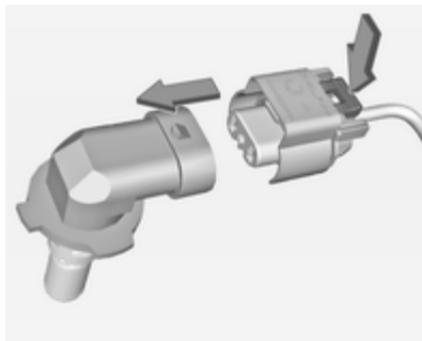
2. Disengage the bulb socket from the plug connector by pressing the retaining lug.
