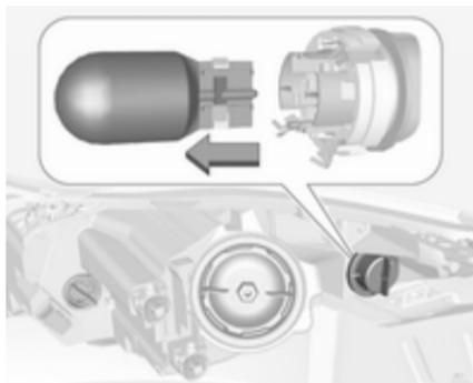
3. Remove the bulb from the socket by pulling.
