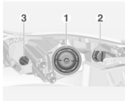
**Bi-Halogen Headlight (1)** with one bulb for low and high beam.
