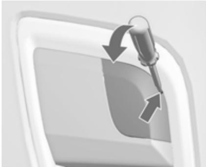
**OPC:** insert screwdriver in the slot at the upper bend of the cap. Release the cap by carefully moving the screwdriver downwards. To prevent damage it is recommended to place a cloth between the screwdriver and the frame.
