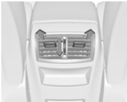
Air vents for rear passenger are in the centre console between the front seats.
