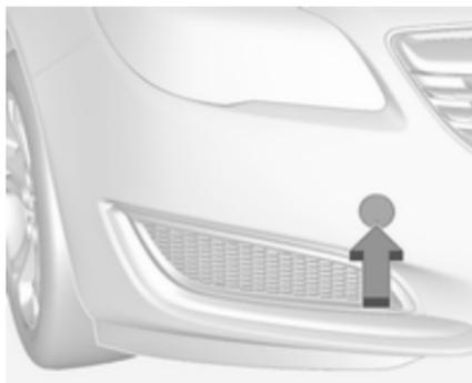
**5-door Hatchback, 4-door Saloon, Sports Tourer:** disengage cap at bottom and remove downwards.
