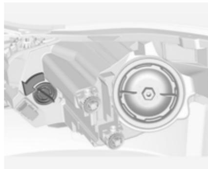
1. Rotate bulb socket anti-clockwise to disengage. Withdraw the bulb socket from the housing.
