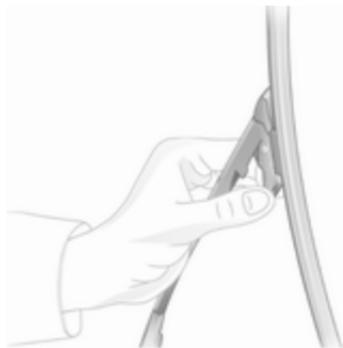
Lift the wiper arm. Press the two catches on the arm, disengage the wiper blade and remove.
