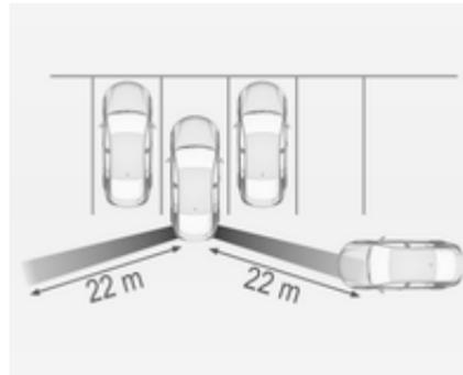
The system sensors cover a zone of approx. 20 metres to the left or right side behind the vehicle.
