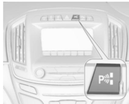
When looking for a parking slot, the system must be activated by pressing the **P** button.
