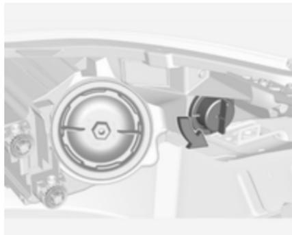
1. Rotate cap anticlockwise and withdraw from the reflector.
