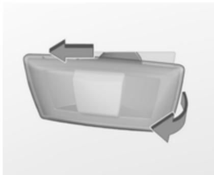
1. On left vehicle side, slide lamp to the front and remove it out of the fender with the rear end.
