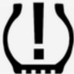
A detected low tyre pressure condition is indicated by the control indicator (⚠) ⇨ 104.
