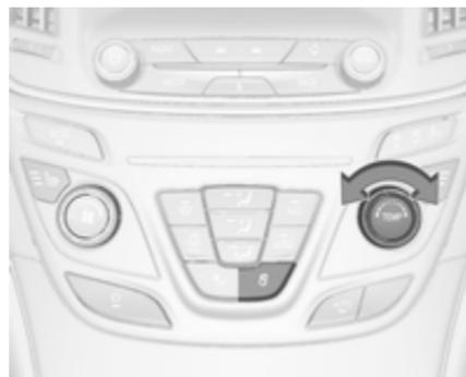
Set temperature by turning controller **TEMP** to the desired value.
