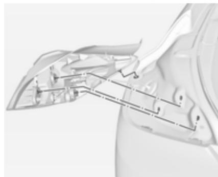
3. Carefully withdraw the light assembly from the recesses and remove.
