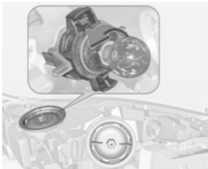
2. Push bulb into socket slightly, rotate anti-clockwise and remove.
