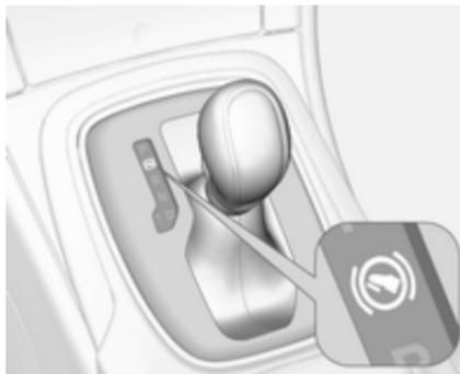
Without applied brake pedal the control indicator
