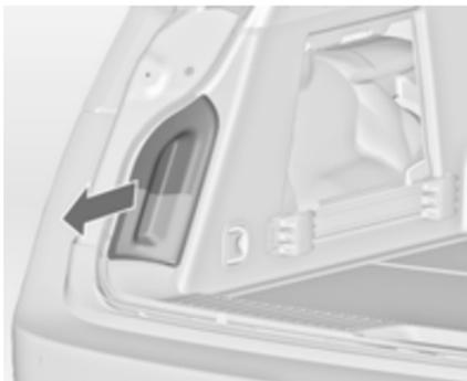
3. Press out lamp housing from the inside of the side trim panel.
