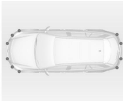
The advanced parking assist system manoeuvres the driver into a parking slot by giving instructions in the Driver Information Centre and acoustic signals.
