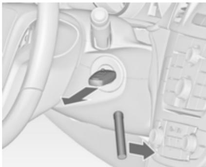
3. Turn special tool to the front and remove key from the ignition switch. Several attempts may be required to successfully remove the key.
