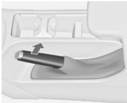
Always apply parking brake firmly without operating the release button, and apply as firmly as possible on a downhill or uphill slope.
