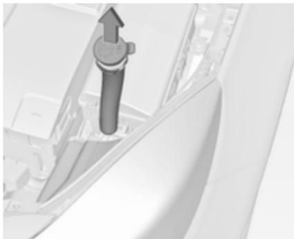
On left vehicle side pull filling pipe out of the windscreen washer fluid container.
