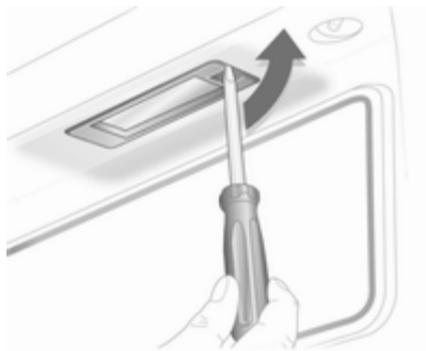
1. Insert screwdriver in bulb housing, press to the side and release spring.
