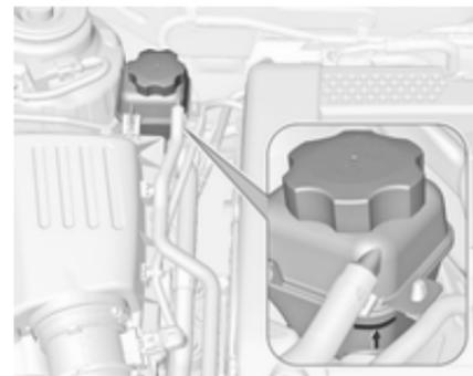
If the cooling system is cold, the coolant level should be above the filling line mark. Top up if the level is low.
