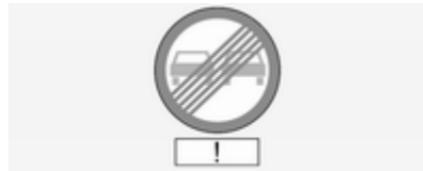
An exclamation mark in a frame indicates that there are additional signs detected which cannot be recognised by the system.
