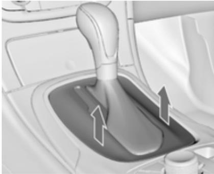
2. Release selector lever trim from centre console at rear, fold upwards and rotate to the left.
