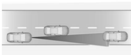
If another vehicle enters your driving path, adaptive cruise control will first consider the vehicle when it is completely in your path. Be ready to take action and press the brake pedal, if you need to brake more quickly.
