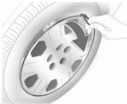
1. Disengage wheel nut caps with a screwdriver and remove. Pull off the wheel cover with the hook. Vehicle tools ⇨ 239.
