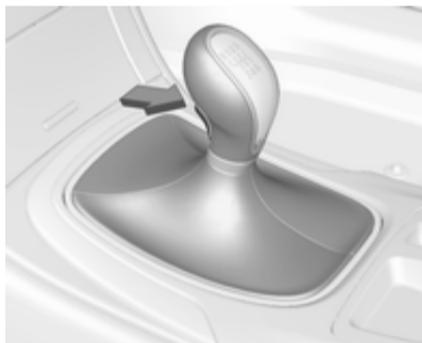
To engage reverse, with the vehicle stationary press the release button on the selector lever and engage the gear.
