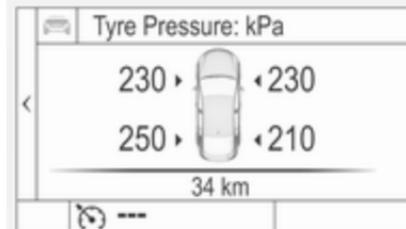
System status and pressure warnings are displayed by a message with the corresponding tyre flashing in the Driver Information Centre.
