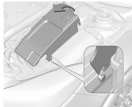
The vehicle battery is covered. Remove the cover to replace the battery. Lift up the cover at the rear and unlatch it at the front.
