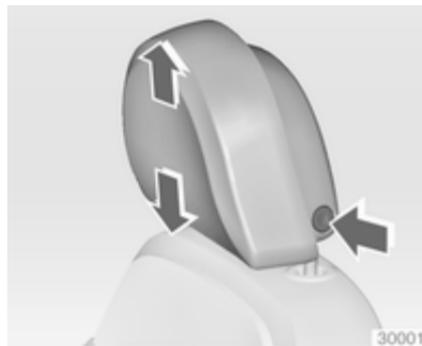
Press release button, adjust height, engage.
