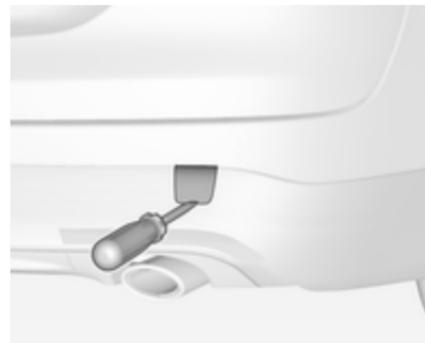
**Country Tourer:** insert a screwdriver in the slot at the lower edge of the cap. Release the cap by carefully moving the screwdriver downwards. To prevent damage it is recommended to place a cloth between the screwdriver and the frame.
