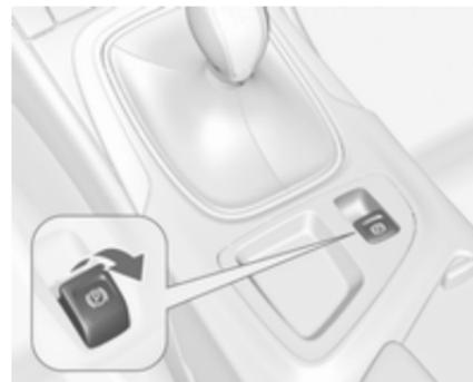
**Applying when vehicle is stationary**
