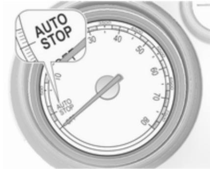
An Autostop is indicated by the needle at the **AUTOSTOP** position in the tachometer. On some versions a control indicator in the instrument cluster lights up when engine is in Autostop.
