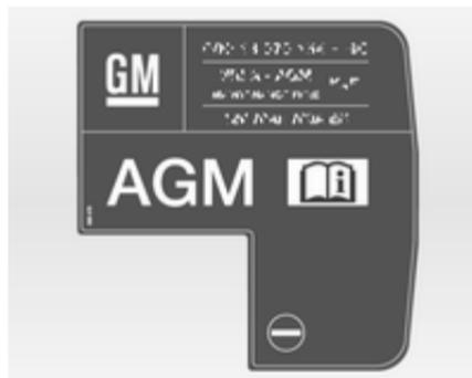
An AGM battery can be identified by the label on the battery. We recommend the use of an original Opel battery.
