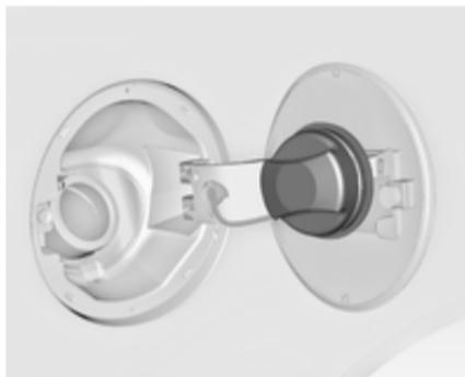
The fuel filler cap can be retained in the bracket on the fuel filler flap.
