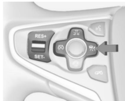
Press button to switch on adaptive cruise control. The control indicator or in the instrument cluster illuminates white.
