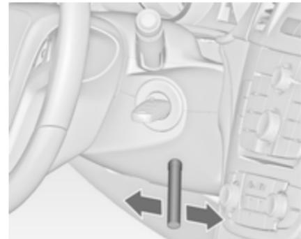
2. Insert the special tool into the opening below the ignition switch as far as it will go and swivel it slightly.
