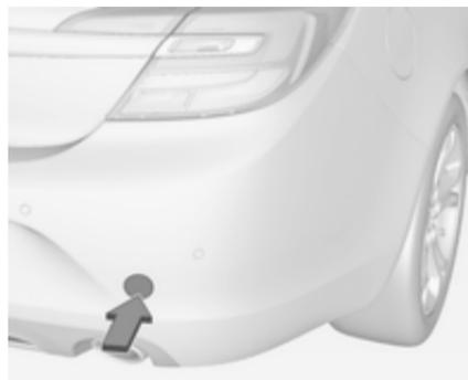
**5-door Hatchback, 4-door Saloon, Sports Tourer, OPC:** disengage cap at bottom and remove downwards.
