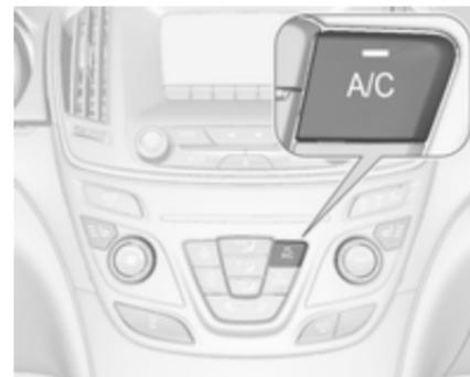
Press button **A/C** to switch on cooling. Activation is indicated by the LED in the button. Cooling is only functional when the engine is running and climate control fan is switched on.
