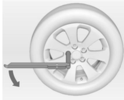
2. Fold out the wheel wrench and install ensuring that it locates securely and loosen each wheel nut by half a turn.
