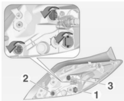
4. Turn bulb holder anticlockwise and remove. Replace bulb by withdrawing or turning:
