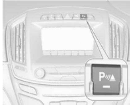
When reverse gear is engaged, the front and rear parking assist is ready to operate.
