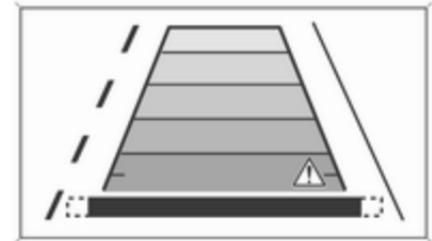
Due to the high position of the camera the rear bumper can be seen on the display as a guide to position.
