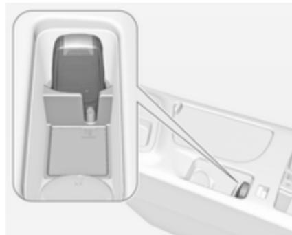
Open the centre console storage area by lifting up the armrest. Place the electronic key in the transmitter pocket. Depress the clutch pedal (manual transmission) or the brake pedal (automatic transmission) and press the **Engine Start/Stop** button. To switch off the engine, press the **Engine Start/Stop** button again. Remove the electronic key from the transmitter pocket.
