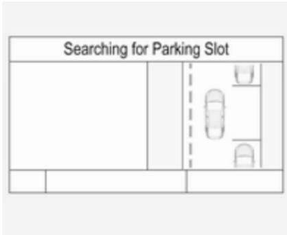
When the vehicle passes a row of cars and the system is activated, the advanced parking assist system begins looking for a suitable parking slot. When a suitable slot is detected,
