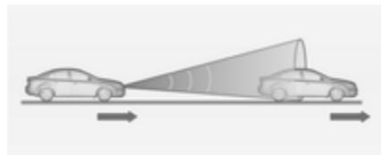
Adaptive cruise control uses a radar sensor to detect the vehicles ahead. If no vehicle is detected in the driving path, the adaptive cruise control will behave like a traditional cruise control.
