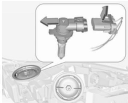
3. Disengage the bulb from the plug connector by unlatching and pulling.
