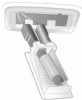
2. Press bulb slightly towards spring clip and remove.
