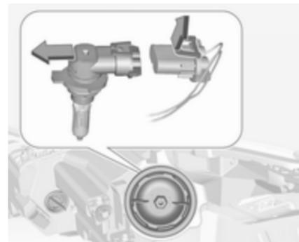
3. Disengage the bulb holder from the plug connector by bending apart slightly the retaining lug.
