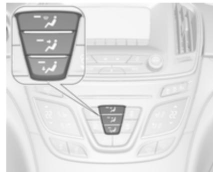
Press appropriate button for desired adjustment. Activation is indicated by the LED in the button.
