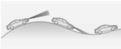
System performance on hills and when towing a trailer depends on vehicle speed, vehicle load, traffic conditions and the road gradient. It may not detect a vehicle in your path while driving on hills. On steep hills, you may have to use the accelerator pedal to maintain your vehicle speed. When going downhill, especially when towing a trailer, you may have to brake to maintain or reduce your speed.
