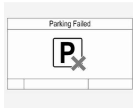
If an object is detected during parking instructions, **Stop** is indicated in the Driver Information Centre. Removing the object will resume the parking manoeuvre. If the object is not removed, the system will be
