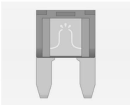
Depending on the type of fuse, a blown fuse can be recognized by its melted wire. Do not replace the fuse until the cause of the fault has been remedied.
