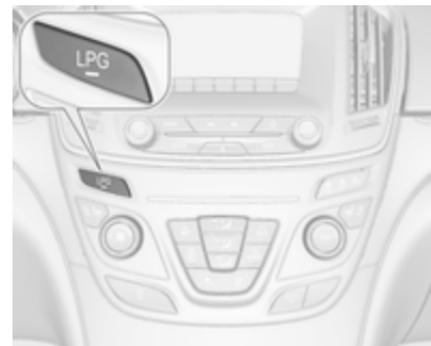
Press the **LPG** button to switch between petrol and liquid gas operation as soon as the required parameters (coolant temperature, gas temperature and minimum engine speed) have been reached. The requirements are usually fulfilled after around 60 seconds (depending on exterior temperature) and the first firm press on the accelerator. The LED status shows the current operating mode.
