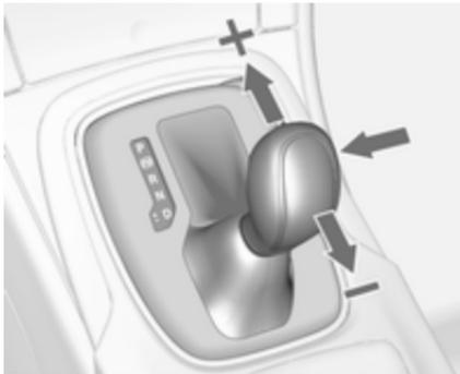
Move selector lever out of position **D** towards the left to select manual mode.
