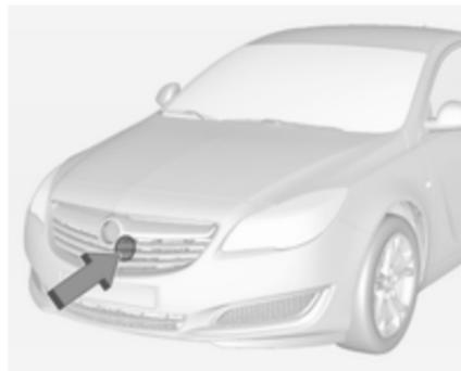
The radar unit is mounted behind the radiator grille below the brand emblem.
