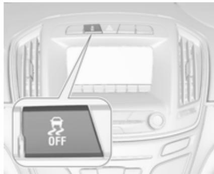
TC can be switched off when spinning of drive wheels is required:
