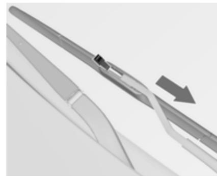
Disengage the wiper blade and remove.
