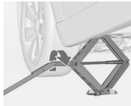
Attach wheel wrench and with the jack correctly aligned rotate wheel wrench until wheel is clear of the ground.
