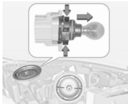
3. Disengage the bulb holder from the plug connector by unlatching and pulling.
