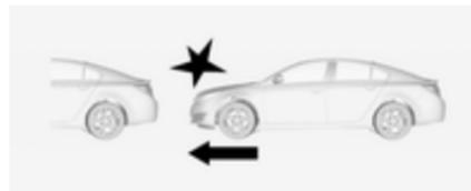
When approaching another vehicle too rapidly, the collision alert warning page will be indicated in the Driver Information Centre. Simultaneously a warning chime sounds. Depress the brake pedal, if it is required by the situation.
