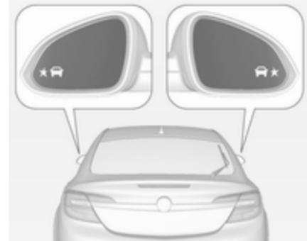
When the vehicle is started, both exterior mirror displays will briefly come on to indicate that the system is operating.
