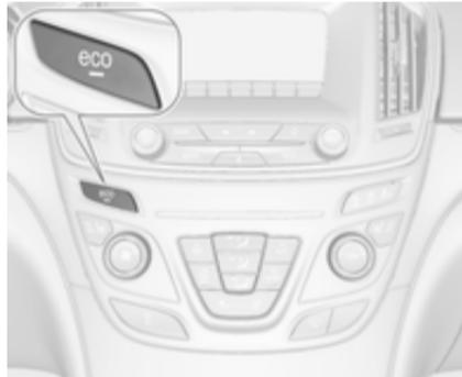
Deactivate the stop-start system manually by pressing the **eco** button. The deactivation is indicated when the LED in the button extinguishes.
