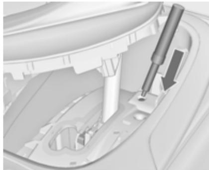
4. Insert it into the opening as far as it will go and move the selector lever out of **P** or **N**. If **P** or **N** is engaged again, the selector lever will be locked in position again. Have the cause of the power supply interruption remedied by a workshop.
