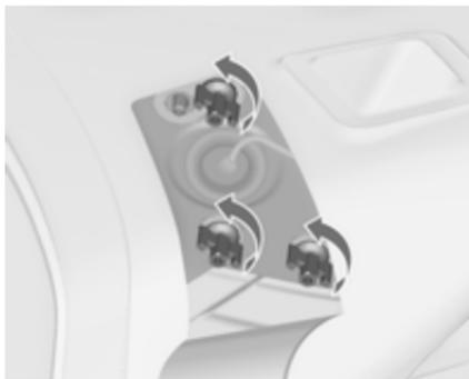
2. Unscrew three plastic securing nuts by hand.
