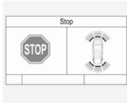
The suggestion of the system is accepted when the vehicle is stopped by the driver within 10 metres after the message is given. The system calculates the optimal route into the parking slot. Then it manoeuvres the driver into the slot by giving detailed instructions.
