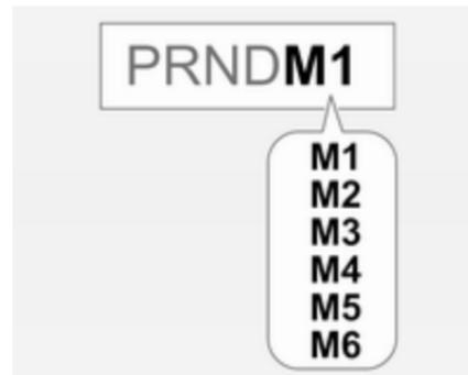
The driving programme in automatic mode or the selected gear in manual mode is indicated in the Driver Information Centre.
