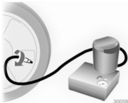
6. Unscrew valve cap from defective tyre.
