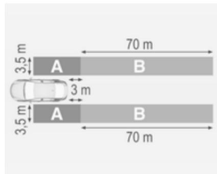
The system sensors cover a zone of approx. 3.5 metres parallel on both vehicle sides and approx. 3 metres rearwards on side blind zone alert (A) and approx. 70 metres rearwards on lane change alert (B) on parallel lanes. The zones start at each exterior mirror. The height of the zone is approx. between 0.5 metres and 2 metres off the ground.
