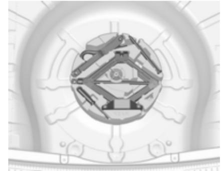
The jack with wheel wrench, the tools, an extension bolt for securing a damaged wheel and the towing eye are placed in the tool box below the spare wheel in the load compartment. Spare wheel ⌀ 250.
