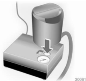
If the prescribed tyre pressure is not obtained within 10 minutes, remove the tyre repair kit. Move the vehicle one tyre rotation. Reattach the tyre repair kit and continue the filling procedure for 10 minutes. If the prescribed tyre pressure is still not obtained, the
