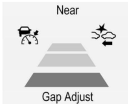
Note that the alert timing sensitivity setting is shared with the following distance setting of the adaptive cruise control ⇨ 173. So changing the alert timing sensitivity changes the adaptive cruise control following distance setting.
