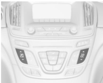
Temperature settings are indicated for driver and passenger side separately on the panels.
