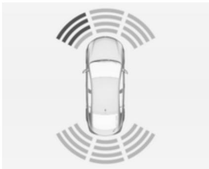
The distance to a front and rear obstacle is indicated by changing distance lines around the vehicle.
