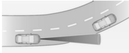
The adaptive cruise control calculates a predicted path based on the centrifugal force. This predicted path considers the current bend characteristic, but cannot consider a future bend change. The system may lose the current vehicle ahead or consider a vehicle which is not in the actual lane. This can happen when entering or exiting a bend or if the bend gets stronger or weaker. If it no
