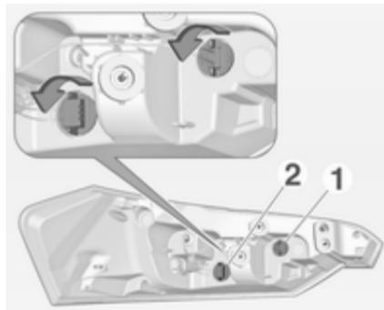
4. Turn bulb holder anticlockwise and remove. Replace bulb by withdrawing:
