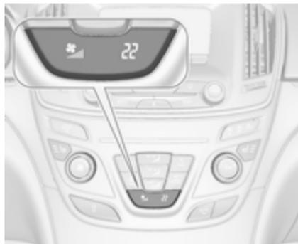
Settings of temperature and fan speed are indicated in the climate display.
