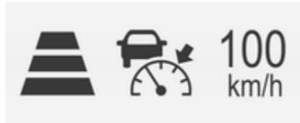
The adaptive cruise control symbol, the following distance setting and set speed are indicated in the Driver Information Centre.
