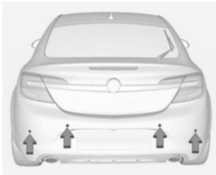
The front-rear parking assist measures the distance between the vehicle and obstacles in front and
