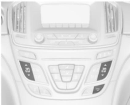
Set desired temperature by touching ▲ for higher temperatures or ▼ for lower temperatures.
