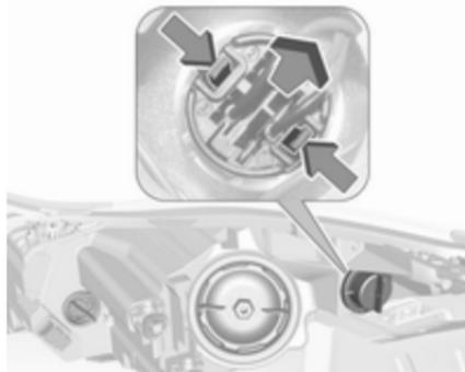
2. Press snap-in tongues together and move socket out of the housing.
