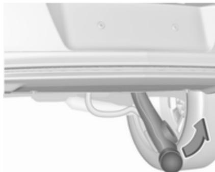
With the flat of the hand, swivel the released coupling ball bar to the right until it engages under the floor. Make sure that the release handle is back in its hidden initial position, otherwise the buzzing tone will not stop.
