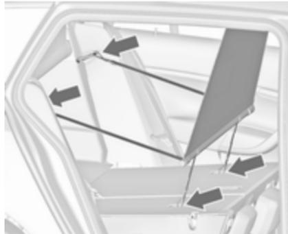
Fit the hooks of the small belts into the Top-Tether mounting loops on the back side of the folded rear seat backrests.
