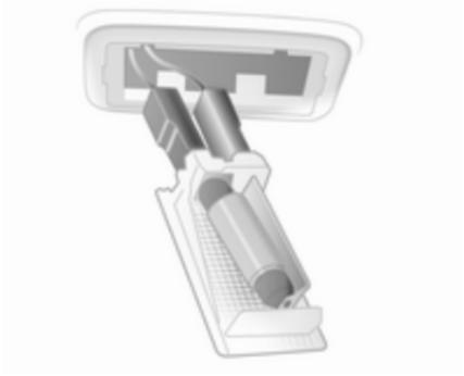
2. Press bulb slightly towards spring clip and remove.
