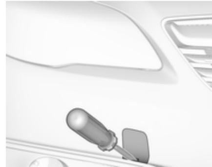
**Country Tourer:** insert a screwdriver in the slot at the lower edge of the cap. Release the cap by carefully moving the screwdriver downwards. To prevent damage, it is recommended to place a cloth between the screwdriver and the frame.
