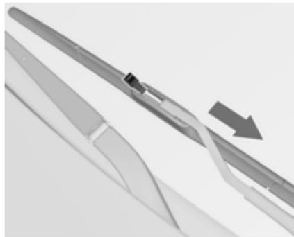
Disengage the wiper blade and remove.
