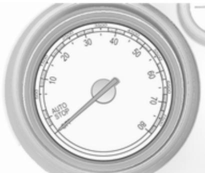
Displays the engine speed.
