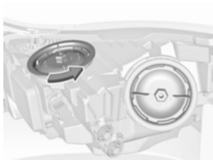
1. Rotate the cap anticlockwise and remove it.
