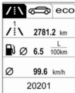
The menu pages of the Baselevel display are selected by pressing **MENU** on the turn signal lever. Main menu symbols are indicated in the top line of the display:
