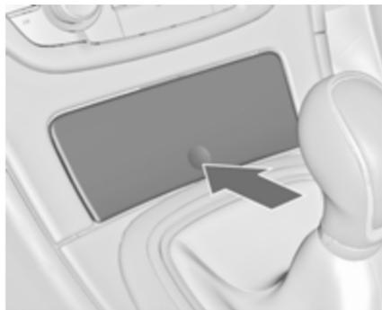
A storage box is located behind a cover below the climate controls. Press cover to open.
