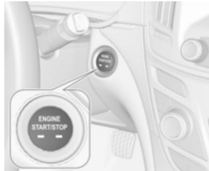
Electronic key must be inside the vehicle.
