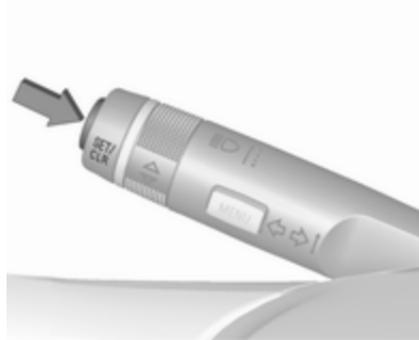
The alert function can be activated or deactivated in the setting menu of the traffic sign assistant page by pressing **SET/CLR** on the turn signal lever or  $\surd$  on the steering wheel.
