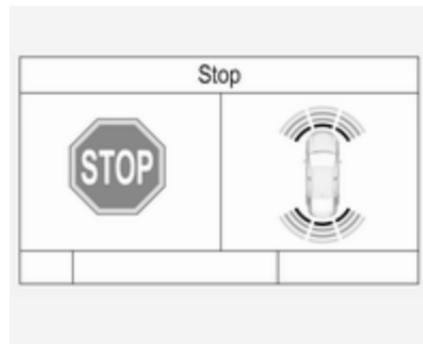
The parking slot suggestion of the system is accepted when the vehicle is stopped by the driver within 10 metres after the "Stop" message is given. The system calculates the optimal route into the parking slot. Then it manoeuvres the driver into the slot by giving detailed instructions.
