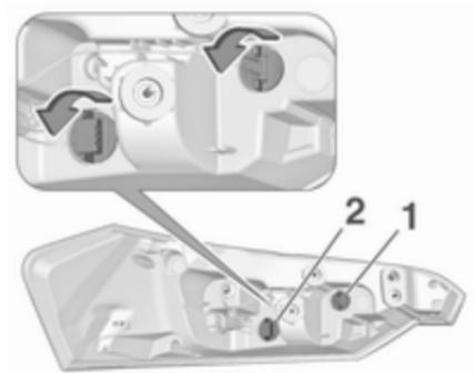
4. Turn bulb holder anticlockwise and remove. Replace bulb by withdrawing:
