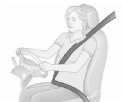
Pull out the seat belt and engage in belt buckle. The seat belt must not be twisted and must fit close against the body. The backrest must not be tilted back too far (maximum approx. 25°).
