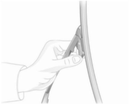
Lift the wiper arm. Press the two catches on the arm, disengage the wiper blade and remove.
