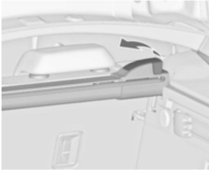
Open the load compartment cover. Pull the release lever on the right side up and hold it. Lift the cover first on the right side and remove from retainers.
