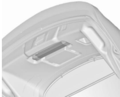
Stow the warning triangle in the space behind the straps on the inside of the tailgate.
