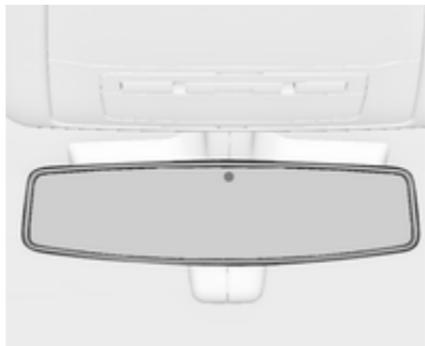
Dazzling by following vehicles at night is automatically reduced by dimming the interior mirror.
