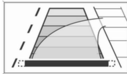
Trajectory lane of the vehicle is shown in accordance with the steering angle.
