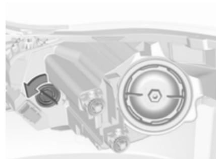
1. Rotate bulb socket anticlockwise to disengage. Withdraw the bulb socket from the housing.
