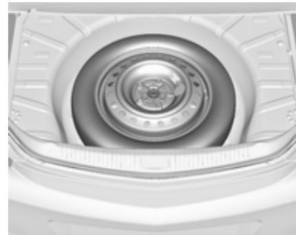
The spare wheel is located in the load compartment beneath the floor covering.
