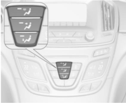
Press appropriate button for desired adjustment. The LED in the button illuminates to indicate activation.
