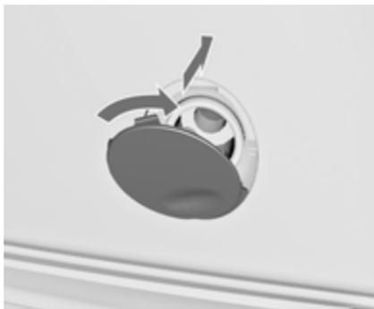
**5-door Hatchback, 4-door Saloon, Sports Tourer, OPC:** insert cap at the bottom, turn slightly clockwise and engage cap.
