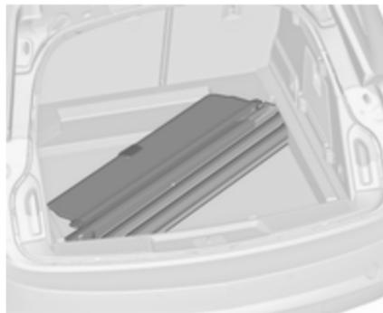
Put the load compartment cover into the hollow with the upper side downwards and with the release lever in the front right edge.
