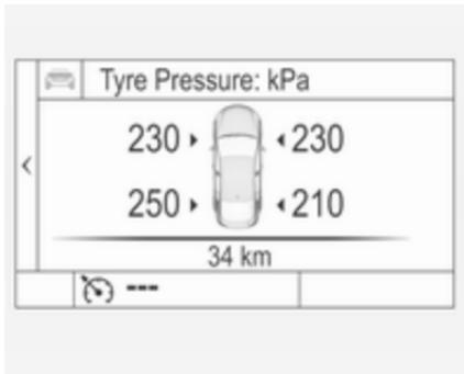
System status and pressure warnings are displayed by a message indicating the corresponding tyre in the Driver Information Centre.
