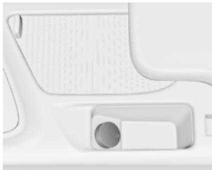
More 12 Volt power outlets are located in the front and rear centre console.
