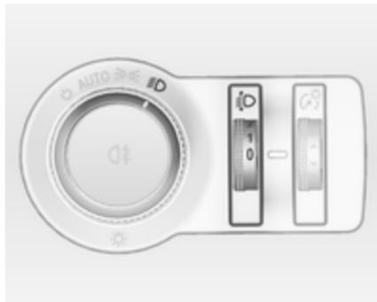
To adapt headlight range to the vehicle load to prevent dazzling: turn thumb wheel
