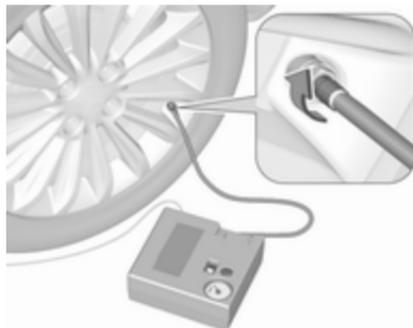
If tyre pressure is more than 1.3 bar, set it to the correct value. Repeat the procedure until there is no more loss of pressure.
