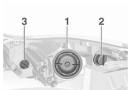
**Bi-Halogen Headlight (1)** with one bulb for low and high beam.
