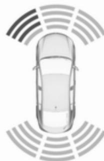
The distance to a front and rear obstacle is indicated by changing distance lines around the vehicle.
