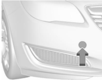
**5-door Hatchback, 4-door Saloon, Sports Tourer:** disengage cap at bottom and remove downwards.
