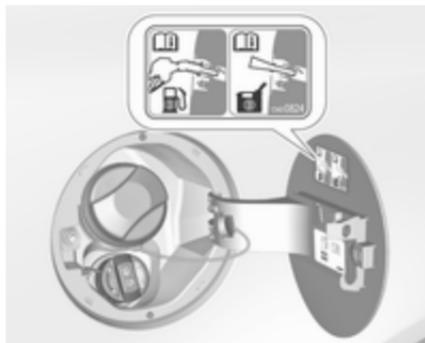
The misfuel inhibitor ensures that the flap of the fuel filler neck can only be opened by using a nozzle for diesel fuel or a funnel for emergency refilling.
