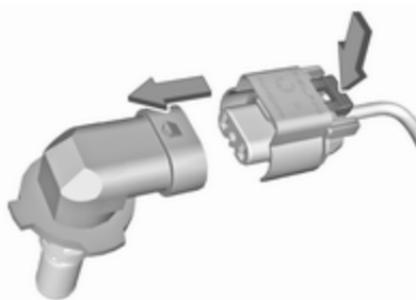
2. Disengage the bulb socket from the plug connector by pressing the retaining lug.
