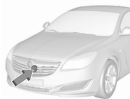
The radar unit is mounted behind the radiator grille below the brand emblem.
