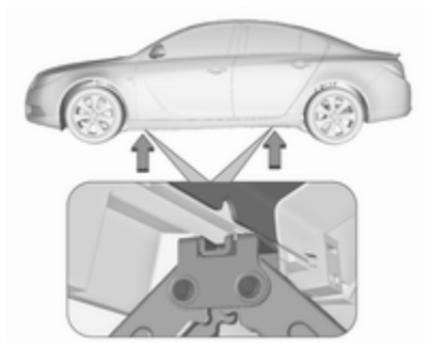
4. Ensure the jack is correctly positioned under the relevant vehicle jacking point.
