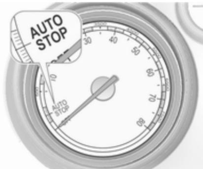
An Autostop is indicated by the needle at the **AUTOSTOP** position in the tachometer. On some versions, a control indicator in the instrument cluster illuminates when engine is in Autostop.
