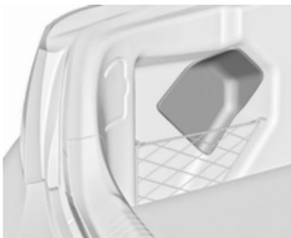
The fuse box is on the left side of the load compartment behind a cover. Remove the cover.
