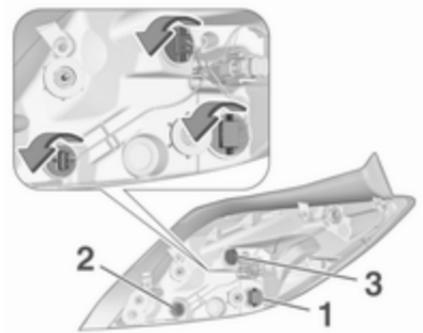
4. Turn bulb holder anticlockwise and remove. Replace bulb by withdrawing or turning:
