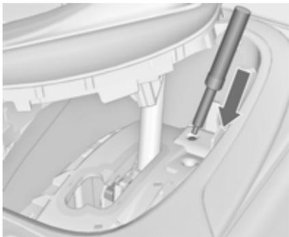
3. Insert the special tool into the opening as far as it will go and move the selector lever out of **P** or **N**. If **P** or **N** is engaged again, the selector lever will be locked in position again. Have the cause of the power supply interruption remedied by a workshop.
