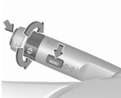
On Baselevel display select the **Settings** Menu by pressing **MENU** on the turn signal lever. Turn the adjuster wheel to select the **Remaining Oil Life** page.
