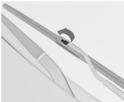
Lift the wiper arm and open the retaining clip.
