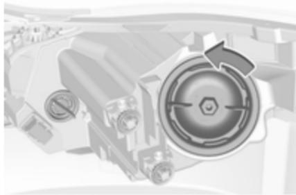
1. Rotate the cap anticlockwise and remove it.
