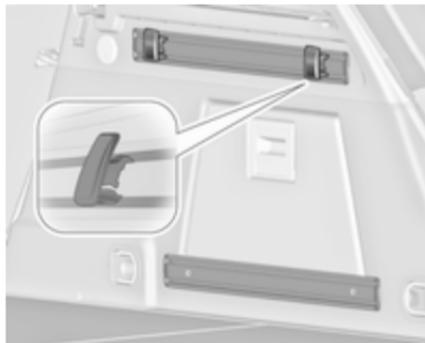
Insert the hook in the desired position first into the upper groove of the rail and then press into the lower groove. To remove, first pull out of the upper groove.
