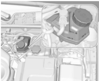
The brake fluid level must be between the **MIN** and the **MAX** marks.
