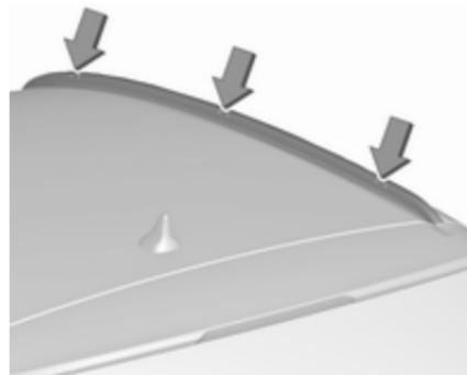
To fasten the roof rack, insert the mounting bolts in the holes indicated in the figure.
