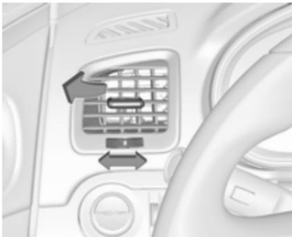
To close the vent, turn the adjuster wheel to **0**.
