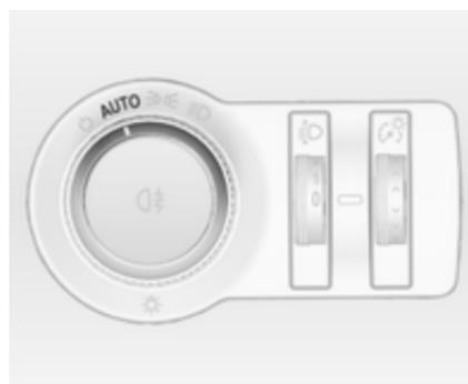
When the automatic light control function is switched on and the engine is running, the system switches between daytime running light and low/high beam automatically depending on the lighting conditions and information given by the rain sensor system.
