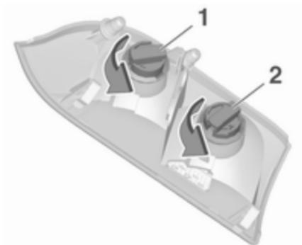
4. Rotate plastic nut anticlockwise and remove from the bulb holder.
