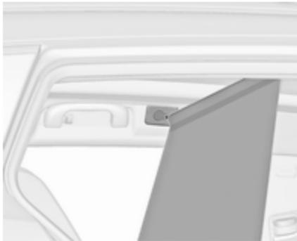
Front installation openings in the roof frame: latch rod of the net at one side, compress rod and latch at the other side.
