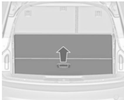
Open the load compartment floor by pulling the handle. Fold and place the floor behind the rear seats.
