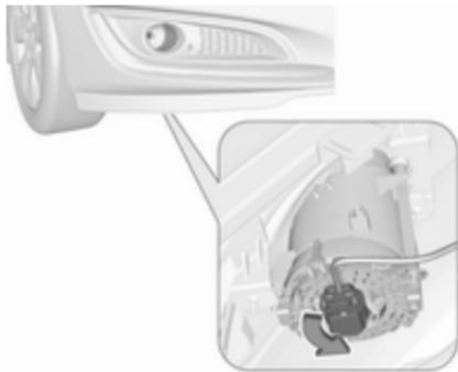
1. Turn the bulb holder anticlockwise and remove it from the reflector.
