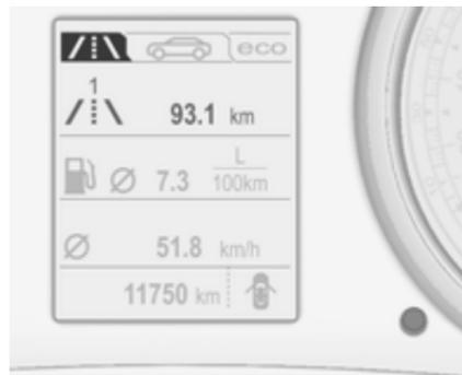
The recorded distance since the last reset is displayed on the trip computer page. Two trip odometer are selectable for different trips.
