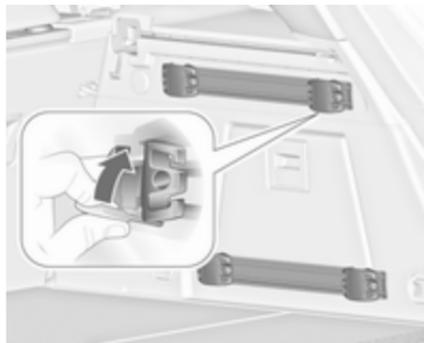
Fold open the handle plate, insert the adapter into the upper and lower groove of the rail and move to the required position. Turn the handle plate upwards to lock the adapter. To remove, turn the handle plate downwards and move out of the rail.
