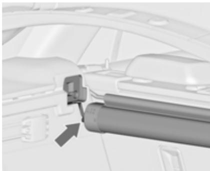
Insert the cassette into the retainers on left and right side. Note the signs **L** (left side) and **R** (right side) on the cassette as an installation hint.
