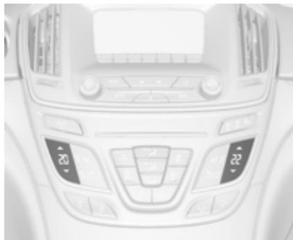
Temperature settings are indicated separately on the panels for driver and passenger side.
