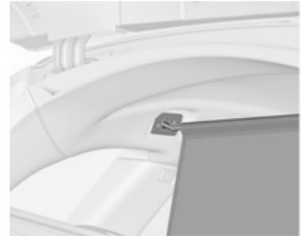
Pull out the net from the cassette and latch the rod of the net at one side into the rear installation opening in the roof frame. Compress the rod and latch at the other side.
