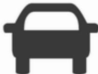
The green illuminated vehicle ahead control indicator
