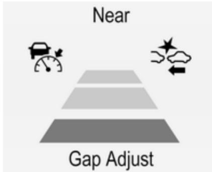
Note that the alert timing sensitivity setting is shared with the following distance setting of the adaptive cruise control ↻ 184. So changing the alert timing sensitivity changes the adaptive cruise control following distance setting.
