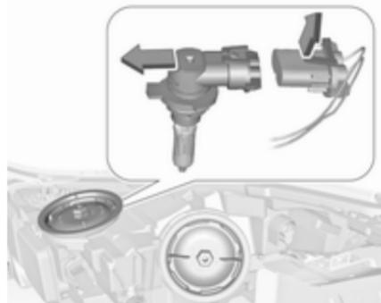
3. Disengage the bulb from the plug connector by unlatching and pulling.
