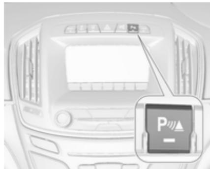
Manual deactivation is possible by pressing the parking assist button **P** with a warning triangle briefly.
