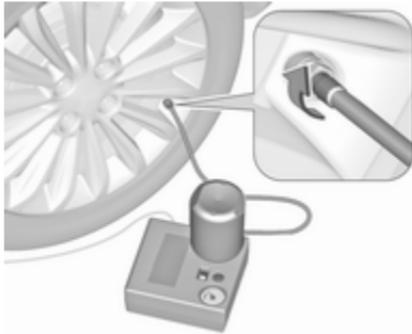
6. Unscrew valve cap from defective tyre.
