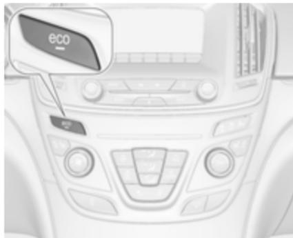
Deactivate the stop-start system manually by pressing **eco**. Deactivation is indicated when the LED in the button extinguishes.
