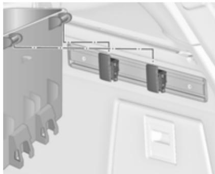
Install two hooks in the upper rail. Insert the upper brackets of the box from above into the hooks.
