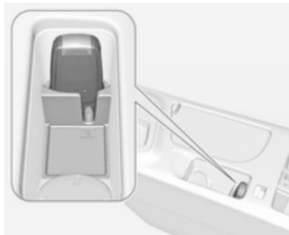
Open the centre console storage area by lifting up the armrest. Place the electronic key in the transmitter pocket.
