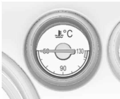
Displays the coolant temperature.
