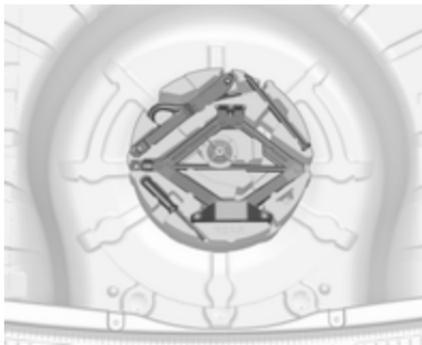
The jack with wheel wrench, the tools, an extension bolt for securing a damaged wheel and the towing eye are placed in the tool box below the spare wheel in the load compartment. Spare wheel ⇨ 263.
