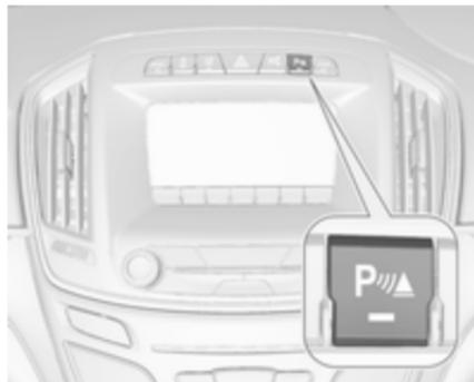
An illuminated LED in the parking assist button **P**
