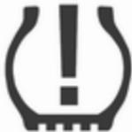
A detected low tyre pressure condition is indicated by the control indicator (⚠) ⇨ 109.
