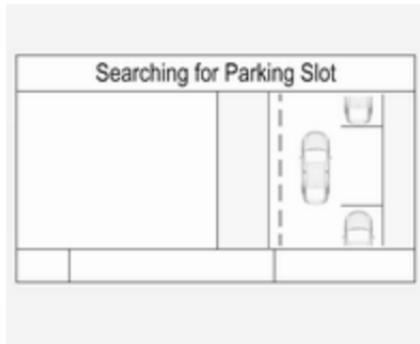
When the vehicle passes a row of cars and the system is activated, the advanced parking assist system begins looking for a suitable parking slot. When a suitable slot is detected, a visual feedback and acoustic signals are given in the Driver Information Centre.
