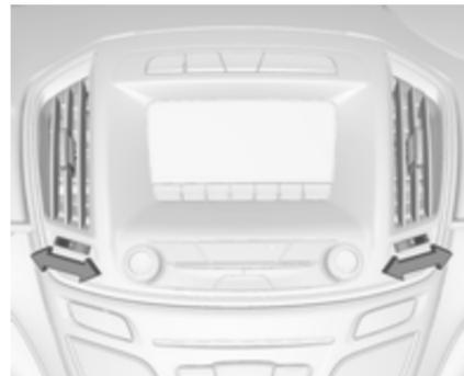
To open the vent, turn the adjuster wheel to
