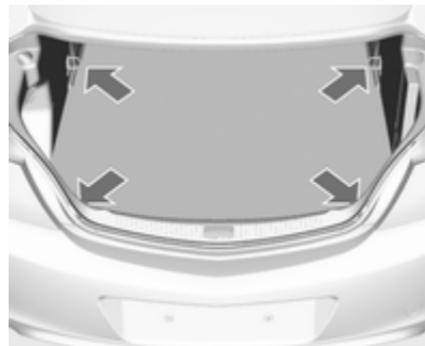
The lashing eyes are designed to secure items against slippage, e.g. using lashing straps or luggage net.
