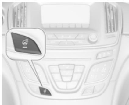
Activate heating by pressing ☀. Activation is indicated by the LED in the button.
