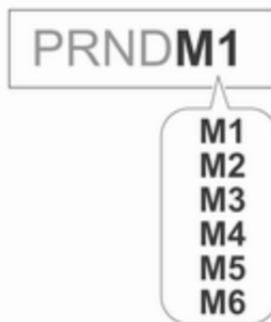
The mode or selected gear is shown in the transmission display.
