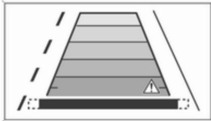
Due to the high position of the camera the rear bumper can be seen on the display as a guide to position.
