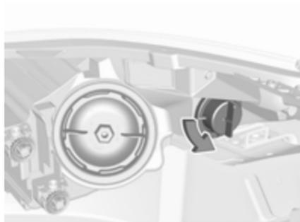
1. Rotate cap anticlockwise and withdraw from the reflector.
