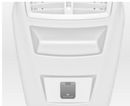
A 230 Volt power outlet is located in the rear centre console. If ignition is on and a device is plugged in, an LED in the outlet illuminates green.
