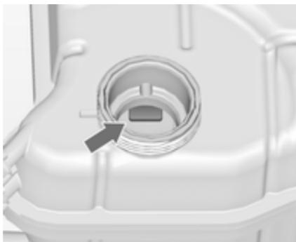
On another version, the filling line mark is inside the filler opening. To check, open the cap.
