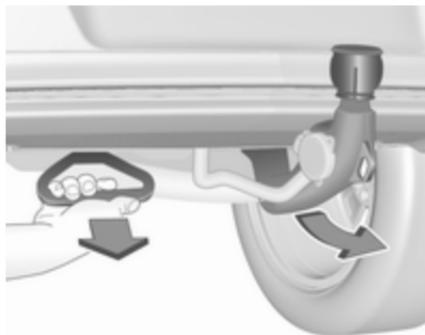
Pull the grip located left of the number plate under the rear bumper fascia at an angle of approx. 45° to the ground.
