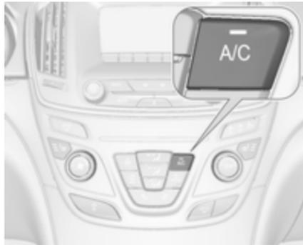
Press **A/C** to switch on cooling. The LED in the button illuminates to indicate activation. Cooling is only functional when the engine is running and climate control fan is switched on. Press **A/C** again to switch off cooling. The air conditioning system cools and dehumidifies (dries) cabin air as required. Therefore condensation may form and is drained under the vehicle. If no cooling or drying is required, switch off the cooling system for fuel saving reasons.
