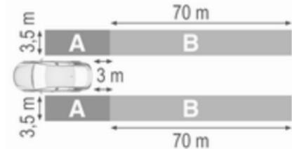
The system sensors cover a zone of approx. 3.5 metres parallel on both vehicle sides and approx. 3 metres rearwards on side blind zone alert (A) and approx. 70 metres rearwards on lane change alert (B) on parallel lanes. The zones start at each exterior mirror. The height of the zone is approx. between 0.5 metres and 2 metres off the ground.
