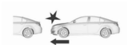
When the distance to a preceding moving vehicle gets too small or when approaching another vehicle too rapidly and a collision is imminent, the collision alert symbol pops-up in the Driver Information Centre.
