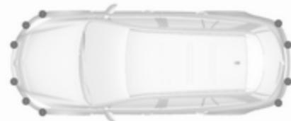
The advanced parking assist system manoeuvres the driver into a parking slot by giving instructions on the Driver Information Centre and acoustic signals. The driver must control acceleration, braking, steering and gear shifting.
