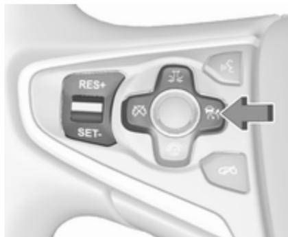
Press to switch on adaptive cruise control. The control indicator or in the instrument cluster illuminates white.
