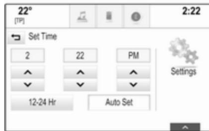
Select the **Auto Set** screen button at the bottom of the screen. Activate either **On - RDS** mode or **Off - Manual** mode.
