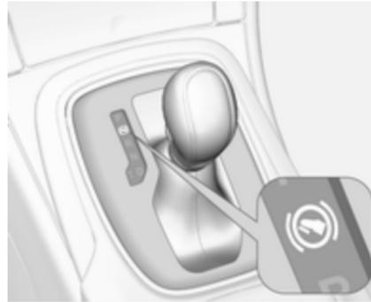
Without applied brake pedal the control indicator (P) illuminates.
