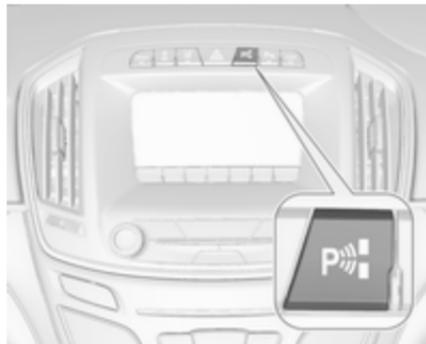
When searching for a parking slot, the system is ready to operate by pressing button
