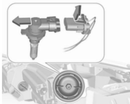
3. Disengage the bulb holder from the plug connector by slightly bending apart the retaining lug.
