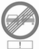
An exclamation mark in a frame indicates that there is an additional sign detected which cannot be clearly identified by the system.
