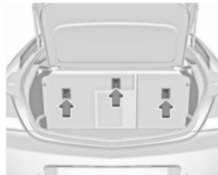
In addition to the ISOFIX mounting, fasten the Top-Tether strap to the Top-Tether fastening eyes. The strap must run between the two guide rods of the head restraint.
