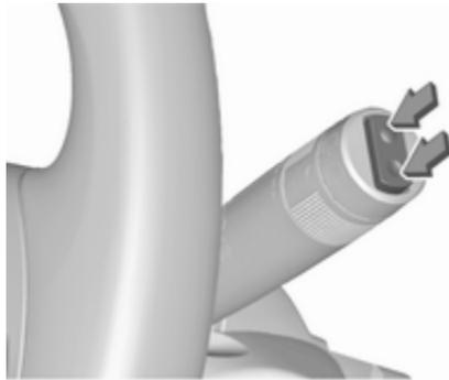
Push the rocker switch to activate the rear window wiper:
