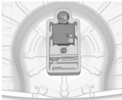
The tyre repair kit is in a compartment under the floor cover in the load compartment.
