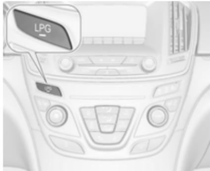
Press **LPG** to switch between petrol and liquid gas operation as soon as the required parameters (coolant temperature, gas temperature and
