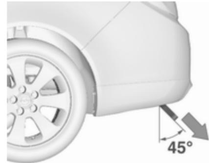
A buzzing tone sounds as a warning when the release handle is pulled out and the ball neck is disengaged.
