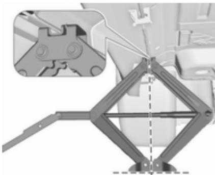
5. Set the jack to the necessary height. Position it directly below the jacking point in a manner that prevents it from slipping.
