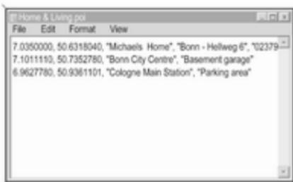
The POI data need to be entered into the text files in the following format:
