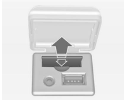
Press on the inserted SD card to unlock it, and then carefully pull the SD card out of the SD card slot.
