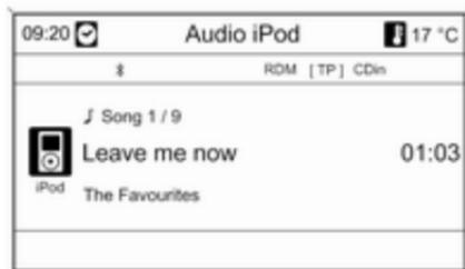
Press the **CD/AUX** button once or several times to activate the audio iPod mode.
