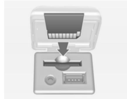
Push the SD card with the cut-out edge on the right side (see image above) carefully into the SD card slot until the card engages.
