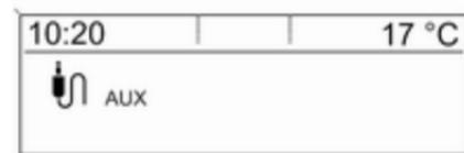
An audio source that is connected to the AUX input can be operated only via the control elements of the audio source.
