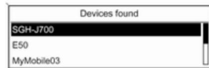
Select the desired mobile phone from the list. The SAP passcode prompt is shown on the Infotainment display containing a 16-digit code.
