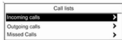
Via the menu **Call lists** the user can view incoming, outgoing and missed calls and dial the relevant numbers. To start a dialling process: select the desired call list, an entry in the call list and finally the desired telephone number.
