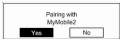
As soon as the Phone portal has detected the mobile phone, the connection set-up can be confirmed. The mobile phone is adopted in the device list and can be operated via the Phone portal.
