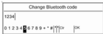
Select **Change Bluetooth code**. On the menu displayed, edit the actual Bluetooth code and accept the modified code using **OK**.
