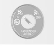
The front passenger airbag system can be deactivated via a keyoperated switch on the passenger side of the instrument panel. Use the ignition key to choose the position:
