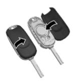
Open the unit. Replace the battery (battery type CR 2032), paying attention to the installation position. Close the unit and synchronise.
