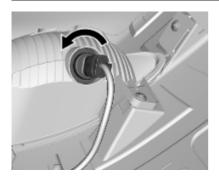
1. Turn the bulb holder anticlockwise and remove it from reflector.
