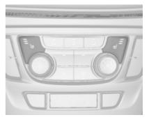
Adjust heating to the desired setting by pressing # for the respective seat one or more times. The LED in the button indicates the setting.
