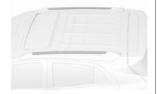
The roof rack has side rails attached to the roof.
