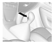
To engage reverse, with the vehicle stationary, depress clutch pedal, press the release button on the selector lever and engage the gear.
