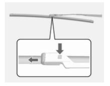
Lift the wiper arm, press button to disengage the wiper blade and remove.
