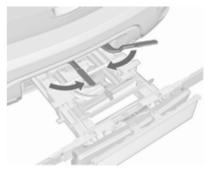
Swivel both clamping levers inwards as far as they will go. Fasten strap.
