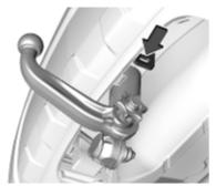
Attach breakaway stopping cable to eye.
