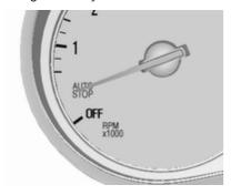
An Autostop is indicated by the needle at the **AUTOSTOP** position in the tachometer.
