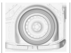
The spare wheel is located in the load compartment beneath the floor covering. It is secured with a wing nut.
