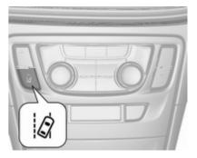
The lane departure warning system is activated by pressing lâ. The illuminated LED in the button indicates that the system is switched on.
