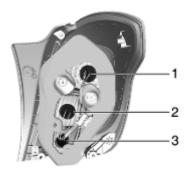
Tail / stop light, if not equipped with LEDs (1)
