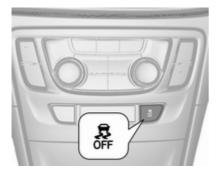
TC can be switched off when spinning of drive wheels is required: press \$\mathbb{B}\$ briefly.
