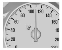
When the control indicator !a in the instrument cluster illuminates green, the system is ready to operate.
