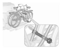
Use the short accessory mounting bracket to attach the third bicycle. The bracket must be fixed between the frames of the second and third bicycle.
