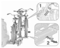
Hold frame (1) of rearmost bicycle with one hand and pull the loop (2) to disengage.
