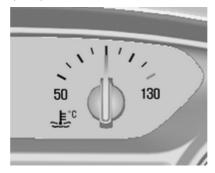
Displays the coolant temperature.
