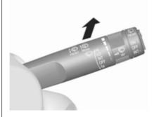
Push lever. Washer fluid is sprayed onto the rear window and the wiper wipes a few times.
