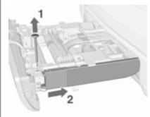
To install the tail lights, remove both pins (1). Pull tail lights out of the retainer towards the front (2) and downwards and swivel them to the side.
