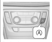
Deactivate the stop-start system manually by pressing (A).
