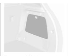
The tyre repair kit is located in the right side of rear compartment.
