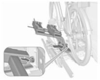
Apply the adapter to the rear carrier system, as shown in the illustration.
