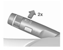
The high beam assist is activated by pushing the indicator lever twice. The high beam is switched on automatically at a speed above 40 km/h.
