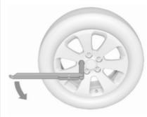
Fold out the wheel wrench and install ensuring that it is located securely and loosen each wheel nut by half a turn.
