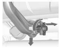
Open the protective flap and turn the key to position to unlock the coupling ball bar.
