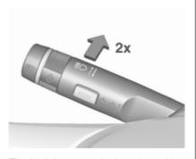
The high beam assist is activated by pushing the indicator lever twice. The high beam is switched on automatically at a speed above 40 km/h.
