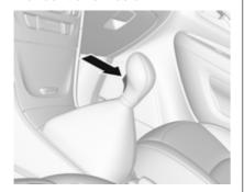
Reverse: with the vehicle stationary, depress clutch pedal, press the release button on the selector lever and engage the gear.
