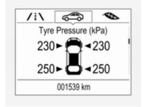
Select the **Tyre pressure** page under the **Vehicle Information Menu** in the Driver Information Centre  $\stackrel{\triangleright}{\circ}$  97.
