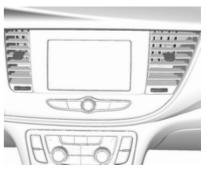
To open the vent, turn the adjuster wheel to the right. Adjust the air amount at the vent outlet by turning the adjuster wheel.
