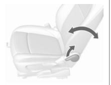
Pull lever, adjust inclination and release lever. Allow the seat to engage audibly.
