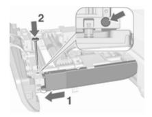
Push the tail lights into the retainer (1). Insert pins into the designated holes of the retainer and the tail lights (2).
