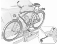
Rotate the pedals into position, as shown in the illustration, and put the bicycle on the wheel recess. Make sure that the bicycle stands centrally on the wheel recesses.
