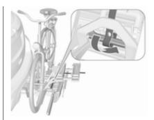
Guide the strap attached to the adapter underneath the lever when folding back the rear carrier system. Fasten the strap.
