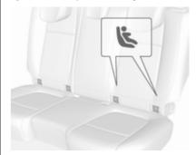
The vehicle might be equipped with guides in front of the mounting brackets to support the installation of the child restraint system.
