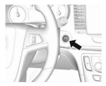
Electronic key must be inside the vehicle.
