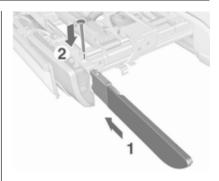
Push the tail lights into the retainer (1) and reinstall pins (2) all the way to attach the lights.
