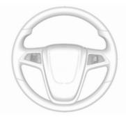
Cruise control and speed limiter are operated via the controls on the left side of the steering wheel.
