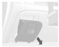
In left-hand drive vehicles, the interior fuse box is located on the underside of the driver's side instrument panel.
