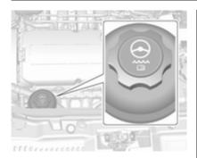
Power steering fluid level normally does not need to be checked. If an unusual noise sounds during steering or the power steering reacts conspicuously, seek the assistance of a workshop.
