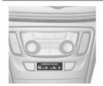
As long as the control indicator \*\*\* is not illuminated, the front passenger airbag system will inflate in the event of a collision.
