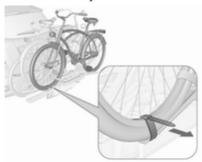
Additionally, secure both bicycle wheels of the third bicycle to the wheel recesses using the tensioning straps.
