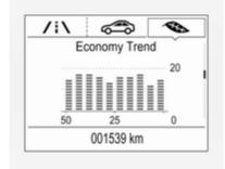
Displays the average consumption development over a distance of 50 km. Filled segments display the consumption in 5 km steps and shows the effect of topography or driving behaviour on fuel consumption.
