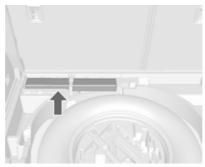
Stow the warning triangle below the floor cover in the load compartment. Secure it with the strap.
