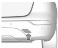
Wrap a cloth around the tip of a flat screwdriver to prevent paint damage. Insert the screwdriver in the slot at the lower bend of the cap. Release the cap by carefully moving the screwdriver downwards.
