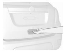
After unlocking, push the touchpad switch and open the tailgate.
