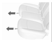
Pull the loop under the seat cushion and fold down the seat cushion.
