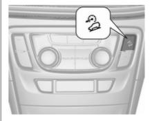
At speeds below approx. 40 km/h, press 2. The green control indicator 3 flashes in the instrument cluster, to
