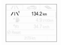
Select /i\ by pressing Menu on the turn signal lever. Turn adjuster wheel and select /i\1 or /i\2. Each trip odometer page can be reset separately by pressing SET/CLR on the turn signal lever for a few seconds on the respective menu.
