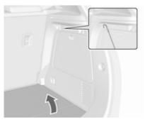
Mount the cover to the hook at the sidewall.
