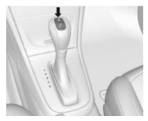
Move selector lever to position **M**. Press button on the selector lever:
