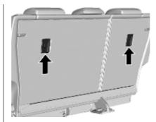
For non-ISOFIX child restraints, fasten the Top-Tether strap to the Top-Tether anchors.
