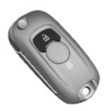
Press to unlock the doors and load compartment. Open the doors by pulling the handles. To open the tailgate, push the touchpad switch below the handle.
