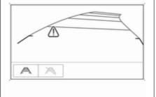
7" Colour Info Display: Activation or deactivation of the visual guiding lines and the warning symbols can be changed via touch buttons in the lower zone of the display.
