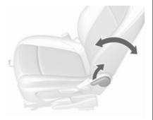
Pull lever, adjust inclination and release lever. Allow the backrest to engage audibly.
