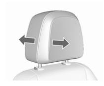
To adjust horizontally, pull the head restraint forwards. It engages in three positions.
