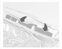
The air intake in front of the windscreen in the engine compartment must be kept clear to allow air intake.
