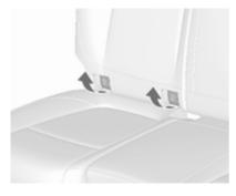
The covers of the guides will swivel backwards automatically when attaching the child restraint system.
