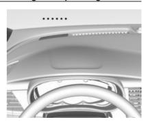
Simultaneously a warning chime sounds. Depress the brake pedal and steer the vehicle, if it is required by the situation.
