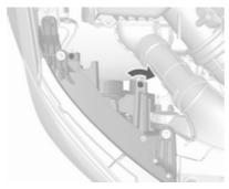
The adjusting screws are located above the headlight.
