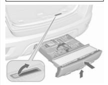
Push the release lever up and hold it. Lift the system slightly and push it into the bumper until it engages.
