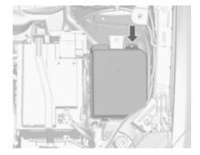
The fuse box is in the engine compartment.
