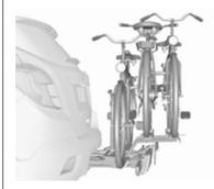
The rear carrier system (Flex-Fix system) allows one bicycle to be attached to an extendable carrier integrated into the vehicle floor. It is possible to attach two further bicycles on an adapter. The transportation of other objects is not permitted.
