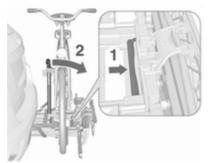
Push the lever (1) to disengage and hold it.
