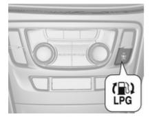
Pressing **LPG** switches between petrol and liquid gas operation as soon as the required parameters (coolant temperature, gas temperature and minimum engine speed) have been reached. The requirements are usually fulfilled after approximately 60 seconds (depending on exterior temperature) and the first firm press on the
