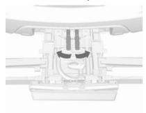
Remove strap and swivel both clamping levers sideways as far as they will go.
