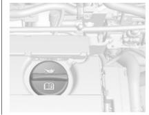
The engine oil filler cap is located on the camshaft cover.
