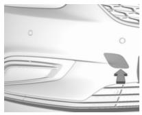
Wrap a cloth around the tip of a flat screwdriver to prevent paint damage. Insert the screwdriver in the slot at the lower part of the cap. Release the cap by carefully moving the screwdriver downwards.
