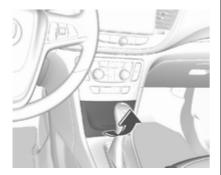
A 12 V power outlet is located in the front console behind the cover. To open, push the button.
