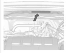
The Vehicle Identification Number is located in the engine compartment.
