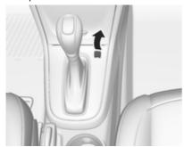
Remove the cap on the console with a thin object such as a screwdriver.
