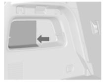
First disengage cover by inserting a screwdriver at the recess. Then disengage cover at the front and upper side. Remove cover.
