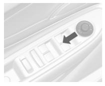
Turn control to **0**, then push the control backwards. Both exterior mirrors will fold in.
