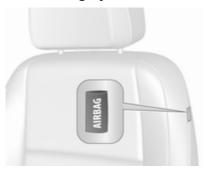
The side airbag system consists of an airbag in each front seat backrest. This can be identified by the word **AIRBAG**.
