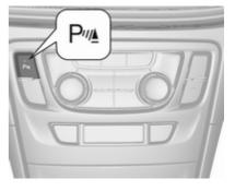
After ignition is switched on, the rear parking assist is activated.
