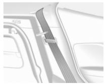
5. Put the seat belts for the outboard seats into the belt guides.
