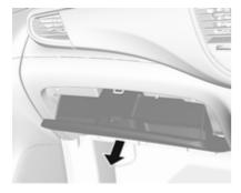
In right-hand drive vehicles, the interior fuse box is located behind a cover in the glovebox on the passenger side. To access the fuses, open the glovebox, then open the cover, fold it down and pull it.
