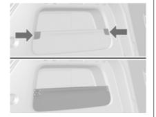
Disengage both covers at the respective outer side by inserting a screwdriver. Remove both covers and unscrew screws. Remove the panel.
