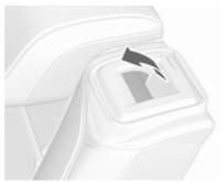
3. Pull the release lever on top of the rear backrest.
