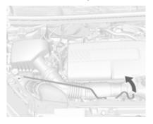
Pull up the support rod lightly from the holder. And then secure it at the left side hook on the bonnet.
