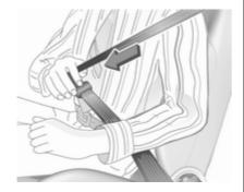
Withdraw the belt from the retractor, guide it untwisted across the body and insert the latch plate into the buckle.
