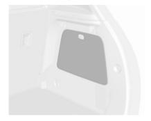
The tools and tyre repair kit are in the right side of the load compartment.
