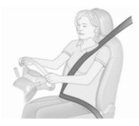
The seat belts are locked during heavy acceleration or deceleration of the vehicle, holding the occupants in the seat position. Thereby the risk of injury is considerably reduced.
