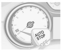
If the vehicle is at a low speed or at a standstill and certain conditions are fulfilled, an Autostop is activated.
