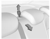
Pull the loop and fold down the backrest of the centre seat.
