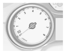
Displays the engine speed.
