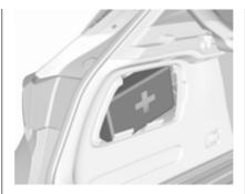
Illustration shows 5-door Hatchback. To open the compartment, disengage cover and open.
