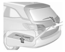
To open the tailgate, press the touchpad switch under the tailgate moulding until the tailgate starts to move. If the vehicle is locked, the electronic key must be outside the vehicle, within a range of approx. one metre of the tailgate.
