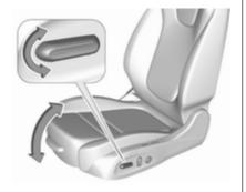
Tilt front of switch upwards/downwards.
