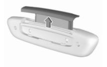
4. To replace fragrance pad, shift cartridge upwards and remove it.
