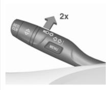
Activate high beam assist by pushing the indicator lever twice. High beam is switched on automatically at a speed above 50 km/h. High beam is switched off at a speed below 35 km/h, but high beam assist remains active.
