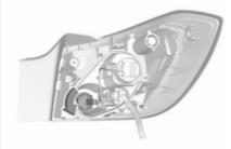
On version with LED tail lights and LED brake lights, only turn signal light bulb can be replaced: remove bulb holder in the light assembly by turning. Replace bulb in the bulb holder.
