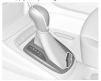
Release the selector lever trim from the centre console. Poke with a finger into the leather socket below the selector lever and push the trim upwards. Rotate trim to the left.
