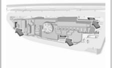
On version with LED tail lights, the position of the retaining lugs is slightly different.
