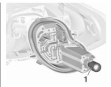
On version with LED tail lights and LED brake lights, only turn signal light bulb (1) can be removed and replaced.
