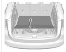
Pull the handle and fold the rear part of the cover forward.
