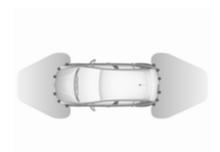
Advanced parking assist is always combined with front-rear parking assist. Both systems use the same sensors in the front and rear bumper.
