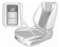
Press at to switch on the back massage function.
