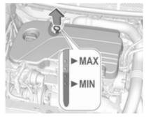
Pull out the dipstick, wipe it clean, reinsert fully, pull out and read the engine oil level.
