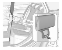
Pull the flap at the tightener on both sides to release the straps. Detach hooks from the eyes.
