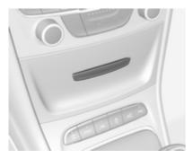
The power connector (PowerFlex Bar) is attached on the instrument panel fuse box cover. A fragrance diffuser (AirWellness) or a phone holder can be attached to the power connector.
