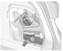
On 5-door hatchback the tyre repair kit is on the right side in the load compartment behind a cover.
