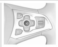
On Uplevel display press **✓** on the steering wheel to confirm a message.
