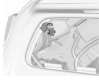
3. Unscrew the plastic securing nut from the inside by hand.
