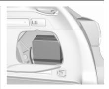
On Sports Tourer the tyre repair kit is in a suitcase on the right side of the load compartment behind a cover. The suitcase is secured with a strap.
