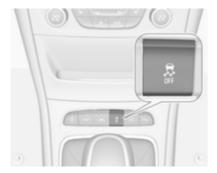
TC can be switched off when spinning of drive wheels is required: press \$\mathcal{B}\$ briefly.
