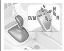
Always move the selector lever in the appropriate direction as far as it will go. Upon release, it automatically returns to the centre position.
