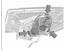
Press the three retaining lugs and remove the bulb carrier from the light assembly.
