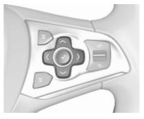
On Uplevel display select **Info** Menu by pressing < on steering wheel. Press  $\checkmark$  to select **Remaining Oil Life** page.
