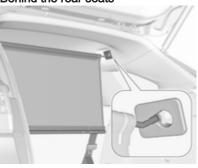
There are installation openings on both sides in the roof frame above the rear seats: suspend and engage rod of net at one side, compress rod and suspend and engage at the other side.
