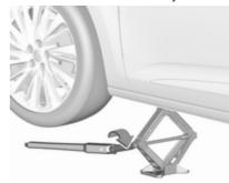
Attach wheel wrench and with the jack correctly aligned rotate wheel wrench until wheel is clear of the ground. Do not raise the jack any further.
