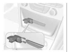
Attach the adapter to the power connector.
