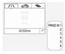
The mode or selected gear is shown in the Driver Information Centre. In automatic mode, the driving programme is indicated by **D**.
