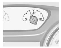
Displays the coolant temperature.
