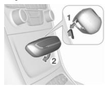
Attach fragrance diffuser to upper side of the power connector (1) and swivel downwards to engage (2).
