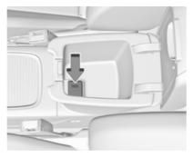
Depending on the infotainment system, one or two USB ports for charging devices are located in between the front seats. These ports have also a data connection to the Infotainment system. For further information, see Infotainment manual.
