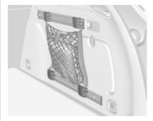
Insert adapters into the required position in the rails. The net pocket can be suspended from the adapters.
