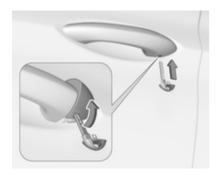
Electronic key: to remove the cap, press button at the back and extract the key blade from the housing. Insert the key into the recess at the bottom of the cap and swivel the key upward. Electronic key system ⋄ 22.
