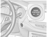
Power button: press Engine Start/Stop and release.
