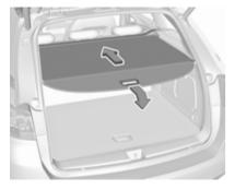
Pull the handle at the end of the roller blind to the rear and downwards. It rolls up automatically.
