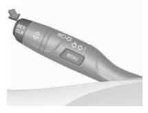
On Midlevel display press **SET/CLR** on the turn signal lever to confirm a message.
