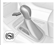
The selector lever is locked in **P** and can only be moved when the ignition is on, the release button on the selector lever is pushed and the brake pedal is applied.
