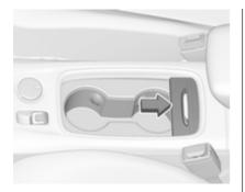
Depending on the version, cupholders are located under a cover in the centre console. Slide cover backwards.
