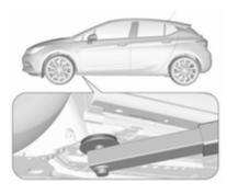
Front arm position of the lifting platform centrically at the underbody.
