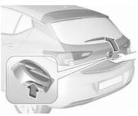
After unlocking, push the touchpad switch under the brand emblem and open the tailgate.
