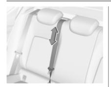
The seat belt of the centre seat could be blocked when the backrest is folded up too quickly. To unlock the retractor, push in the seat belt or pull it out by approx. 20 mm then release.
