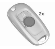
Press no n the radio remote control twice within five seconds.
