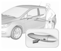
The electronic key must be outside the vehicle, within a range of approx. one metre of the relevant door side.
