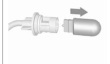
3. Pull bulb from bulb holder and replace it.
