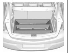
A storage box is located in the load compartment. Remove the cover to gain access to the storage box. Rear floor storage cover ♀ 81.
