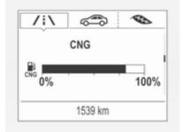
For bi-fuel engines, the Driver Information Centre displays the fuel level for the fuel type which is currently not in operation.
