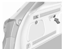
Sports Tourer: A 12 Volt power outlet is located at the left sidewall in the load compartment.
