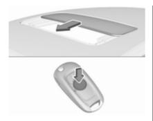
Press and hold to close the sunroof. Release the button to stop the movement.
