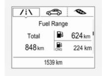
Display of the approximate total fuel range and for each fuel tank (CNG and petrol). A low fuel level in either tank is indicated by **Low** in the respective section.
