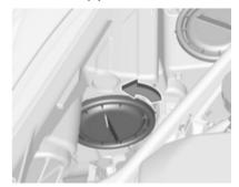
Rotate the cap anticlockwise and remove it.
