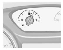
Displays the fuel level or gas content (CNG) in the tank depending on the current operation mode.
