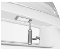
Insert screwdriver in recess of the cover, press to the side and release spring.
