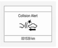
Note that the alert timing sensitivity setting is shared with the following distance setting of the adaptive cruise control. So changing the alert timing sensitivity changes the adaptive cruise control following distance setting.
