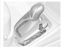
3. Insert a small stick (e.g. a pen or screw driver) into the opening near the selector lever. Push down the the stick vertically and move the selector lever out of **P**. If this position is engaged again, the selector lever will be locked again.
