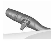
Activate high beam assist by pressing once. High beam is switched on automatically at a speed above 50 km/h. High beam is switched off at a speed below 35 km/h, but high beam assist remains active.
