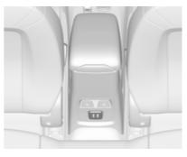
Two USB ports for charging devices only are located in the back of the centre console.
