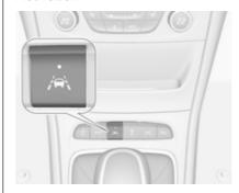
The lane keep assist is activated by pressing A. The LED in the button illuminates to indicate that the system is switched on.
