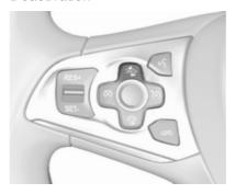
On vehicles with front camera active emergency braking can be deactivated by repeatedly pressing the gap switch & to **Off** setting.
