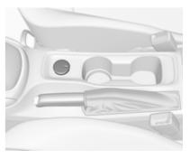
A 12 Volt power outlet is located in the centre console. With ignition off, this power outlet is deactivated.
