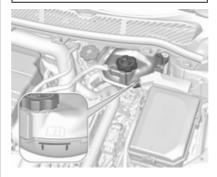
If the cooling system is cold, the coolant level should be above the filling line mark. Top up if the level is low.
