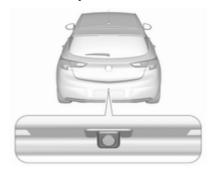
On 5-door hatchback the camera is mounted between the number plate lights.
