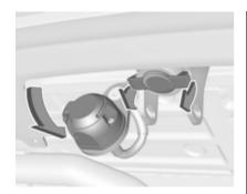
Disengage and fold down the connecting socket. Remove the sealing plug from the opening for the coupling ball bar and stow it.
