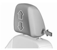
**Height adjustment**Press release button, adjust height, engage.
