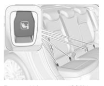
Fasten vehicle-approved ISOFIX child restraint systems to the ISOFIX mounting brackets. Specific vehicle ISOFIX child restraint system positions are marked in the ISOFIX table ♀ 67.
