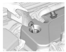
When the engine oil level has dropped to the **MIN** mark, top up engine oil.
