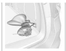
Stow the coupling ball bar in the bag and secure by fixing the strap through the rear right lashing eye. Wrap around twice and tighten the strap to secure the bag.
