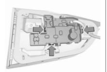
Press the three retaining lugs and remove the bulb carrier from the light assembly.
