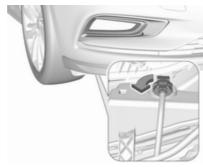
Turn the bulb holder anticlockwise and remove it from the reflector housing.
