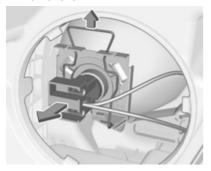
Disengage spring clip from retainer by pulling. Withdraw the bulb holder from the reflector housing.
