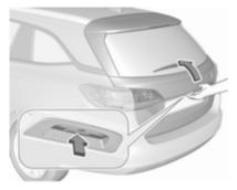
After unlocking, push the touchpad switch under the tailgate moulding and open the tailgate manually. Central locking system ♀ 24.
