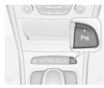
Press parking assist button P<sup>n</sup> to deactivate, the LED in the button extinguishes.
