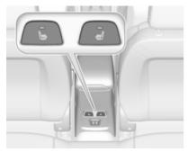
Activate seat heating by pressing #J for the respective rear outer seat. Activation is indicated by the LED in the button.
