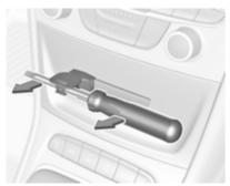
Push the screwdriver through the recess in the adapter. Remove the cover by pulling the screwdriver.
