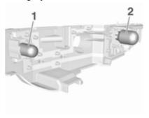
Remove and replace the bulb: Tail light (1)
