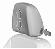
Press release button, adjust height, engage.
