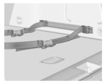
Insert the adapters of the strap set in a rail. Make sure that the belt is not twisted.
