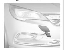
Wrap a cloth around the tip of a flat screwdriver to prevent paint damage. Insert a screwdriver in the slot at the lower part of the cap. Release the cap by carefully moving the screwdriver downwards.
