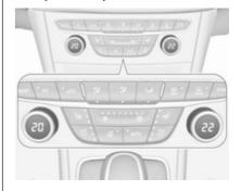
Set temperatures to the desired value. The knob on the passenger side changes the temperature for the passenger side. The knob on the driver's side changes the temperature for the driver's side or for both sides depending on activation of synchronisation **SYNC**.
