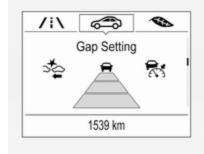
If Adaptive cruise control is active, this page shows the alert sensitivity setting instead of following distance setting. ▷ 189.
