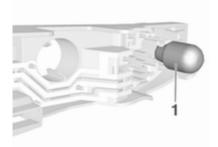
On version with LED tail lights only reverse light bulb (1) can be removed and replaced.
