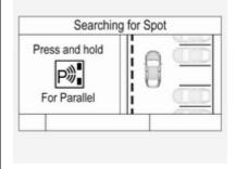
Select parallel or perpendicular parking slot in Driver Information Centre by long press on P#3.
