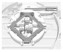
The jack, the towing eye, a strap for securing a damaged wheel and the tools are located in the tool box below the spare wheel. Spare wheel
