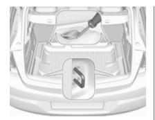
On vehicles equipped with tyre repair kit, the front lashing eyes are located underneath the rear floor cover behind the rear seats. To get access to the lashing eyes, open the perforated parts of the cover by using the screwdriver. Vehicle tools \$\display\$ 256.
