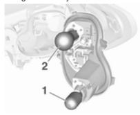
7. Remove and replace the bulbs: Turn signal light (1) Tail light/brake light (2)
