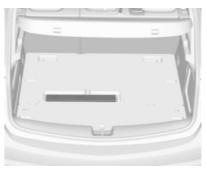
Stow the warning triangle in the recess beneath the rear floor cover.
