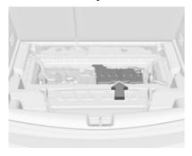
The vehicle battery is located in the load compartment under the rear floor cover behind the rear seats. Rear floor cover ♀ 81.
