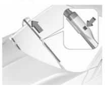
Lift the wiper arm until it stays in the raised position, press button to disengage the wiper blade and remove.
