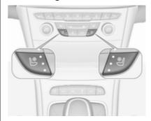
Adjust ventilating to the desired setting by pressing affor the respective seat one or more times. The control indicator in the button indicates the setting.
