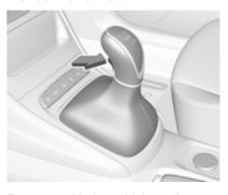
Reverse: with the vehicle stationary, depress clutch pedal and press the release button on the selector lever and engage the gear.
