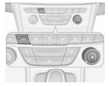
Press to activate air recirculation mode. The LED in the button illuminates to indicate activation.
