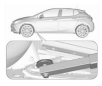
Front arm position of the lifting platform centrically at the underbody.
