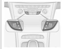
Adjust ventilating to the desired setting by pressing a for the respective seat one or more times. The control indicator in the button indicates the setting.
