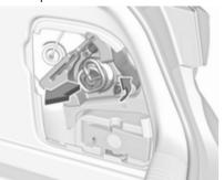
Vehicles with tyre repair kit: To replace bulbs on the right side, first unscrew the plastic nut and take out the insert with the sealant bottle.
