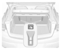
In addition to the ISOFIX mounting brackets, fasten the Top-tether strap to the Top-tether anchors.
