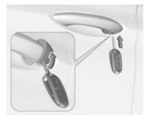
Remote control: to remove the cap, insert the key into the recess at the bottom of the cap and swivel the key upward.
