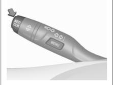
On Midlevel display press **SET/CLR** on the turn signal lever to confirm a message.
