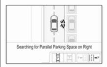
Select parallel or perpendicular parking slot by tapping the respective icon on the display.
