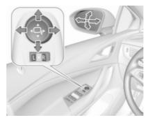
Select the relevant exterior mirror by switching the rocker control to left mirror (L) or right mirror (R). Adjust respective mirror by the four-way control.
