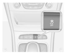
TC can be switched off when spinning of drive wheels is required: press \$ briefly.
