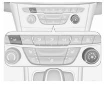
Press **A/C** to switch on cooling. The LED in the button illuminates to indicate activation. Cooling is only functional when the engine is running and climate control fan is switched on.
