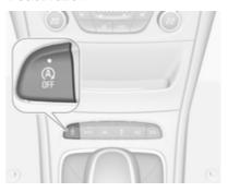
Deactivate the stop-start system manually by pressing . The deactivation is indicated when the LED in the button illuminates.
