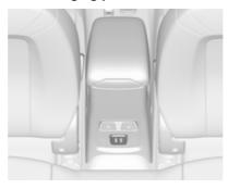
Two USB ports for charging devices only are located in the back of the centre console.
