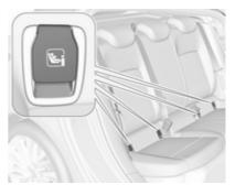
Fasten vehicle-approved ISOFIX child restraint systems to the ISOFIX mounting brackets. Specific vehicle ISOFIX child restraint system positions are marked in the ISOFIX table ♀ 68.
