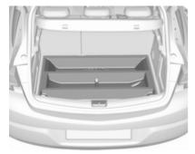
A storage box is located in the load compartment. Remove the cover to gain access to the storage box. Rear floor storage cover ♀ 82.
