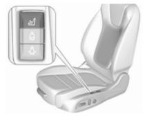
Press at to switch on the back massage function.
