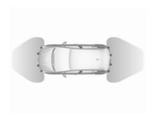
The system has four ultrasonic parking sensors each in the rear and front bumper.
