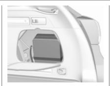
On Sports Tourer the tyre repair kit is in a suitcase on the right side of the load compartment behind a cover. The suitcase is secured with a strap.
