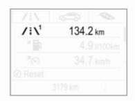
Select /i\ by pressing Menu on the turn signal lever. Turn adjuster wheel on turn signal lever and select /i\1 or /i\2. Each trip odometer page can be reset separately by pressing SET/CLR on the turn signal lever for a few seconds on the respective menu.
