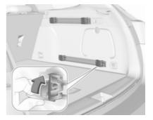
Fold open the handle plate, insert the adapter into the upper and lower groove of the rail and move to the required position. Turn the handle plate upwards to lock the adapter. To remove, turn the handle plate down and move out of the rail.
