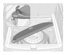
All engine versions, except CNG: The removed roller blind can be stored under the rear floor cover as shown in the illustration. Insert the left side of the rolled up cover first in the front right recess, pull the release lever up and insert the right side in the front left recess.
