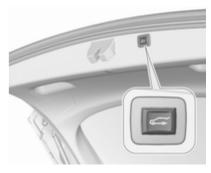
Press and hold the button on the inside of the open tailgate for three seconds.
