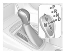
P : park position, wheels are locked, engage only when the vehicle is stationary and the parking brake is applied
