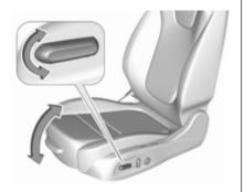
Tilt front of switch upwards/downwards.
