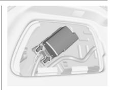
Disengage the fuse box cover and remove it.
