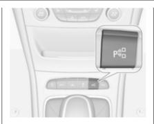
When searching for a parking slot, the system is ready to operate with a short press of ps.
