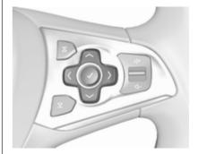
On Uplevel display select **Info** Menu by pressing < on steering wheel. Press  $\checkmark$  to select **Remaining Oil Life** page.
