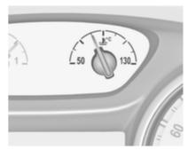
Displays the coolant temperature.
