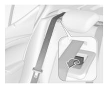
Guide the seat belts of the outer seats through side supports to protect them against damage.
