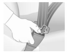
To release belt, press red button on belt buckle.
