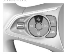
On vehicles with front camera active emergency braking can be deactivated by repeatedly pressing the gap switch so to **Off** setting,
