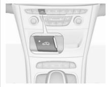
Press to activate the air recirculation mode. The LED in the button illuminates to indicate activation.
