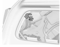
3. Unscrew the plastic securing nut from the inside by hand.
