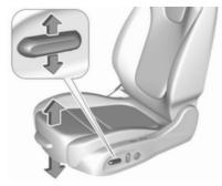
Move switch upwards/downwards.
