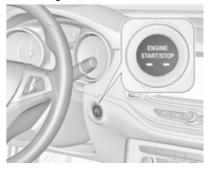
Press Engine Start/Stop and release.
