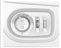
To adapt headlight range to the vehicle load to prevent dazzling: turn thumb wheel ∮○ to required position.
