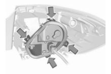
Release the retaining lugs and remove the bulb carrier from the light assembly.
