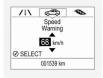
The speed warning function alerts the driver when a set speed is exceeded.
