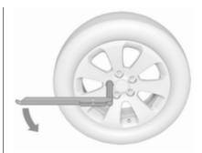
Fold out the wheel wrench and install ensuring that it locates securely and loosen each wheel nut by half a turn.
