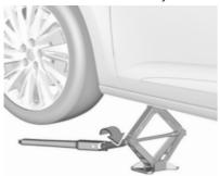
Attach wheel wrench and with the jack correctly aligned rotate wheel wrench until wheel is clear of the ground. Do not raise the jack any further.
