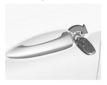
Push inside locking knob of all doors except driver's door or press 🕏 in the driver's door panel. Then close the driver's door and lock it from the outside by turning the key in the lock cylinder. The fuel filler flap and tailgate are possibly not locked.
