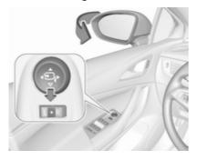
Switch control to ●, then push the control ∇ down. Both exterior mirrors will fold.
