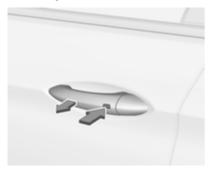
Press the button on a front door handle and pull the handle.
