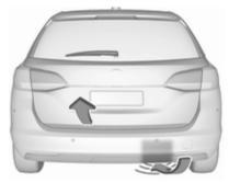
To open or close the tailgate, move the foot below the rear bumper back and forth in the area shown in the illustration. If equipped with parking assist, the area is recognisable below the sensor shown. Do not hold the foot longer or move too slow below the bumper. The electronic key must be outside the vehicle, within a range of approx. one metre of the tailgate.
