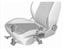
Lever pumping motion up : seat higher down : seat lower
