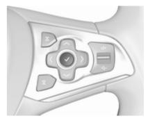
On Uplevel display press  $\checkmark$  on the steering wheel to confirm a message.
