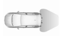
The system has four ultrasonic parking sensors in the rear bumper.
