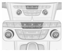
Press the appropriate button for the desired adjustment. The LED in the button illuminates to indicate activation.
