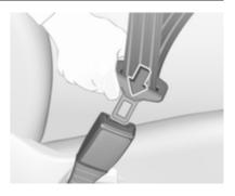
Loose or bulky clothing prevents the belt from fitting snugly. Do not place objects such as handbags or mobile phones between the belt and your body.
