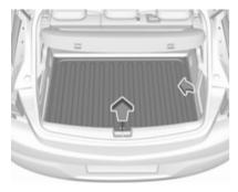
The rear floor cover can be removed. Raise cover at the rear and slightly rotate at one side before removing.
