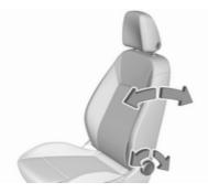
Turn handwheel. Do not lean on backrest when adjusting.
