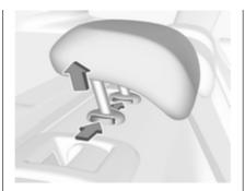
Press both catches, pull the head restraint upwards and remove.
