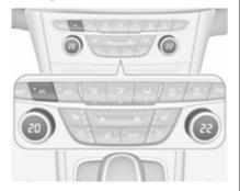
Press **A/C** to switch on cooling. The LED in the button illuminates to indicate activation. Cooling is only functional when the engine is running and climate control fan is switched on.
