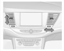
To open the vent, turn the adjuster wheel towards the bigger ■ symbol. Adjust the air amount at the vent outlet by turning the adjuster wheel.
