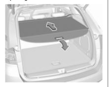
Pull the handle at the end of the roller blind to the rear and downwards. It rolls up automatically.
