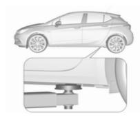
Rear arm position of the lifting platform centrically under the rear recess of the sill.
