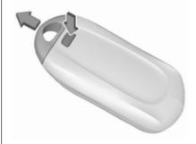
Press button at the back of the electronic key unit and extract the key blade from the housing.
