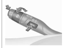
On Midlevel display select the **Settings** Menu by pressing **MENU** on the turn signal lever. Turn the adjuster wheel to select the **Remaining Oil Life** page.
