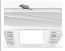
Status LED is integrated in the sensor on top of the instrument panel.
