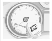
An Autostop is indicated by the needle at the **AUTOSTOP** position in the tachometer.
