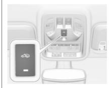
Switch off the monitoring of passenger compartment and vehicle inclination when animals are being left in the vehicle, because of high volume ultrasonic signals or movements triggering the alarm. Also switch off when the vehicle is on a ferry or train.
