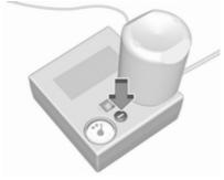
If the prescribed tyre pressure is not obtained within 10 min, remove the tyre repair kit. Move the vehicle one tyre rotation. Reattach the tyre repair kit and continue the filling procedure for 10 min. If the prescribed tyre pressure is still not obtained, the tyre is too badly damaged. Seek the assistance of a workshop.
