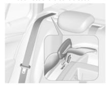
Insert latch plates of the outer seat belts into side holder to protect the belts against damage, see illustration.
