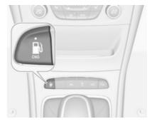
Press • to switch between petrol and natural gas operation.
