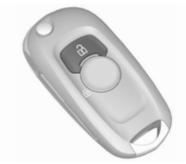
Press to unlock the doors and load compartment. Open the doors by pulling the handles.
