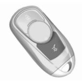
Press so twice to open or close the tailgate. To prevent unintended opening of the tailgate, so must be pressed longer than during locking or unlocking.
