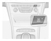
The heating is operated by pressing ...
