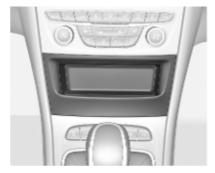
A combined storage and mobile device compartment is located in the instrument panel center stack.
