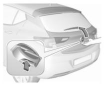
5-door Hatchback: to open the tailgate, push the touchpad switch below the brand emblem.
