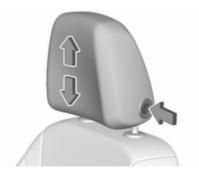
**Height adjustment**Press release button, adjust height, engage.
