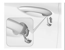
Electronic key: to remove the cap, press button at the back and extract the key blade from the housing. Insert the key into the recess at the bottom of the cap and swivel the key upward. Electronic key system ⋄ 23.
