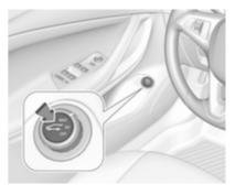
Press on the inside of the driver's door until the tailgate starts to open or close.
