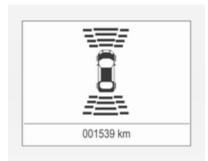
The distance indication can be inhibited by vehicle messages with a higher priority. After dismissing the message distance indication appears again.
