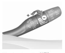
Wiper lever in position **AUTO**. Turn the adjuster wheel to adjust the sensitivity of the rain sensor.
