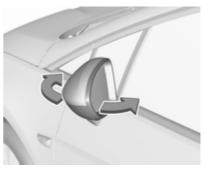
For pedestrian safety, the exterior mirrors will swing out of their normal mounting position if they are struck with sufficient force. Reposition the mirror by applying slight pressure to the mirror housing.
