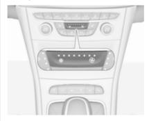
Press left button to decrease or right button to increase fan speed. The fan speed is indicated by the number of LEDs in the button.
