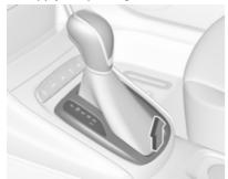
2. Release the selector lever trim from the centre console. Poke with a finger into the leather socket below the selector lever and push the trim upwards. Rotate trim to the left.
