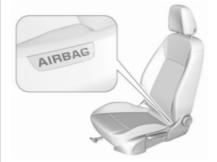
The side airbag system consists of an airbag in each front seat backrest. This can be identified by the word **AIRBAG**.
