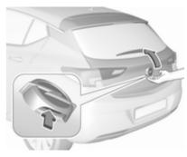
After unlocking, push the touchpad switch under the brand emblem and open the tailgate.
