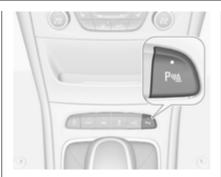
An illuminated LED in the parking assist button  $P^{-1}$  indicates that the system is ready to operate.
