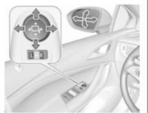
Select the relevant exterior mirror by switching the control to left **(L)** or right **(R)**. Then swivel the control to adjust the mirror.
