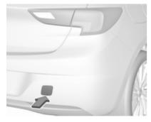
Wrap a cloth around the tip of a flat screwdriver to prevent paint damage. Insert a screwdriver in the slot at the lower bend of the cap. Release the cap by carefully moving the screwdriver downwards.
