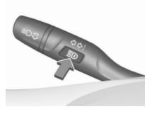
Activate high beam assist by pressing © once. High beam is switched on automatically at a speed above 50 km/h. High beam is switched off at a speed below 35 km/h, but high beam assist remains active.
