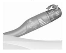
Turn outer cap to activate the rear window wiper:
