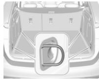
Front and rear lashing eyes are located at the sidewalls. Fold up the lashing eyes to use and fold down when not required.
