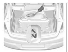
On vehicles equipped with tyre repair kit, the front lashing eyes are located underneath the rear floor cover behind the rear seats. To get access to the lashing eyes, open the perforated parts of the cover by using the screwdriver. Vehicle tools \$\dip\$ 254.
