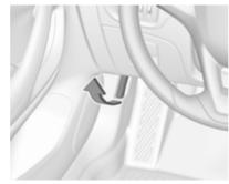
Pull the release lever and return it to its original position.
