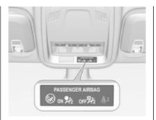
If the control indicator  $\Re_2$  illuminates for approx. 60 seconds after the ignition is switched on, the front passenger airbag system will inflate in the event of a collision.
