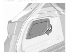
1. Release the cover on the respective side and remove it.
