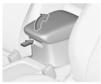
Press button to fold up the armrest. The armrest must be in rearmost position.
