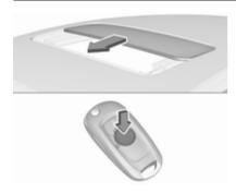
Press and hold to close the sunroof. Release the button to stop the movement.
