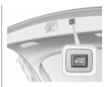
To close, press in the open tailgate until the tailgate starts to move.
