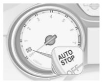
If the vehicle is at a low speed or at a standstill and certain conditions are fulfilled, an Autostop is activated.
