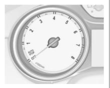
Displays the engine speed.
