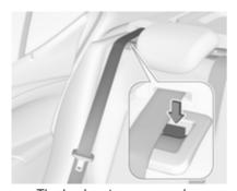
The backrests are properly engaged when the red mark near the release lever is no longer visible.
