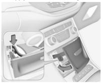
Fold the left side of the cover forwards. Take care that the securing clamp is guided as shown in the illustration.
