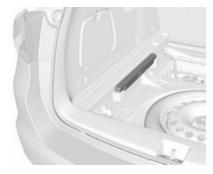
Stow the warning triangle in the recess under the rear floor cover on the right or left side.
