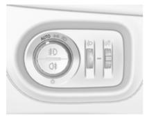
When the automatic light control function is switched on and the engine is running, the system switches between daytime running lights and headlights automatically depending on the external lighting conditions and information given by the rain sensor system.
