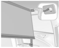
There are installation openings on both sides in the roof frame above the front seats: suspend and engage rod of net at one side, compress rod and suspend and engage at the other side.
