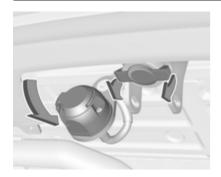
Disengage and fold down the connecting socket. Remove the sealing plug from the opening for the coupling ball bar and stow it.
