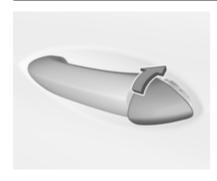
After locking, cover the lock cylinder with the cap: insert the cap with the lower side in the recesses, swivel and push the cap until it engages at the upper side.
