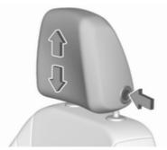
Press release button, adjust height, engage.
