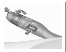
Press **MENU** to switch between the main menus or to return from a submenu to the next higher menu level.
