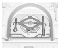
The jack, the towing eye and the tools are located in the tool box below the spare wheel. Spare wheel ♀ 266.
