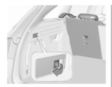
Alternatively fold seat backrests from the load compartment: pull switch on left or right sidewall of the load compartment to fold the corresponding part of the rear seat backrest.
