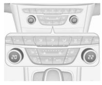
Set temperatures to the desired value. The knob on the passenger side changes the temperature for the passenger side. The knob on the driver's side changes the temperature for the driver's side or for both sides depending on activation of synchronisation **SYNC**.
