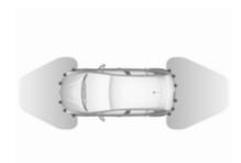
Advanced parking assist is always combined with front-rear parking assist. Both systems use the same sensors in the front and rear bumper.
