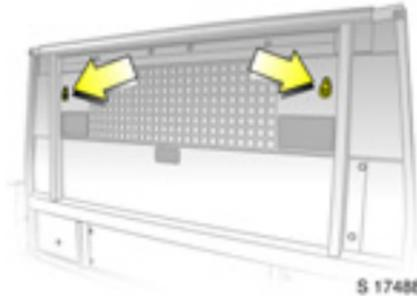
The two additional lashing points on the bulkhead should also be used to secure the load whenever possible.
