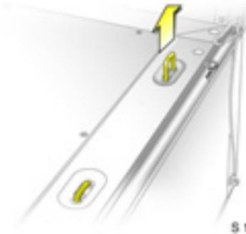
Pull up the lashing eyes as required. Secure heavy objects with lashing straps attached to the lashing points. If heavy loads slip when the vehicle is braked heavily or driven around a bend, the handling of the vehicle may change.
