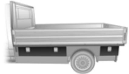
Certain models feature five lockable underfloor storage compartments. For security, these can be locked with the key provided.
