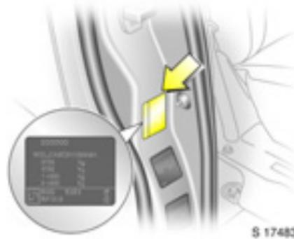
The Gross Vehicle Weight and Gross Train Weight can be found on the vehicle identification plate, which is located on the right-hand door pillar.
