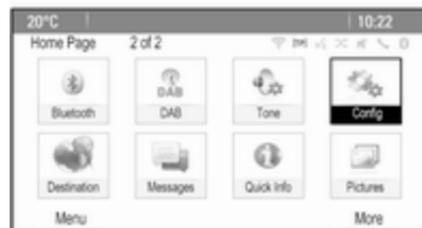
Press the multifunction knob (Navi 950 / Navi 650: press the outer ring) to display the second **Home Page** with further applications.
