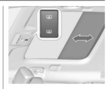
Press or gently to the first detent: the sunblind is opened or closed as long as the switch is operated.
