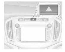
Operated by pressing <u>A</u>. In the event of an accident with airbag deployment the hazard warning flashers are activated automatically.
