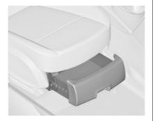
Press button in the recess and pull out drawer. Maximum load: 3 kg. To close, push in and engage.
