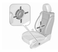
Adjust lumbar support using the fourway switch to suit personal requirements.
