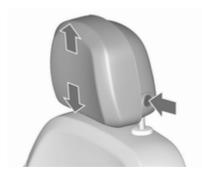
**Height adjustment**Press release button, adjust height, engage.
