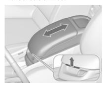
The armrest can be moved in a centre console. Pull the handle to slide the armrest.
