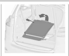
Pull up the seat by the upper loop, fold out and allow seat to engage in upright position.
