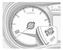
If the vehicle is at a low speed or at a standstill and certain conditions are fulfilled, activate an Autostop as follows:
