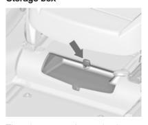
There is a storage box under the passenger's seat. Slide the rollo to open or close the box. Maximum load: 1.5 kg.
