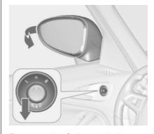
Turn control to **0**, then push the control down. Both exterior mirrors will fold.
