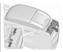
Press fastenings inward and fold down locking mechanism at the rear end of the armrest.
