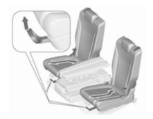
In lounge position, the outer seats are additionally movable in transverse direction when the centre seat backrest is folded to an armrest.
