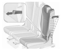
Raise backrest to vertical position. Adjust inclination by pulling the loop. Ensure that all positions are engaged correctly.
