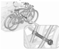
Use the short accessory mounting bracket to attach the fourth bicycle. The bracket must be fixed between the frames of the third and fourth bicycle.
