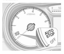
An Autostop is indicated by the needle at the **AUTOSTOP** position in the tachometer.
