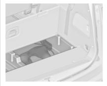
On version without third seat row, there are storage boxes under the floor cover. Lift up the cover to open.
