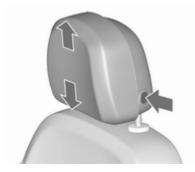
Press release button, adjust height, engage.
