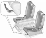
Pull the handle under each outer seat and slide seats to forward position.
