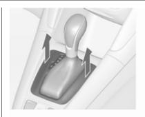
Release the selector lever trim from the centre console at the front, fold it upwards and rotate it to the left.
