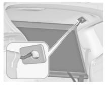
There are installation openings on both sides in the roof frame above second row seats: suspend and engage rod of net at one side, compress rod and suspend and engage at the other side.
