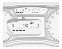
Displays the fuel level or gas content (LPG or CNG) in the tank depending on the operation mode.
