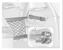
Insert adapters into the required position in the rails. Stick together the halves of the net rods.
