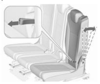
Pull the loop, adjust inclination, release strap and allow backrest to engage.
