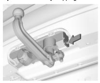
Attach breakaway stopping cable to eye.
