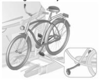
Rotate the pedals into position as shown in the illustration and put the bicycle on the foremost wheel recess.
