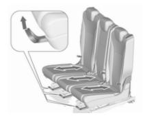
In normal position, the three seats of the second seat row can be individually moved in longitudinal direction.
