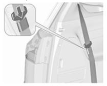
Insert the latch plate of the seat belt on each side into the pocket that is mounted at the belt.
