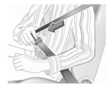
Withdraw the belt from the retractor, guide it untwisted across the body and insert the latch plate into the buckle. Tighten the lap belt regularly whilst driving by pulling the shoulder belt
