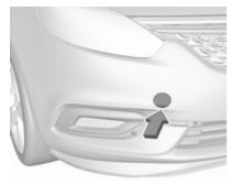
Disengage cap at bottom and remove downwards.
