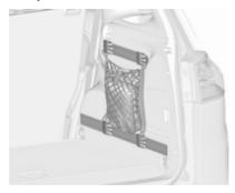
Insert adapters into the required position in the rails. The net pocket can be suspended from the adapters.
