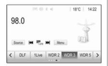
Briefly press or touch  $\blacktriangleleft$  or  $\blacktriangleright$  on the control panel or on the screen to play the previous or next station in the station memory.
