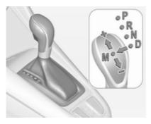
P: park positionR: reverseN: neutral modeD: automatic modeM: manual mode
