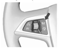
Press % to switch on adaptive cruise control. The control indicator (5) illuminates white. Additionally % appears in the Driver Information Centre.
