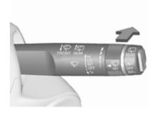
Push lever. Washer fluid is sprayed onto the rear window and the wiper wipes a few times.
