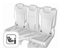
Fasten vehicle-approved ISOFIX child restraint systems to the ISOFIX brackets. Specific vehicle ISOFIX child restraint system positions are marked in the ISOFIX table ♀ 63.
