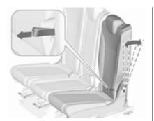
Pull the loop, adjust inclination, release strap and allow backrest to engage.
