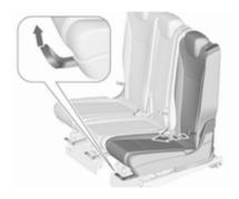
When using ISOFIX fastened child restraint systems on the second seat row, we recommend to adjust the accordant outer seat in third notch from rear end position, regarding to base seats. Lounge seat, if equipped, must be in normal position ♀ 44.
