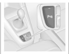
An illuminated LED in the parking assist button  $P^{-1}$  indicates that the system is ready to operate.
