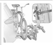
Guide the strap attached to the adapter underneath the lever to fold back the rear carrier system. Fasten the strap.
