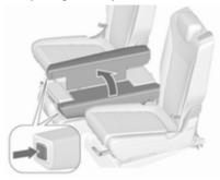
Push the left and right buttons near the centre head restraint and fold in the outer backrest
