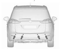
The system has four ultrasonic parking sensors each in the rear and front bumper.
