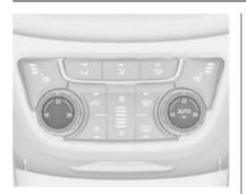
If the minimum temperature **Lo** is set, the climate control system runs at maximum cooling, if cooling **\$\pi\$** is switched on.
