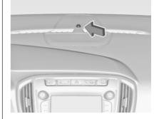
Status LED is integrated into the sensor on top of the instrument panel.
