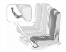
Pull handle, slide seat, release handle and allow seat to engage.
