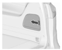
To open, release cover in side trim panel and remove.
