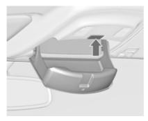
Press button to open storage box. The box may be loaded with max. 0.2 kg.
