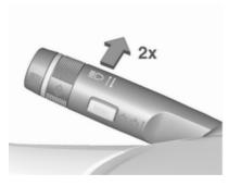
The high beam assist is activated by pushing the indicator lever twice with a speed above 40 km/h.
