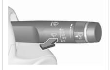
Pull lever. Washer fluid is sprayed onto the windscreen and the wiper wipes a few times.
