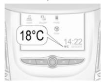
A drop in temperature is indicated immediately and a rise in temperature after a time delay.
