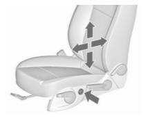
Adjust lumbar support using the fourway switch to suit personal requirements.
