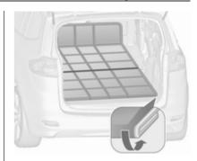
Fold the overlaying rear part under the mat before closing the tailgate.
