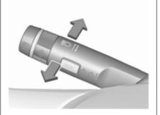
headlight flash: pull lever high beam: push lever
