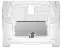
Pull out the mat a little to protect load compartment sill when loading heavy objects. Raise up the overlaying part of the mat before closing the tailgate.
