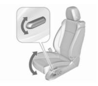
Move front of switch upwards/downwards.
