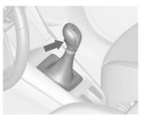
Reverse: with the vehicle stationary, depress clutch pedal, press the release button on the selector lever and engage the gear.
