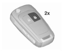
Press no n the radio remote control twice within 5 seconds.
