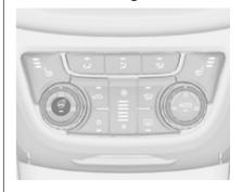
Activate heating by pressing **a**. Activation is indicated by the LED in the button.
