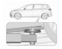
Rear arm position of the lifting platform centrically under the recess of the sill.
