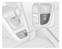
The lane departure warning system is activated by pressing \u00ed . The illuminated LED in the button indicates that the system is switched on. When the control indicator \u00ed in the instrument cluster illuminates green, the system is ready to operate.
