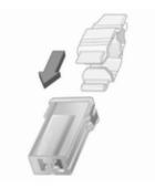
Place the fuse extractor on the various types of fuse from the top or side, and withdraw fuse.
