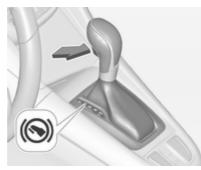
The selector lever is locked in **P** and can only be moved when the ignition is on, the release button on the selector lever is pushed and the brake pedal is applied.
