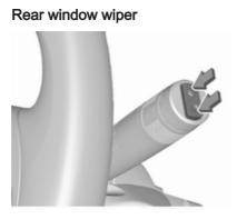
Press the rocker switch to activate the rear window wiper:
