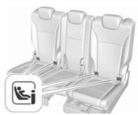
Fasten vehicle-approved ISOFIX child restraint systems to the ISOFIX brackets. Specific vehicle ISOFIX child restraint system positions are marked in the ISOFIX table ⇔ 59.
