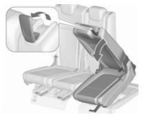
**Folding back easy entry** First move seat to desired position and then raise backrest.
