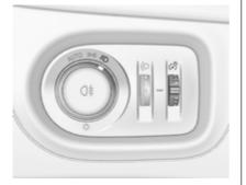
Brightness of the following lights can be adjusted when the exterior lights are on:
