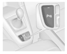
Manual deactivation is also possible by pressing the parking assist button  $\mathbf{P}^{m} \mathbf{A}$ .
