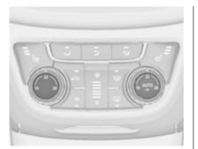
If the minimum temperature **Lo** is set, the climate control system runs at maximum cooling, if cooling \$\$ is switched on.
