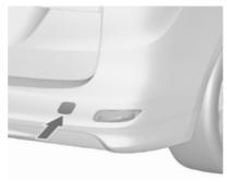
Wrap a cloth around the tip of a flat screwdriver to prevent paint damage. Insert a screwdriver in the slot at the lower edge of the cap. Release the cap by carefully moving the screwdriver downwards. To prevent damage it is recommended to place a cloth between the screwdriver and the frame.
