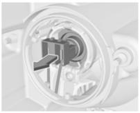
2. Withdraw the bulb holder from the reflector housing.
