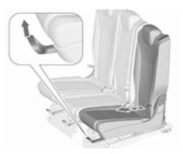
When using ISOFIX fastened child restraint systems on the second seat row, we recommend to adjust the accordant outer seat in third notch from rear end position, regarding to base seats. Lounge seat, if equipped, must be in normal position  $\diamondsuit$  42.
