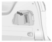
The funnel is located on the righthand side storage compartment in the load compartment.
