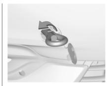
Screw in the towing eye as far as it will go until it stops in a horizontal position.
