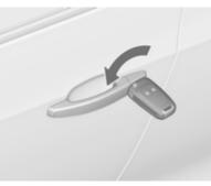
Manually unlock the driver's door by turning the key in the lock. Switch on the ignition and press T to unlock all doors, load compartment and fuel filler flap. By switching on the ignition, the anti-theft locking system is deactivated.
