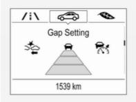
If Adaptive cruise control is active, this page shows the alert sensitivity setting instead of following distance setting. ♀ 206.
