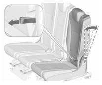
Raise backrest to vertical position. Adjust inclination by pulling the loop. Ensure that all positions are engaged correctly.
