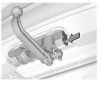
Attach breakaway stopping cable to eye.
