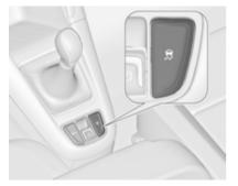
TC can be switched off when spinning of drive wheels is required: press  $\mathfrak{B}$  briefly.
