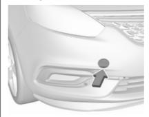
Disengage cap at bottom and remove downwards.
