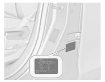
The identification plate is located on the front left or right door frame.
