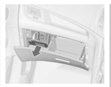
In right-hand drive vehicles, the fuse box is located behind a cover in the glovebox. Open the glovebox, then open the cover and fold it down.
