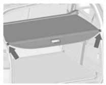
Pull the load compartment cover towards the rear using the handle and engage it in the retainers at the sides. Opening
