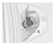
2. Turn the bulb holder anticlockwise and remove it from the reflector.
