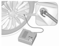
If tyre pressure is more than 1.3 bar, set it to the correct value. Repeat the procedure until there is no more loss of pressure. If the tyre pressure has fallen below 1.3 bar, the vehicle must not be used. Seek the assistance of a workshop.
