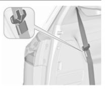
Insert the latch plate of the seat belt on each side into the pocket that is mounted at the belt.
