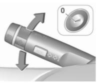
When the vehicle is parked, the parking lights on one side can be activated:
