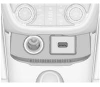
A 12 Volt power outlet is located in the front console. Fold the cover downwards.
