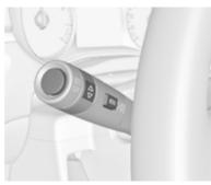
Select Vehicle Information Menu 🖘 by pressing **MENU** on the turn signal lever. Turn the adjuster wheel to select **Remaining Oil Life**.
