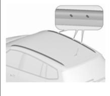
Fasten the roof rack in the area of the holes.
