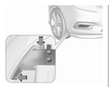
1. Remove the outer screws of the cover, as shown in the illustration.
