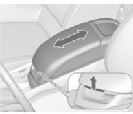
The armrest can be moved in a centre console. Pull the handle to slide the armrest.
