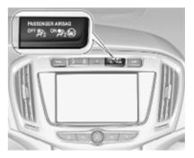
If the control indicator ON **X**<sup>2</sup> illuminates for approx. 60 seconds after the ignition is switched on, the front passenger airbag system will inflate in the event of a collision.
