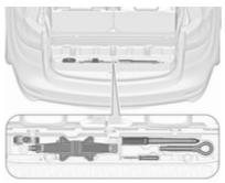
Some tools, the towing eye and (only on vehicles with spare wheel) the vehicle jacking equipment are placed in the rear storage in the load compartment floor.
