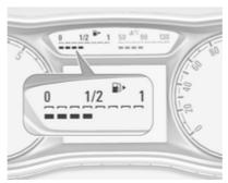
Displays the fuel level in the tank depending on the operation mode.
