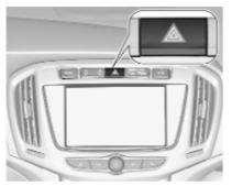
Operated by pressing ▲. In the event of an accident with airbag deployment the hazard warning flashers are activated automatically.
