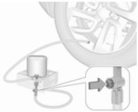
Depending on version the button can be located on the air hose.
