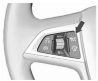
Press % to switch on adaptive cruise control. The control indicator  $\Im$  illuminates white. Additionally % appears in the Driver Information Centre.
