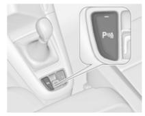
An illuminated LED in the parking assist button  $\mathbf{P}$ <sup>w</sup> indicates that the system is ready to operate.
