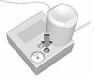
Drain excess tyre pressure with the button over the pressure indicator.
