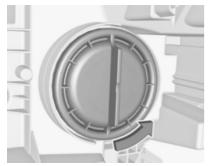
1. Rotate cap anticlockwise and remove it.
