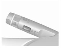
Press **MENU** to switch between the menus or to return from a submenu to the next higher menu level.
