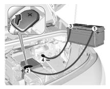
Open the positive terminal protection caps of both vehicle batteries.
