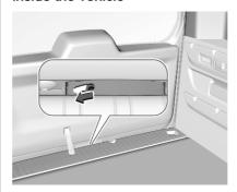
An access hole between the door and the floor enables the tailgate latch to be released using a suitable tool. Push lever to the left to unlock and open the tailgate.
