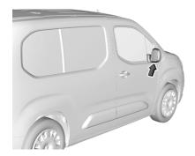
The camera is mounted at the bottom of the exterior mirror on the passenger side.
