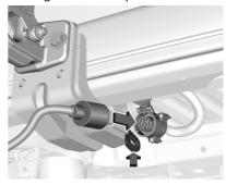
Connect the trailer plug to the socket and attach the breakaway stopping cable to the eye on the carrier.
