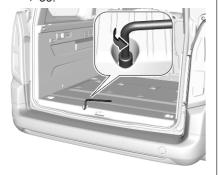
Fit the wheel wrench on one hexagon bolt. Turn it anticlockwise until the spare wheel holder is low enough allow the catch to be unhooked.
