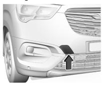
Wrap a cloth around the tip of a flat screwdriver to prevent paint damage. Insert the screwdriver in the slot at the lower part of the cap. Release the cap carefully.
