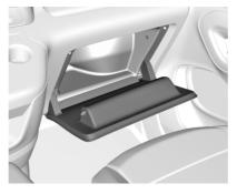
To open the glovebox pull the handle.
