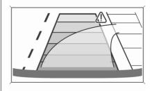
Trajectory lane of the vehicle is shown in accordance with the steering angle.
