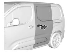
After unlocking, pull the outside door handle and slide the door towards the rear beyond the point of resistance.
