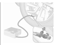
16. Continue driving immediately so that sealant is evenly distributed in the tyre. After driving approx. 5 km but no more than ten minutes, stop and check tyre pressure. Screw compressor air hose directly onto tyre valve when doing this. Fill tyre as described before. Drain excess tyre pressure with the button on the air hose.
