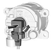
Turn the bulb socket anticlockwise and remove it from the light assembly.
