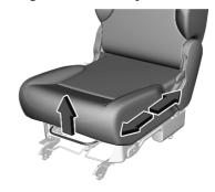
Pull the handle, slide the seat, then release the handle. Try to move the seat back and forth to ensure that the seat is locked in place.
