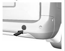
Wrap a cloth around the tip of a flat screwdriver to prevent paint damage. Insert the screwdriver in the slot at the lower part of the cap. Release the cap carefully.
