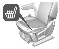
Activate seat heating by pressing ## for the respective front seat.
