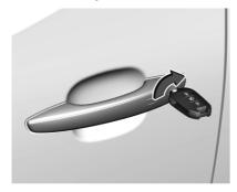
Manually lock the doors, tailgate and fuel filler flap by inserting and turning the key in the lock cylinder of the driver's door.
