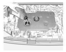
When the engine oil level has dropped to the **MIN** mark, top up the engine oil.
