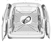
Lashing eyes may be located on the vehicle floor and / or in the sidewall. The number and location of the lashing eyes may vary depending on the vehicle.
