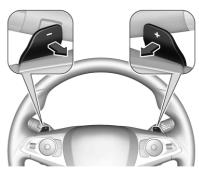
Pull steering wheel paddles to select gears manually.
