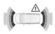
Additionally, the distance to rear and front obstacles is displayed by changing distance lines in the Info Display \$\phi\$ 113.
