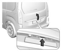
After unlocking, press the tailgate button and open the tailgate.
