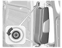
Unscrew and remove the two screws.
