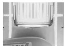
The camera records the vehicle's surroundings during the manoeuvre in order to reconstruct a view from above the rear of the vehicle in its near surroundings, allowing the vehicle to be manoeuvred around obstacles nearby. This view is available with **AUTO Mode** or in the view selection menu.
