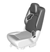
2. Pull the lever and fold down the backrest onto the seat cushion.
