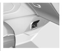
A 230 V power outlet may be located on the lower side of the centre console in the front passenger compartment.
