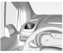
Cup holders are located at the sides of the instrument panel.
