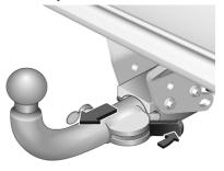
Move the lever of the coupling ball bar to the rear position. Remove the coupling ball bar by pulling it.
