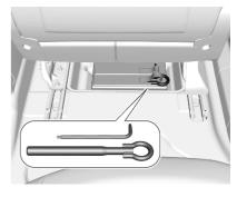
The towing eye and the tools are located in the stowage compartment underneath the right front seat.
