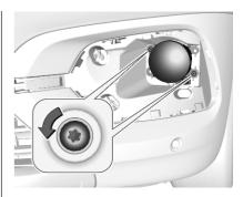
Unscrew and remove the two screws and remove the light assembly to the front.
