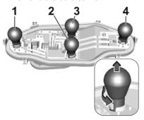
Push the bulb slightly down, turn it and remove it from the bulb carrier. Replace the bulb: Tail light / brake light (1)
