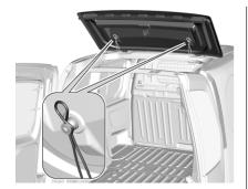
Move past the point of resistance to lock the ladder flap with the props.
