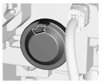
1. Remove the protective cover by pulling.
