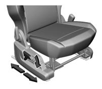
Depending on version, pull the lever of the passenger seat and slide the seat, then release the handle.
