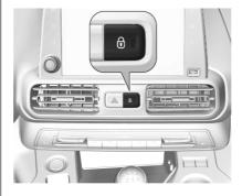
This function can be activated or deactivated at any time. With the ignition on, press \( \text{\text{d}} \) until an audible signal starts and a corresponding message is displayed.
