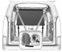
There are installation openings on both sides in the roof frame above the front seats. Open the covers and suspend and engage rod of net at one side, compress rod and suspend and engage at the other side.
