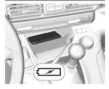
The portable device to be charged must be compatible with the Qi standard, either by design or by using a compatible holder or shell. The charging zone is identified by the Qi symbol.
