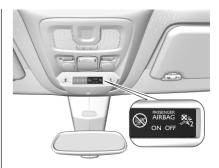
If the control indicator @ illuminates for approx. 60 seconds after the ignition is switched on, the front passenger airbag system will inflate in the event of a collision.
