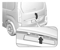
After unlocking, press the middle tailgate button and open the tailgate.
