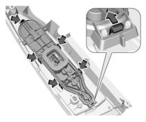
Press the retaining lug backwards, pull the bulb carrier and disengage the remaining retaining lugs.
