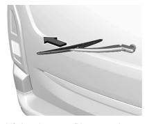
Lift the wiper arm. Disengage the wiper blade as shown in the illustration and remove.
