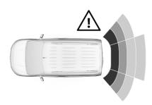
Additionally, the distance to rear obstacles is displayed by changing distance lines in the Info Display
