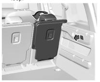
Alternatively fold seat backrests from the load compartment: pull lever on left or right sidewall of the load compartment to fold the rear seat backrests.
