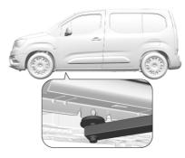
The front arm position of the lifting platform is centrically under the relevant vehicle jacking point.
