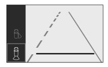
The horizontal line represents a distance of about 4 m beyond the edge of vehicle's rear bumper.
