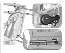
Move the partition and lock the four locking devices on the top and the bottom.
