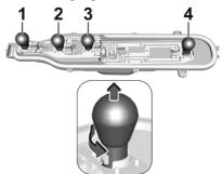
5. Push the bulb slightly down, turn it and remove it from the bulb carrier. Replace the bulb:
