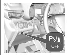
Graphic Info Display: The system is ready to operate when the LED in the parking assist button is not illuminated.
