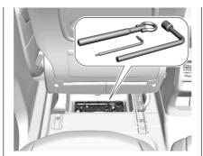
The towing eye and the tools are located in the stowage compartment underneath the left front seat.
