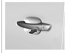
Press with a finger or thumb on one of the door handles (at the markings) or press the tailgate button.
