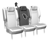
Depending on version, fold down the centre backrest by pulling the loop.
