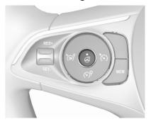
Activate heating by pressing **8**. Activation is indicated by the LED in the button.
