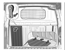
Turn the locking device upwards. Put the hinges of the flap in their housing, lift the flap and close the locking device.
