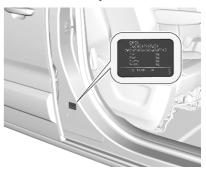
The identification plate is located on the front left or right door frame.
