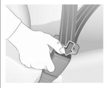
To release seat belt, press red button on belt buckle.
