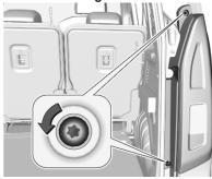
Unscrew and remove the two screws.
