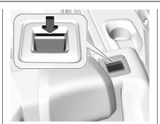
The backrests are properly engaged when the red mark near the release lever is no longer visible.
