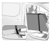
Pass the strap of the cover around the head restraint. Tension the strap by pulling at the loose end.
