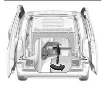
The doors are retained in the 90° position by locking stays. To open the doors to 180°, push the latch and swing open to the desired position.
