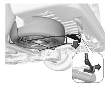
3. Lift the spare wheel holder and unhook the catch.
