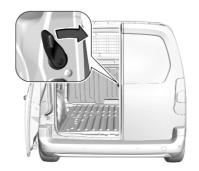
The right hand rear door is released using the lever.
