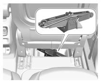
The jack is located in the stowage compartment underneath the right front seat.
