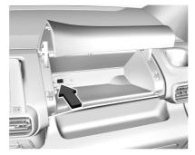
A USB port may be located within the compartment located above the glovebox.
