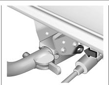
8. Attach the breakaway stopping cable to the eye on the carrier.
