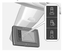
Select the standard rear view or passenger side view by pressing the "IIII on the bottom side.
