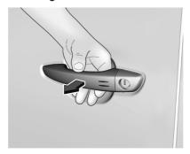
Pass a hand behind the door handle of one of the front doors or the rear door to unlock the vehicle or press the middle tailgate button.
