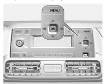
Press **MENU** to open the menu page. Use four-way button to operate the display: Select Personalisation-configuration,
