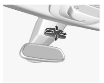
A child surveillance mirror allows to observe the rear seats. The mirror can be adjusted.
