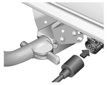
7. Connect the trailer plug to the socket.
