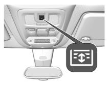
Press 👪 at the rear: the sunblind is opened as long as the switch is operated.
