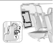
2. Release the locking device of the flap and open the flap.
