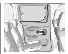
To open from inside push the handle and slide the door towards the rear beyond the point of resistance.
