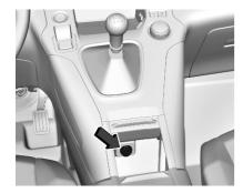
A 12 V power outlet is located behind the storage cover. Push cover upwards to open.
