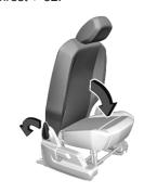
Push lever, fold backrest fully forwards and release the lever. Then push the backrest down further until it is completely flat.
