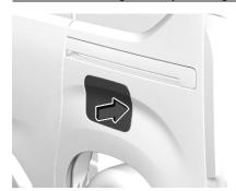
If the vehicle is equipped with an electronic key system, the fuel filler flap can only be opened if the vehicle is unlocked. Depending on the version, release the fuel filler flap by pushing the flap or pulling at the right bottom corner.
