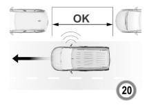
When a free slot is detected, a visual feedback on the Info Display and a first acoustic signal is given. Drive slowly forwards. When the second acoustic signal is given, stop the vehicle, select reverse gear, release the steering wheel and start moving slowly. A visual feedback is given on the Info Display.
