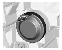
1. Remove the protective cover by pulling.
