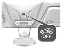
Switch off the monitoring of passenger compartment when animals are being left in the vehicle, because of high volume ultrasonic signals or movements triggering the alarm. Also switch off when the vehicle is on a ferry or train.
