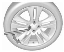
Attach the wheel wrench and loosen each wheel bolt by half a turn.
