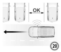
When a free slot is detected, a visual feedback on the Info Display and an acoustic signal is given. Stop the
