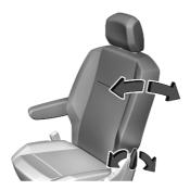
Push the lever and adjust the inclination. Do not lean on backrest when adjusting.
