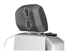
Press release button, adjust height, engage.
