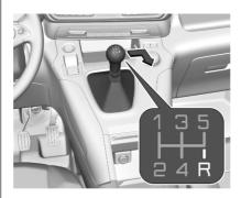
To engage reverse on 5-speed transmission, depress the clutch pedal and move the selector lever to the right and rear.
