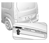
With the electronic key outside the vehicle and within a range of approx. one metre of the tailgate, press the left tailgate button to lock the vehicle. Central locking system ⋄ 26.
