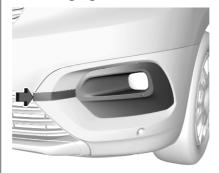
Wrap a cloth around the tip of a flat screwdriver to prevent paint damage. Insert the screwdriver in the recess at the edge of the cover. Release the cover by levering it out carefully.
