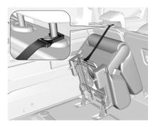
Secure the folded seat in the upright position by attaching the strap to one of the pillars of the head restraint in front of the folded seat.
