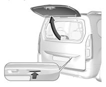
After unlocking, press the right tailgate button and open the rear window.
