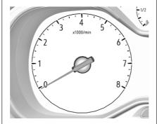
Displays the engine speed.
