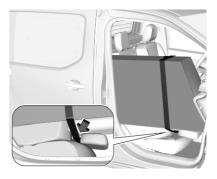
Pass the strap of the cover around the head restraint. Tension the strap by pulling at the loose end.
