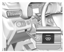
Heating is operated by pressing w. LED in button illuminates.
