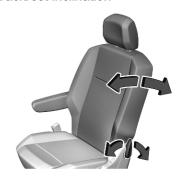
Push the lever, adjust inclination and release the lever. Do not lean on backrest when adjusting.
