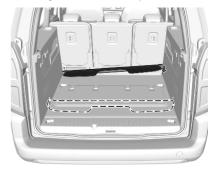
If the load compartment cover is not used, stow it in the load compartment. It can be stowed behind the second or third row seats.
