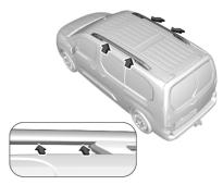
Mounting points are located at the bottom of the roof railing.
