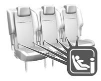
Fasten vehicle-approved ISOFIX child restraint systems to the ISOFIX brackets. Specific vehicle ISOFIX child restraint system positions are marked in the ISOFIX table ♦ 69.
