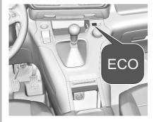
This mode adjusts the settings of the systems for a more economic fuel consumption, e.g. by optimising the automatic transmission shift points and adapting the sensitivity of the accelerator pedal.
