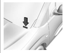
The Vehicle Identification Number may be embossed on the instrument panel, visible through the windscreen.
