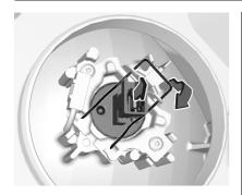
Disengage the spring clip from the retainer by moving it to the righthand side. Swivel the spring clip downwards.
