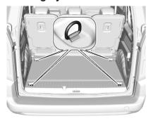
The lashing eyes are designed to secure items against slippage, e.g. using lashing straps or luggage net.
