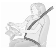
Pull out the seat belt and fasten in seat belt buckle. The seat belt must not be twisted and must fit close against the body. The backrest must not be tilted back too far (maximum approx. 25°).
