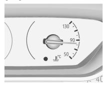
Displays the coolant temperature.
