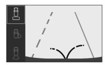
Additionally the opening radius of the rear doors are shown in the rear view display.
