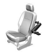
To remove the armrest fold it up, push and turn it to the position shown in the picture.
