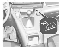
At speeds below approx. 50 km/h, press \*\*. The system can also be activated when the vehicle is stationary with the engine running. The control indicator \*\*. in the instrument cluster is illuminated in green to show the system is activated.
