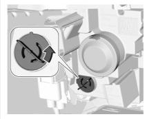
Rotate the bulb socket anticlockwise to disengage and withdraw from the reflector.
