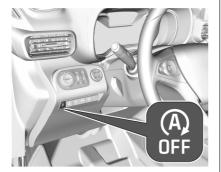
Deactivate the stop-start system manually by pressing . The deactivation is indicated when the LED in the button illuminates.
