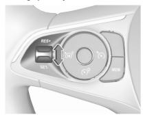
Accelerate to the desired speed and press thumb wheel once briefly to RES/+ or SET/-. The current speed is stored and maintained. Accelerator pedal can be released.
