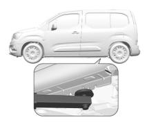
The rear arm position of the lifting platform is centrically under the relevant vehicle jacking point.
