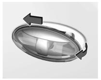
1. Slide the lamp housing forward and remove it at the back.
