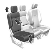
Fold down the outer backrest by pulling the loop. Swing the backrest forwards until the seat is lowered on the vehicle floor.
