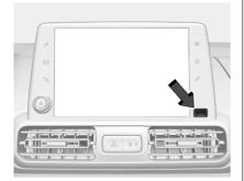
A USB port is located in the instrument panel next to the Info Display.
