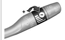
Turn the adjuster wheel to adjust the sensitivity.
