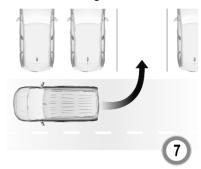
Move forwards and backwards as instructed by observing the warnings of the parking assist and paying attention to the acoustic signals until the end of manoeuvre is indicated. When finished, Pe extinguishes in the instrument cluster.
