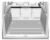
Open the load compartment cover. Compress the load compartment cover at one side and lift it up. Remove the load compartment cover.
