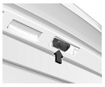
1. Insert a screwdriver in the recess of the cover and remove it.
