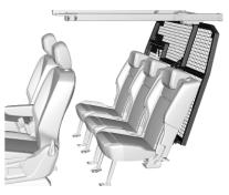
There is a flap in the partition which can be opened to accommodate long objects. A protective cover is provided in the vehicle to assure safe transportation.
