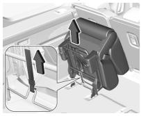
Pull the loop to disengage the locks and remove the seat assembly from the floor anchor points.
