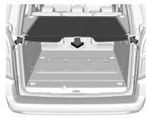
Pull the load compartment cover towards the rear and engage it in the side brackets.
