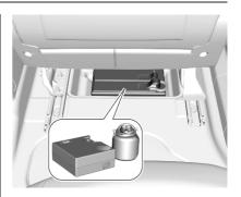
The tyre repair kit is located in the storage compartment underneath the passenger front seat.
