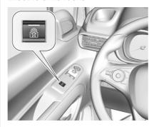
Depending on version, the \( \mathbb{L} \) button may be located in the driver's door or below the light switch.
