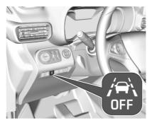
If the system is activated, the LED in the button # is not illuminated. To activate the system when the system is deactivated, press #.
