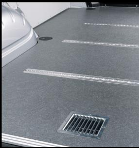
**Protective side wall** and floor cladding, complete with load-securing devices, are ideal for delivery services.
