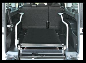
The Opel Combo F-Style 2 LWB guarantees great versatility thanks to the new Free Access Ramp, which is available as an option. The Free Access Ramp can be folded inside the vehicle, when no wheelchair is loaded, enabling a flat floor for loading of luggage and other goods. The Free Access Ramp is ideal for taxi and associations who need a conversion solution suitable for different uses.
